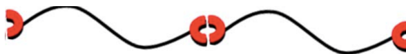
Figure 20 – Cartoon representing main-chain supramolecular polymers (red object represents a self-complementary supramolecular moiety, black line represents a classical covalent polymeric backbone).
