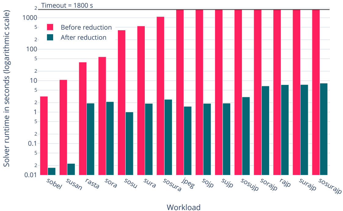
Figure 4.5: Solver run-time to produce a deadline-aware solution, as a function of different workloads using initial formulation and optimized formulation, 1 slot = 1 cycle.
