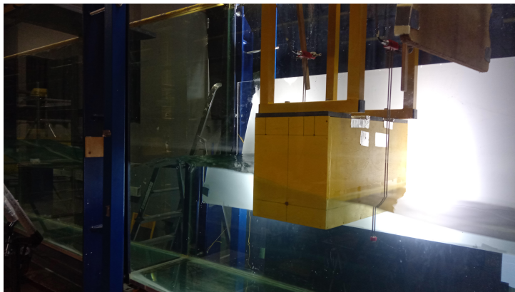
Figure 3.8: Photograph of the experimental setup of the rectangular barge in the wave flume close to the body.
