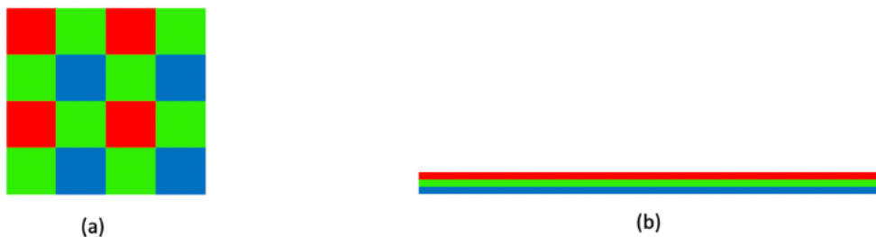
Figure 2.6: Digital camera vs scanner imaging sensor (a) camera sensor (b) scanner sensor
