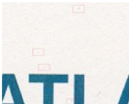
Figure 2.10: Dark spots in a scanned image due to dust/scratches over the scanner platen
