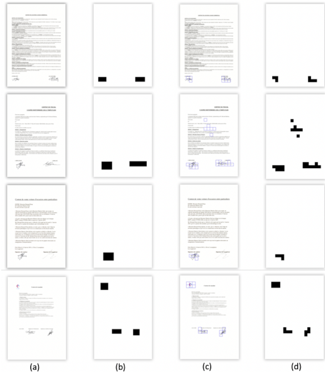
Figure 6.15: Examples of forged images and the outputs of the proposed CNN-based FD method (a) Forged images (b) Ground truths (c) Forged blocks marked by blue boxes (d) Estimated binary masks
