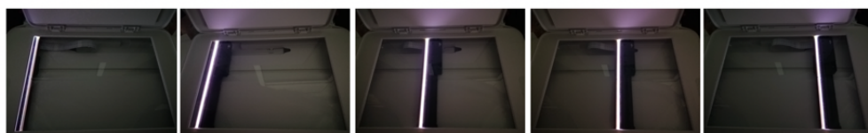
Figure 2.3: Changing positions of the scan head during the scanning process
