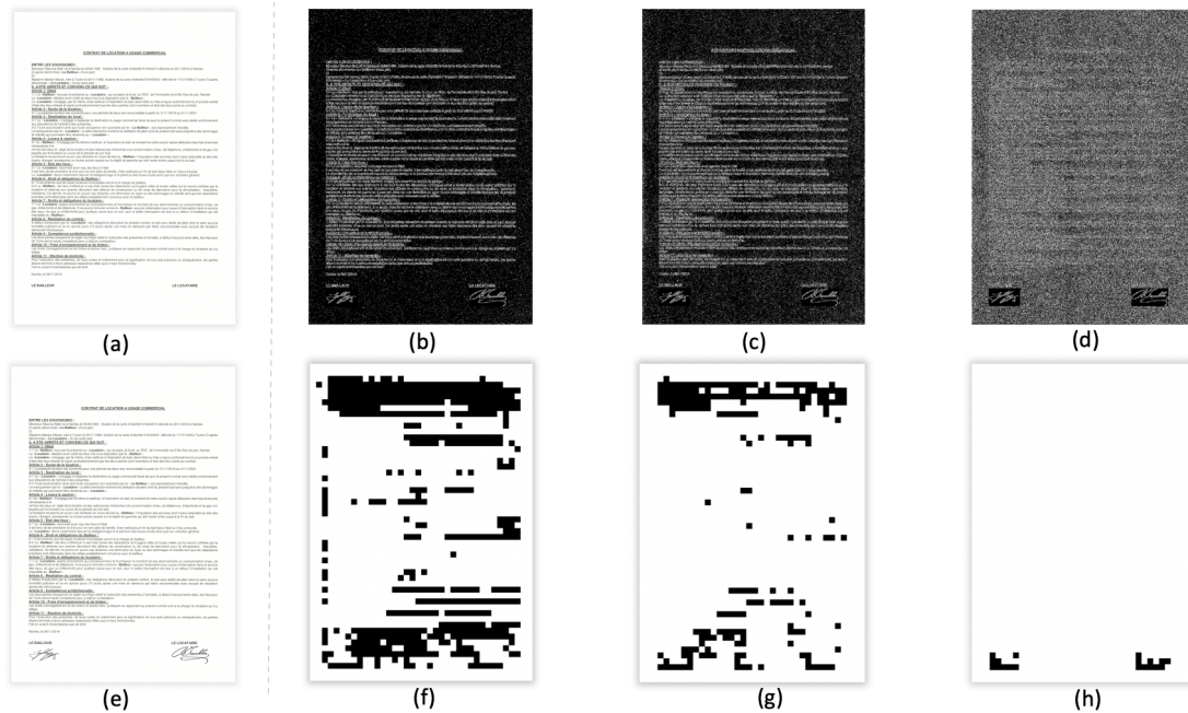
Figure 6.12: Sample HH subbands ((b), (c), (d)) of each color channel of an RGB image and their estimated forgery masks ((f), (g), (h)). From left to right are presented R, G and B, respectively. (a) is the original image and (e) is the tampered one
