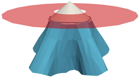
(a) Target shape (in blue) generated by dropping the flat torus (in red) on the cone.
