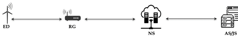
FIGURE 3.1: Basic LoRaWAN set up
