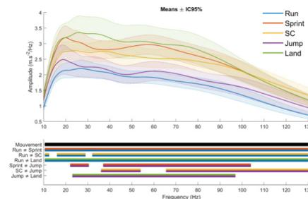
Figure 2: Heel impact amplitude in the frequency domain (means  $\pm$  95% CI) for each movement. Black line represents the ANOVA significant effect for the movements and colored lines are the significant differences between the different movements (post-hoc tests). SC: side-cuts
