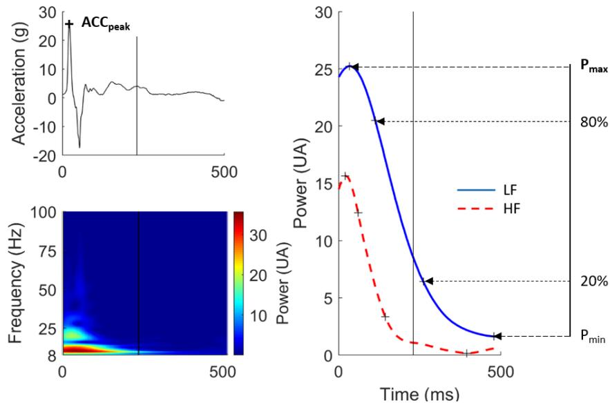
**Fig. 2. top left: acceleration signal of the *gastrocnemius medialis* at 15.5 km/h; bottom left: The map represents the power at each time and frequency obtained by the wavelet analysis; right: Low (LF, blue solid line) and high (HF, red dashed line) frequency components of the signal. The damping coefficient corresponds to the mean slope between 80% and 20%. The black vertical line represents the end of the stance phase.**
