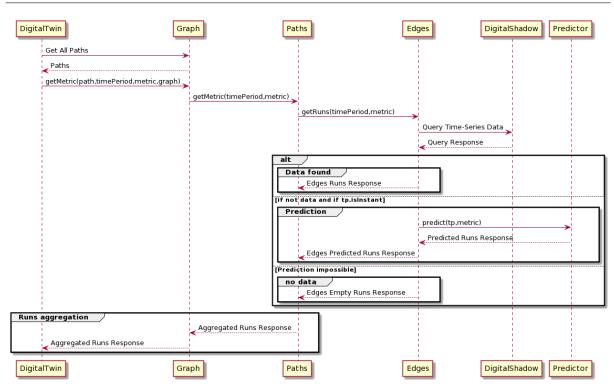
Figure 5.2 – Sequence diagram for getMetric
