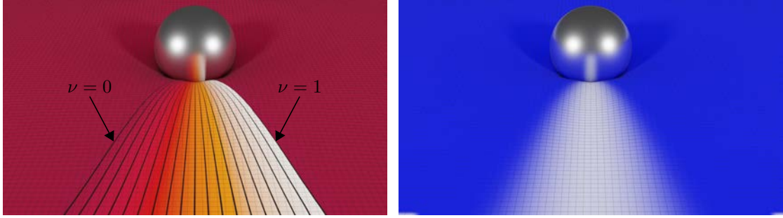
Figure 5.8.: Selected region parametrization of an elastic plane colliding with a rigid sphere. Left: the selected region \mathcal{Z} is equipped with a 1D parametrization \nu with Dirichlet constraint on \partial\mathcal{Z}_1 and \partial\mathcal{Z}_2 and Neumann conditions on \partial\mathcal{C} and \partial\mathcal{D} . Left: This parametrization allows us to define a fall-off on the user-controlled brush magnitude to produce smooth deformations.
