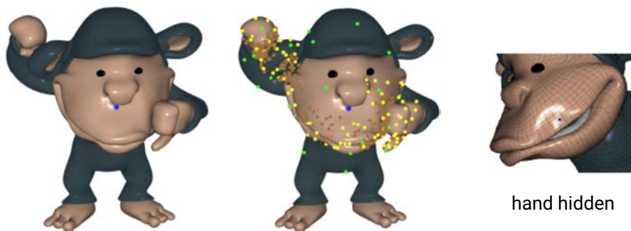
Figure 2.11.: Multi-resolution and collision free modeling of [LB19]. Multiple levels, corresponding to the different colored points, are activated around the multiple contact sites (lips, cheek and ear) on the chimpanzee to detect and resolve the collisions. User handles are shown in blue. Right: zoom-in on the resolved collision between the mouth and the hand. (Source: [LB19])
