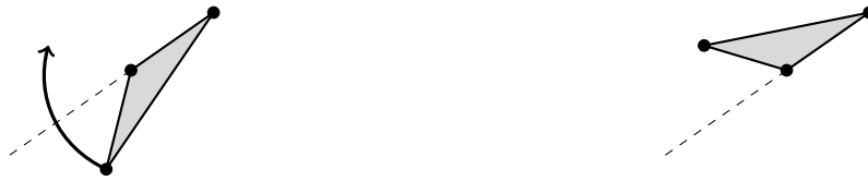
Figure 1.5: Example of how a mesh element in two dimensions can be reversed without any vertex superposing an edge. The cost function is generally not differentiable at the inversion location.
