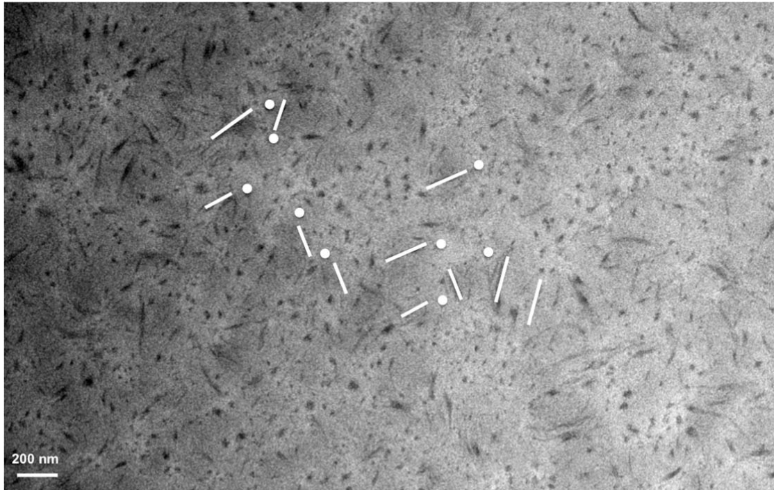
Figure S5/ TEM micrograph of a transparent collagen matrix (~45 mg/mL). Collagen fibrils are monodisperse in diameter (~25-30 nm). They appear aligned parallel or perpendicular to the section plane, as respectively underlined by lines and dots.
