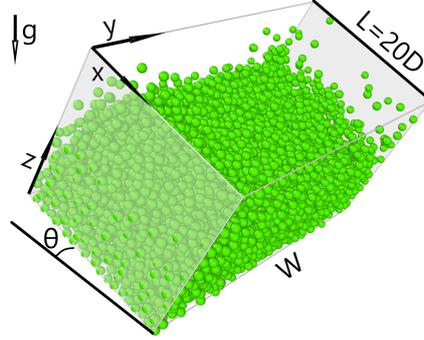
**Figure 3.1:** Figure for numerical simulation system on  $W = 40D$ . The system is driven by gravity  $\mathbf{g}$  with periodic condition ( $L = 20D$ ) along the flow direction  $\mathbf{x}$ ,  $\mathbf{y}$  is the transverse direction normal to the flat side-walls (width of the cell:  $W$ ) and  $\mathbf{z}$  is normal to the flat base. The angle  $\theta$  between  $\mathbf{g}$  and  $\mathbf{z}$  is the inclination angle.
