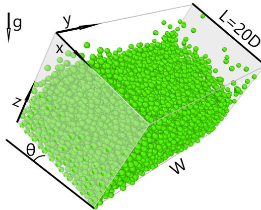
**Figure 1.2:** Scheme of the simulated system. The channel is inclined with an angle  $\theta$  with respect to the horizontal. Cartesian coordinate system with unit vectors  $x$  along the flow,  $y$  perpendicular to side-walls, and  $z$  normal to bottom.
