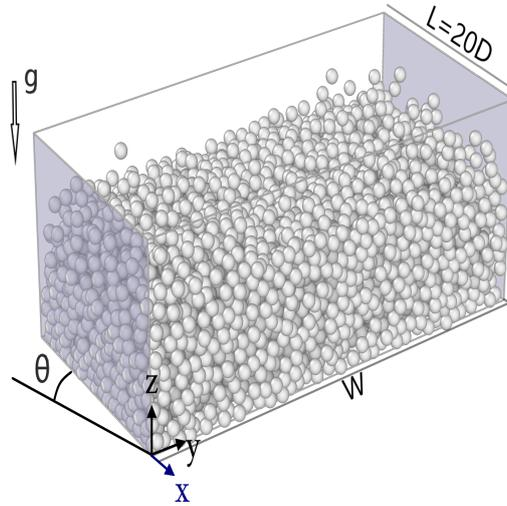
**Figure 2.2:** Figure for numerical simulation system (periodic cell). The flow is driven by gravity  $g$ , periodic conditions are applied in direction  $x$ . The flow direction corresponds thus to  $x$ ,  $y$  is the horizontal transverse direction perpendicular to the side walls and  $z$  is perpendicular to the base. The angle  $\theta$  between  $z$  and  $g$  is the inclination angle.
