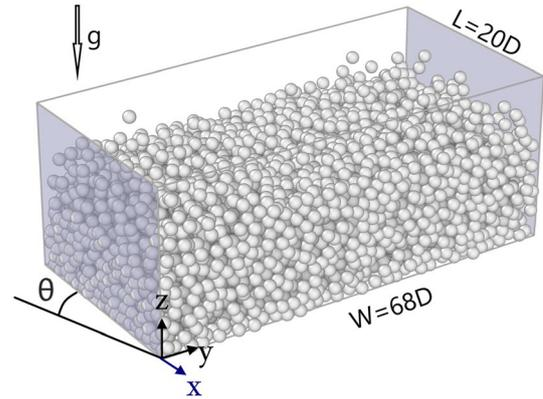
**Fig. 1** Scheme of the simulated system. The channel consists of frictional and flat bottom and sides and is inclined with an angle  $\theta$  with respect to the horizontal. The longitudinal length  $L$  and width  $W$  of the channel are set to  $20D$  and to  $68D$ , respectively. The channel is not bounded in the  $(0z)$  direction and we use periodic boundary conditions in the stream-wise direction
