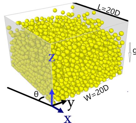
Figure 1: Configuration setup. The granular flow is confined by lateral walls with a width  $W = 20D$ . Periodic boundary conditions are used in the stream-wise direction with a length  $L$  and an angle of inclination  $\theta$ .
