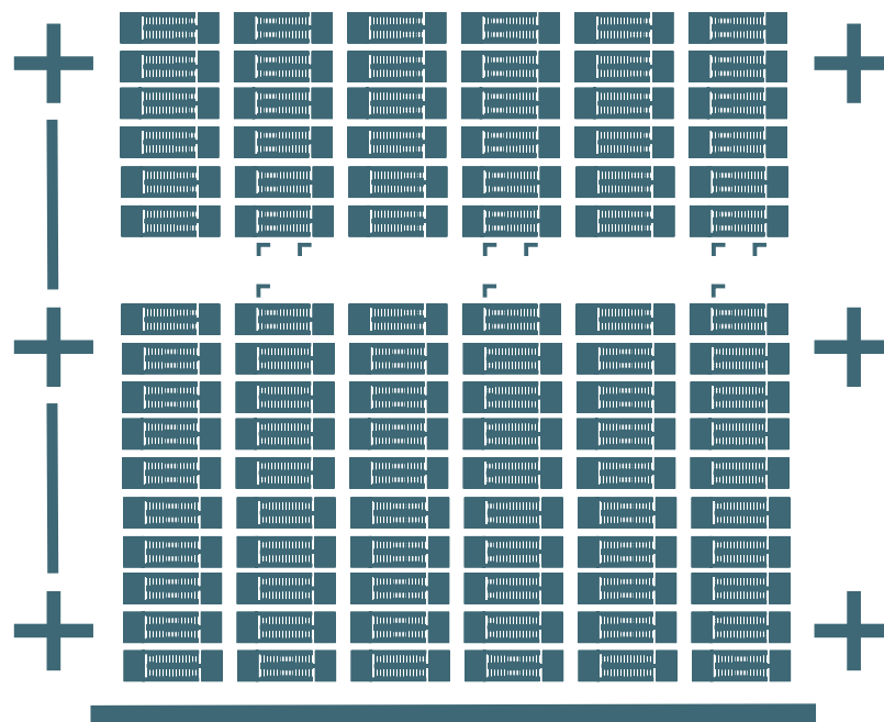
Fig. 4.13 Lithography mask design for e-actuated trumpets.
