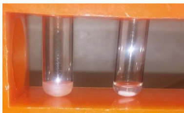
Figure 42. Re-lipidation of AcrB with a protein:lipid ratio of 3:1 (right sample) and 2:1 (left sample). White precipitate, likely to be precipitated lipid.
