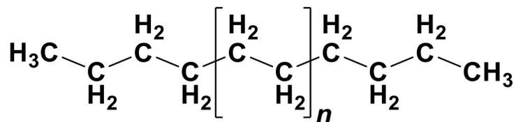
*Figure 3. Polyethylene molecular structure*
