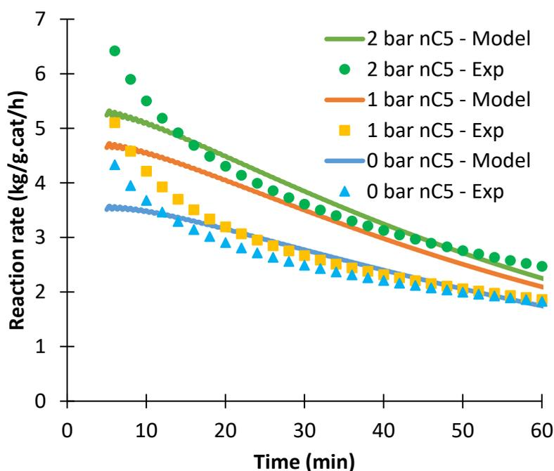
*Figure 111. Polymerization rate calculated with the PFM and the experimental data of 7 bar of ethylene, with different amounts of n-pentane, and without hydrogen, at 80°C*
