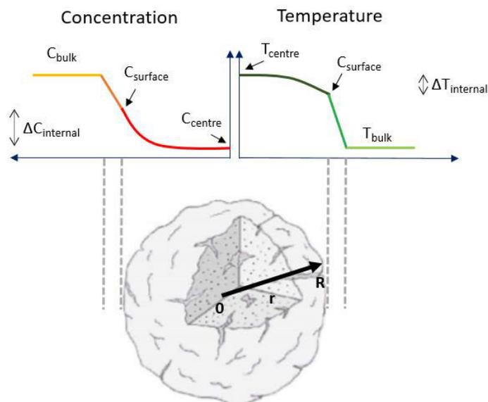
*Figure 7. Schematic representation of temperature and concentration gradient through the growing polymer particle. Adapted from <sup>47</sup>*
