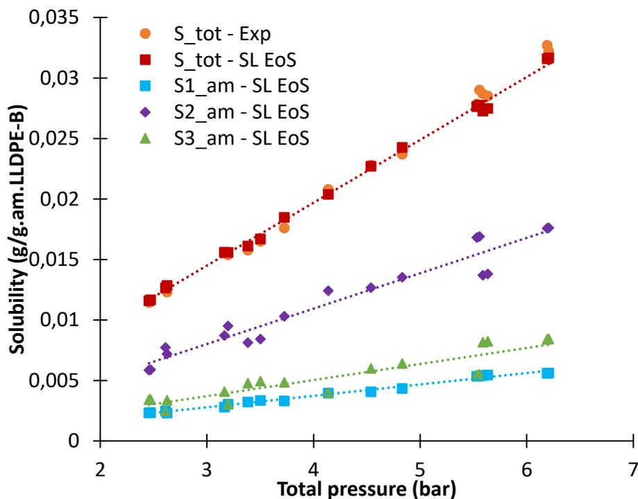
**Figure 69.** Experimental and SL modeling of overall and partial solubility of each component in ethylene/propane/1-butene/LLDPE-B at 70°C. Gas phase composition of the mixture is given in **Table 24**.  $k_{ij}$  are given in **Table 25**
