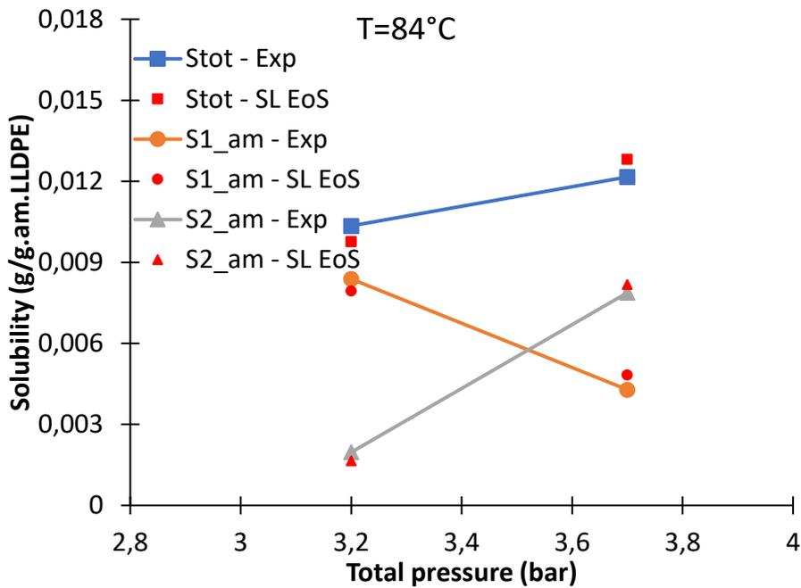
Figure 43. Total ( $S_{tot}$ ) and partial solubility of ethylene ( $S1_{am}$ ) and 1-butene ( $S2_{am}$ ) in ethylene/1-butene/LLDPE-I system at 84°C. The lines represent the experimental solubility and the red points represent the solubility calculated with SL EoS. Gas phase composition is  $x_{C2}=0.496$  and  $x_{1C4}=0.504$  at 84°C.  $k_{ij}$  correlations are given in Table 20
