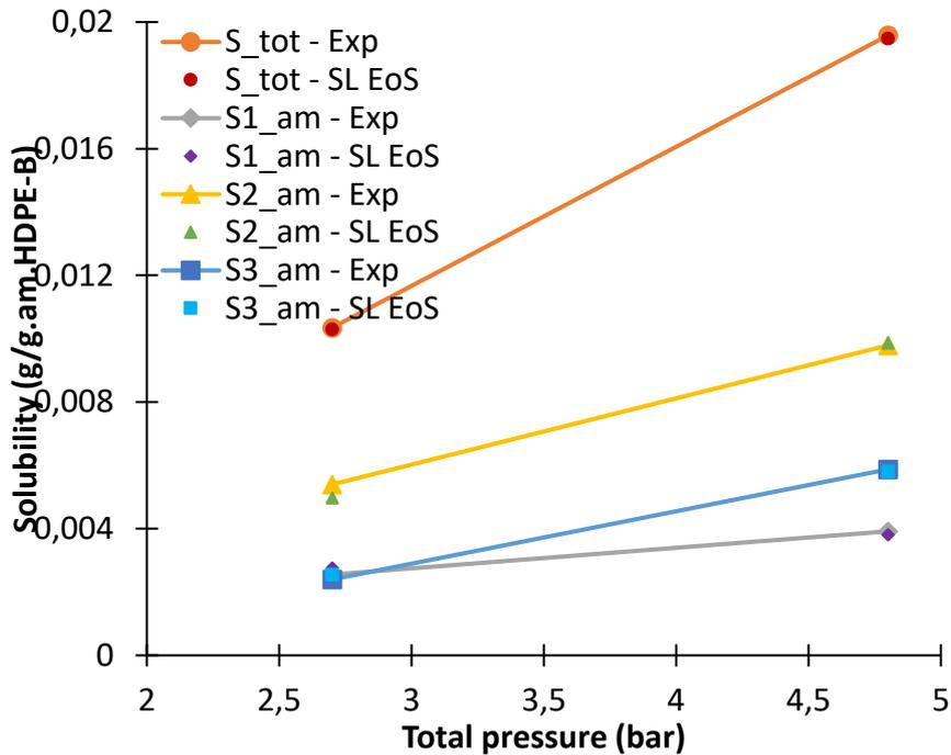
Figure 67. Experimental and SL modeling of overall and partial solubility of each component in ethylene/propane/1-butene/HDPE-B at 75°C. Gas phase composition of the mixture is given in Table 23.  $k_{ij}$  are given in Table 25
