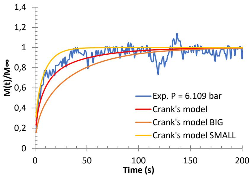
*Figure 83.* Sorption rates of ethylene/LLDPE-B binary system for a total pressure of 6.109 bar at 70°C obtained through gravimetric method and Crank's diffusion equation for particles with two sizes of granules
