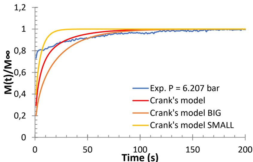
**Figure 97.** Sorption rates of ethylene/propane/1-butene/LLDPE-B quaternary system at total pressure of 6.207 bars and 70°C obtained through gravimetric method and Crank's diffusion equation for **Composition 1**. Molar composition is:  $x_{C3}=0.39$ ,  $x_{1C4}=0.23$  and  $x_{C2}=0.38$ .
