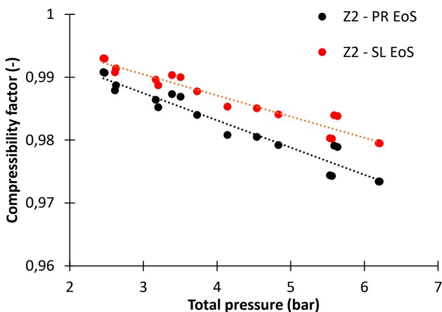
**Figure 71.** Compressibility factor of propane in  $C_2/C_3/1C_4/LLDPE-B$  quaternary system at  $70^\circ C$ . The red points represent the compressibility values calculated with Peng-Robinson ( $Z_1 - PR$  EoS) and the black points represent the predictions of the compressibility factor from the ternary SL EoS ( $Z_1 - SL$  EoS). The dashed lines are simply trend lines to guide the eye.
