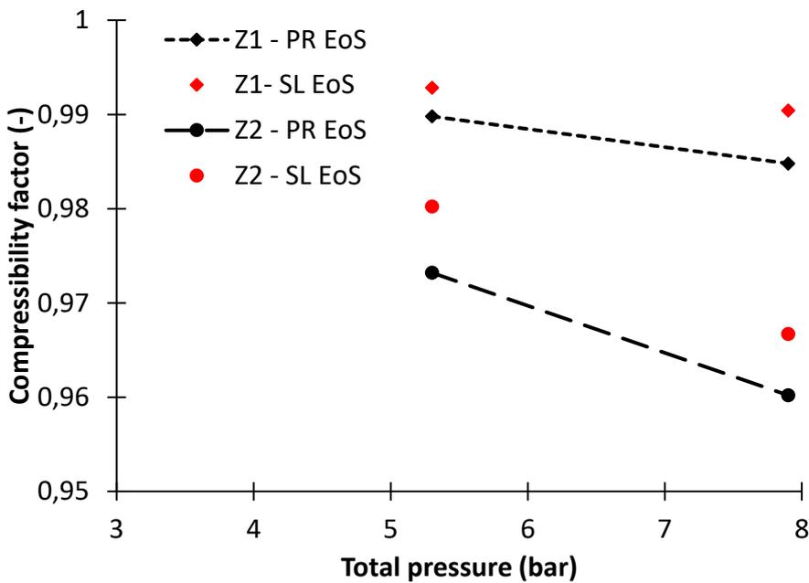
Figure 46. Compressibility factor of ethylene ( $Z_1$ ) and propane ( $Z_2$ ) in ethylene/propane/LLDPE-I system at 80°C. The lines represent compressibility values calculated with Peng-Robinson and points represent the predictions of the compressibility factor from the ternary SL EoS.
