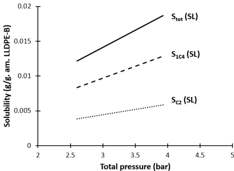
**Figure 26.** Total solubility  $S_{tot}$  (SL), partial solubility of ethylene  $S_{C2}$  (SL) and partial solubility of 1-butene  $S_{1C4}$  (SL) in LLDPE-B at 70°C from SL EoS (ternary system  $C_2/1C_4/LLDPE-B$ ).  $k_{ij}$  are defined in **Table 15**
