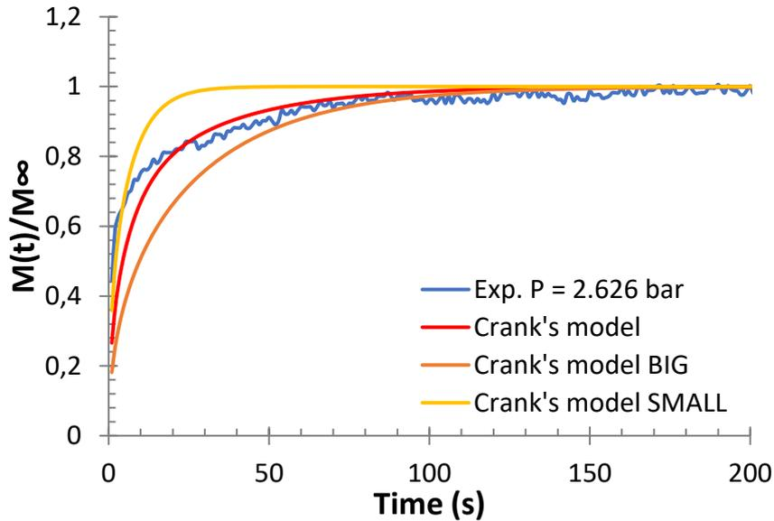
*Figure 95.* Sorption rates of ethylene/propane/1-butene/LLDPE-B quaternary system at total pressure of 2.626 bars and 70°C obtained through gravimetric method and Crank's diffusion equation for particles with two sizes of granules for **Composition 1**. Molar composition is:  $x_{C3}=0.39$ ,  $x_{1C4}=0.23$  and  $x_{C2}=0.38$ .
