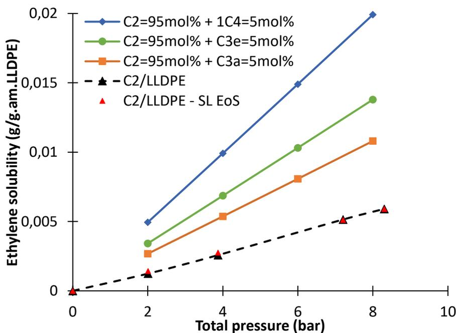
**Figure 52.** Binary solubility of ethylene in LLDPE taken from<sup>21</sup> (dotted lines) and from SL EoS (points) and the partial ternary solubility of ethylene in presence of 5 mol% of propane, propylene and 1-butene in LLDPE-I at 80°C.  $k_{ij}$  for the studied ternary systems at the temperature of interest are defined in **Table 20** and for the ethylene/LLDPE binary system in **Table 22**.
