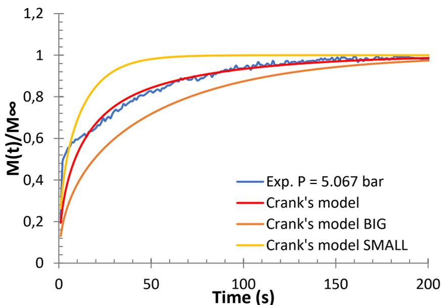
**Figure 87.** Sorption rates of ethylene/isobutane/LLDPE-B ternary system at total pressure of 5.067 bars and 70°C obtained through gravimetric method and Crank's diffusion equation for particles with two sizes of granules. Molar composition is:  $x_{C2} = 0.485$  and  $x_{iC4} = 0.515$ .
