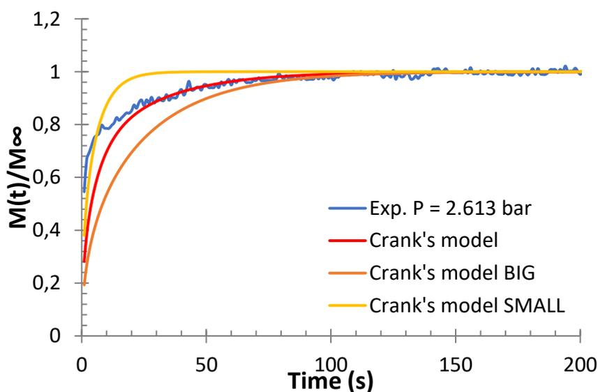
**Figure 98.** Sorption rates of ethylene/propane/1-butene/LLDPE-B quaternary system at total pressure of 2.613 bars and 70°C obtained through gravimetric method and Crank's diffusion equation for particles with two sizes of granules for **Composition 2**. Molar composition is:  $x_{C3}=0.42$ ,  $x_{1C4}=0.17$  and  $x_{C2}=0.41$
