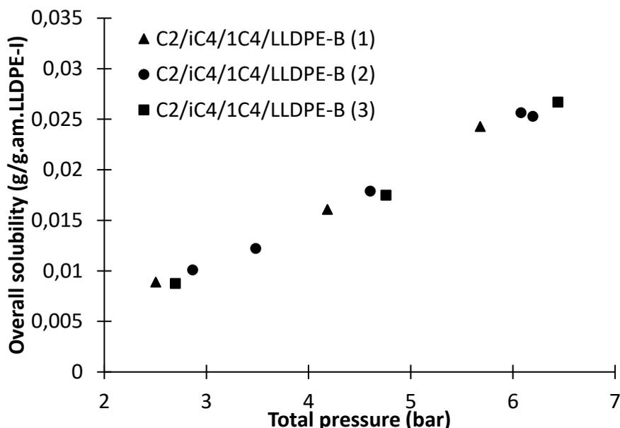
**Figure 62.** Overall solubility of quaternary system of ethylene/isobutane/1-butene/LLDPE-B at 70°C with different composition of the gas-phase. Gas-phase composition for each experiment is  $x_{iC_4}=0.43$  and  $x_{1C_4}=0.17$  for (1),  $x_{iC_4}=0.4$  and  $x_{1C_4}=0.23$  for (2) and  $x_{iC_4}=0.44$  and  $x_{1C_4}=0.21$  for (3)
