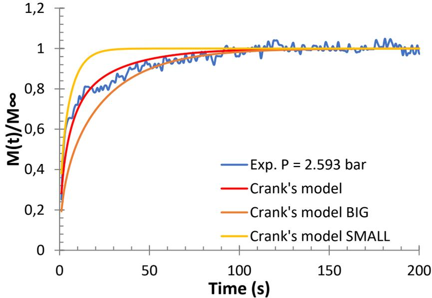
**Figure 91.** Sorption rates of ethylene/propane/LLDPE-B ternary system at total pressure of 2.593 bars and 70°C obtained through gravimetric method and Crank's diffusion equation for particles with two sizes of granules. Molar composition is:  $x_{C_2} = 0.509$  and  $x_{iC_4} = 0.491$ .
