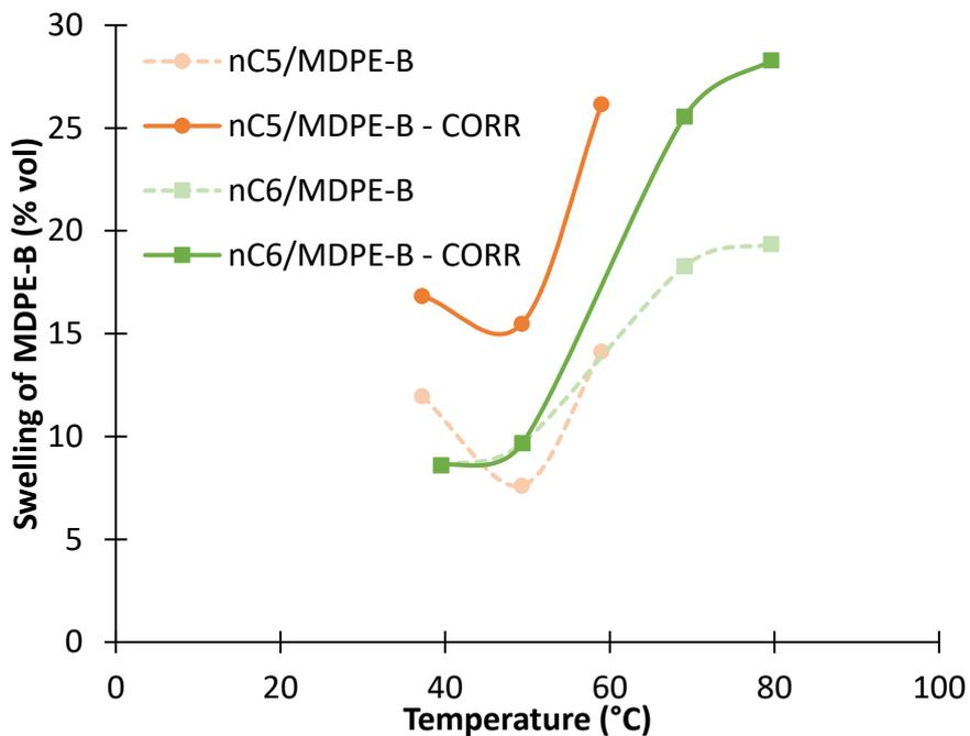
Figure 149. Swelling measured experimentally and corrected with MDPE-B dissolution in the solvent given in Table 42
