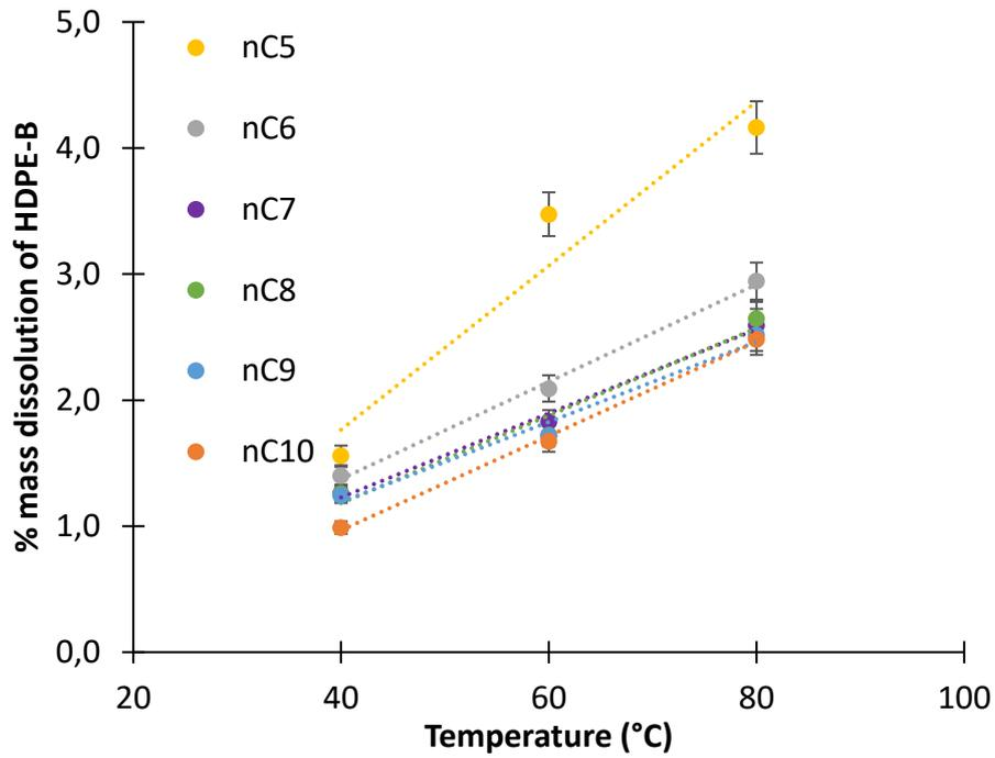
Figure 130. Percent mass dissolved of HDPE-B powders in the presence of different solvents and at different temperatures.
