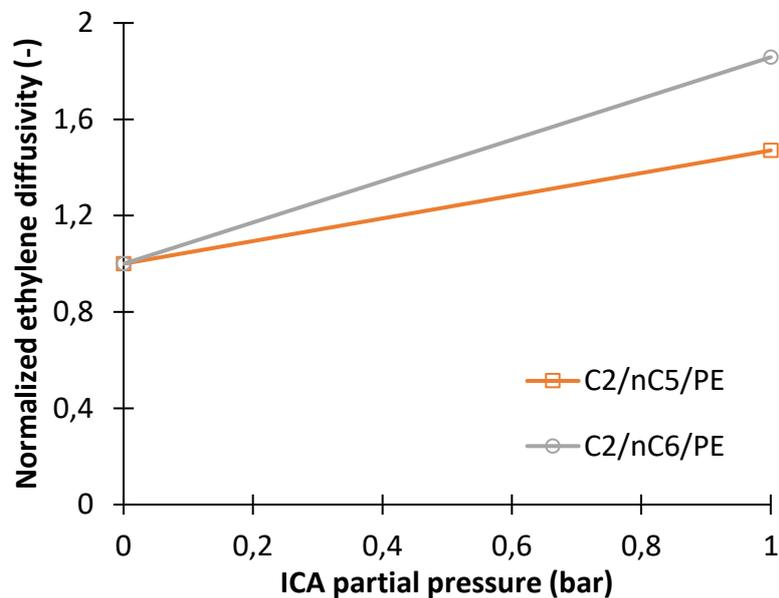
*Figure 123.* Ethylene diffusivity in the ternary system of ethylene/ICA/PE normalized by ethylene diffusivity in the binary system of ethylene/PE as a function of ICA partial pressure at 80°C.
