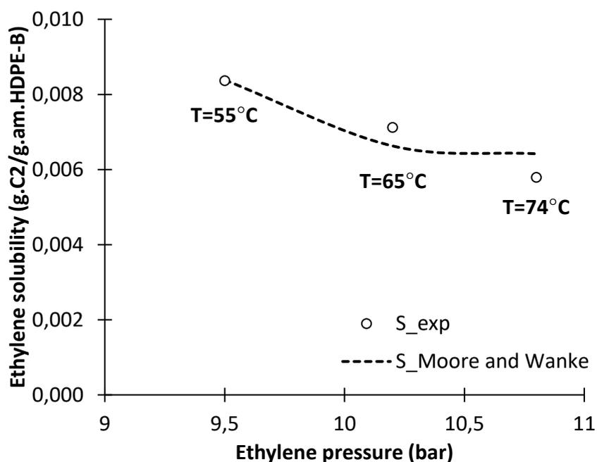
**Figure 35.** Ethylene solubility in the amorphous phase of HDPE-B at different temperatures and ethylene pressures. The lines represent the solubility from Moore and Wanke<sup>6</sup> and the points represent the experimental solubility measured with the pressure decay method.
