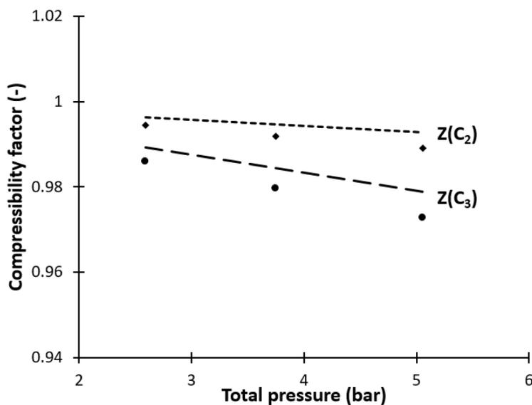
**Figure 21.** Compressibility factor of ethylene ( $C_2$ ) and propane ( $C_3$ ) in  $C_2/C_3/LLDPE-B$  mixture. Points represent compressibility values calculated with Peng-Robinson and the lines represent the predictions of the compressibility factor from the ternary SL EoS
