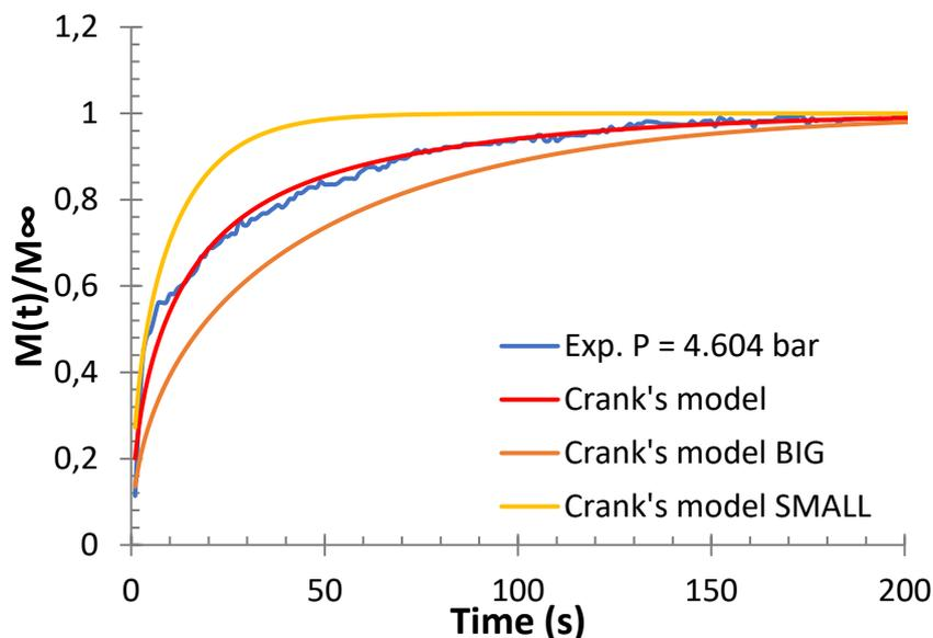
*Figure 103.* Sorption rates of ethylene/isobutane/1-butene/LLDPE-B quaternary system at total pressure of 4.604 bars and 70°C obtained through gravimetric method and Crank's diffusion equation for particles with two sizes of granules equation for **Composition 3**. Molar composition is:  $x_{iC4}=0.37$ ,  $x_{1C4}=0.23$  and  $x_{C2}=0.40$ .
