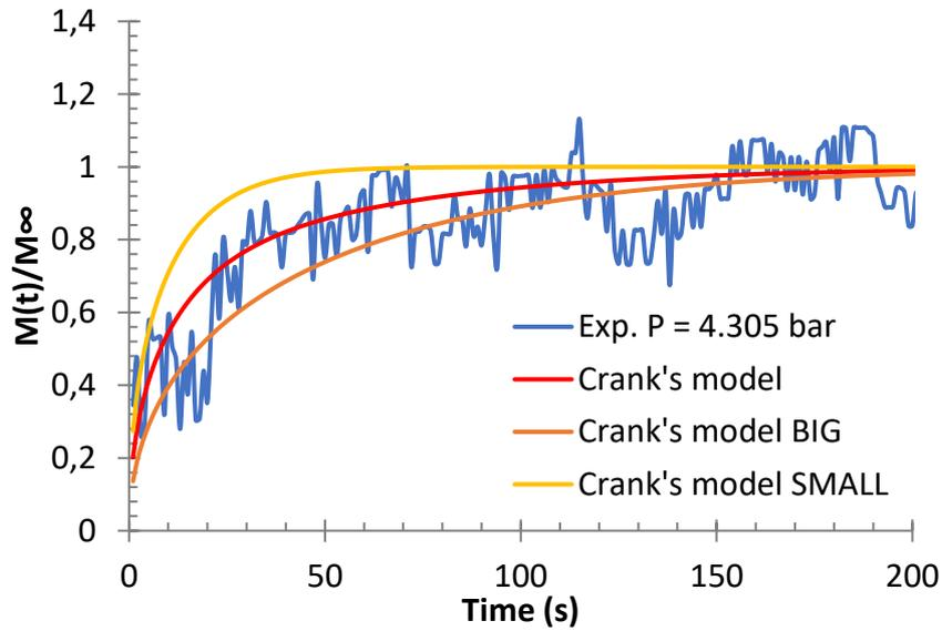
*Figure 82.* Sorption rates of ethylene/LLDPE-B binary system at a total pressure of 4.305 bar at 70°C obtained through gravimetric method and Crank's diffusion equation for particles with two sizes of granules
