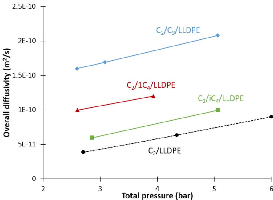
**Figure 94.** Overall diffusivity of ethylene in LLDPE-B in binary system and in presence of propane, isobutane and 1-butene at 70°C with the molar fractions:  $x_{1C_4} = 0.383$ ,  $x_{iC_4} = 0.515$  and  $x_{C_3} = 0.491$ .
