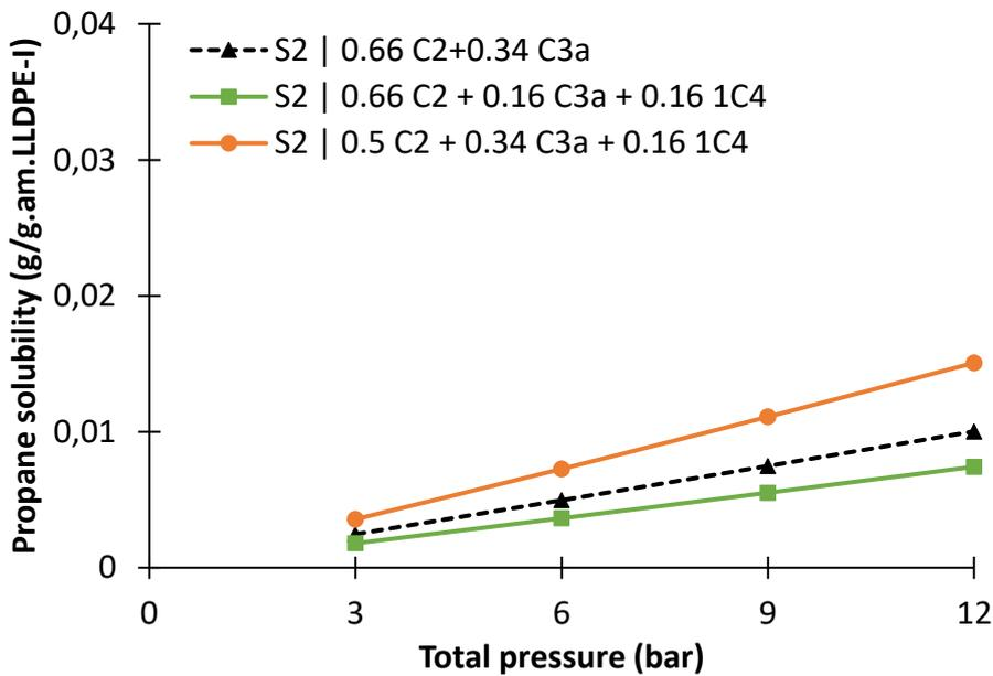
Figure 80. Propane partial solubility calculated from SL EoS for ethylene/propane /LLDPE-I ternary system and for ethylene/propane/1-butene/LLDPE-I quaternary system at 80°C.  $k_{ij}$  for the ternary system was taken from Table 20 and for the quaternary system from Table 25
