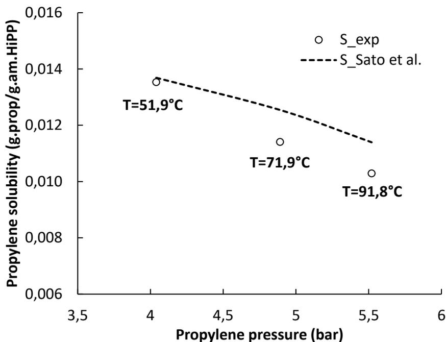
**Figure 34.** Propylene solubility in the amorphous phase of HiPP at different temperatures and propylene pressures. The lines represent the solubility from Sato et al.<sup>12</sup> and the points represent the experimental solubility measured with the pressure decay method.
