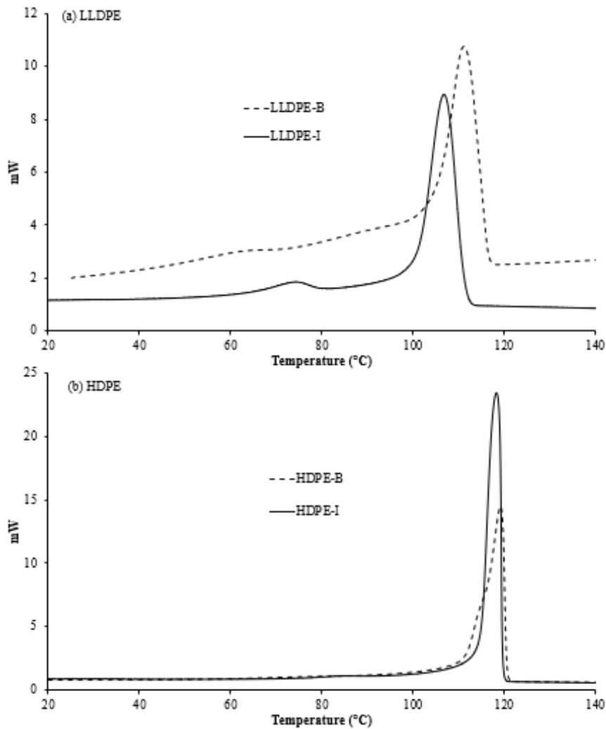
Figure 30. DSC thermograms of the 4 PE shown in Table 17. (a) LLDPE and (b) HDPE.
