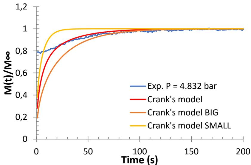
*Figure 96.* Sorption rates of ethylene/propane/1-butene/LLDPE-B quaternary system at total pressure of 4.832 bars and 70°C obtained through gravimetric method and Crank's diffusion equation for particles with two sizes of granules for **Composition 1**. Molar composition is:  $x_{C3}=0.39$ ,  $x_{1C4}=0.23$  and  $x_{C2}=0.38$ .
