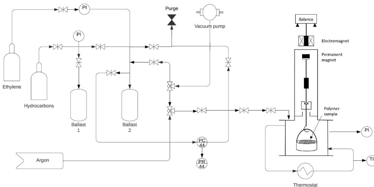
**Figure 10.** P&ID of the sorption reactor based on gravimetric method
