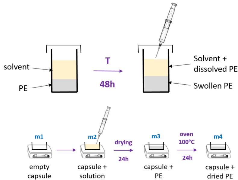
*Figure 125. Experimental scheme of the dissolution of polyethylene powders in liquid diluents at different temperatures*
