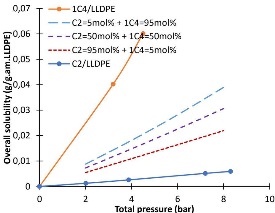
**Figure 51.** Solubility of binary ethylene/LLDPE (C2) and 1-butene/LLDPE (1C4) systems and overall solubility of their mixture in ternary system of ethylene/1-butene/LLDPE at 80°C, calculated with SL EoS. Different composition of the gaseous mixture in the ternary system is shown.  $k_{ij}$  for binary systems are defined in Table 22 and for ternary systems in Table 20
