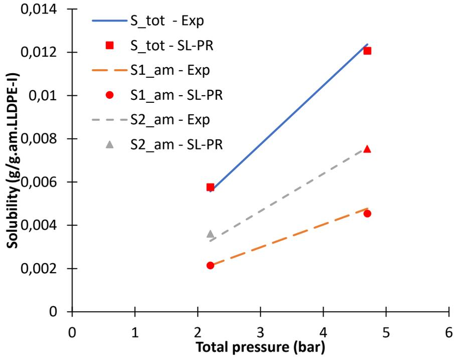
Figure 47. Overall and partial solubility of ethylene/propylene/LLDPE-I ternary system at 68°C. The estimation of the partial solubility is achieved by using the SL-PR method. Molar composition of the system is given in Table 19 and  $k_{ij}$  used for this study is given in Table 20
