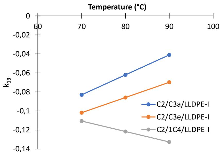
**Figure 44.** Temperature dependent correlation of  $k_{13}$  for the different studied systems of ethylene/propane/LLDPE-I (C<sub>2</sub>/C<sub>3a</sub>/LLDPE-I), ethylene/propylene/LLDPE-I (C<sub>2</sub>/C<sub>3e</sub>/LLDPE-I) and ethylene/1-butene/LLDPE-I (C<sub>2</sub>/1C<sub>4</sub>/LLDPE-I).
