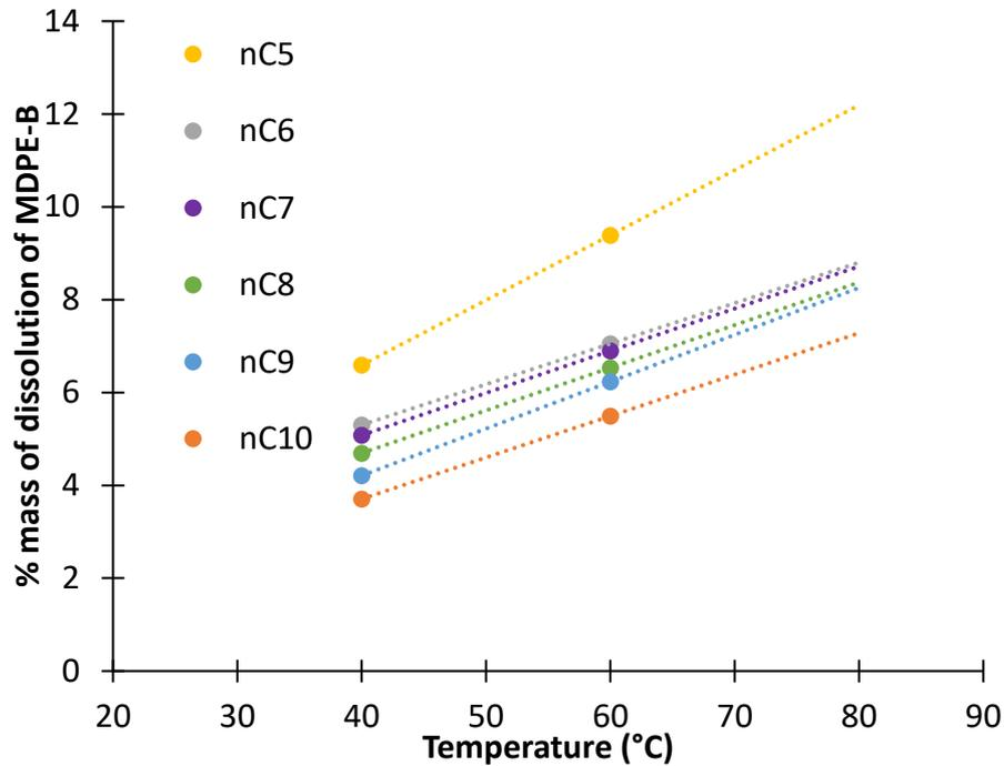
Figure 132. Percent mass dissolved of MDPE-B powders in the presence of different solvents and at different temperatures.
