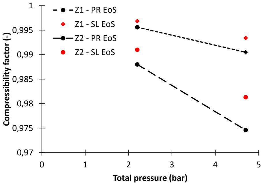
Figure 48. Compressibility factor of ethylene ( $Z_1$ ) and propylene ( $Z_2$ ) in ethylene/propylene/LLDPE-I system at 68°C. The lines represent compressibility values calculated with Peng-Robinson and points represent the predictions of the compressibility factor from the ternary SL EoS.
