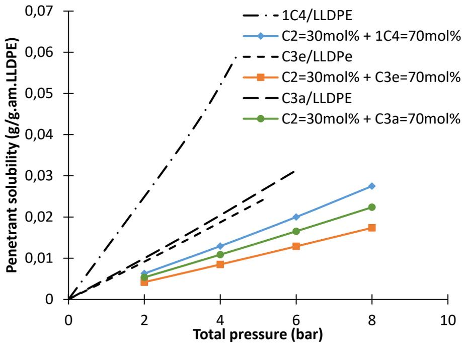
Figure 55. Binary solubility of 1-butene (1C4), propylene (C3e) and propane (C3a) and the partial ternary solubility of these penetrants with 30 mol% of ethylene in LLDPE at 80°C, calculated with SL EoS.  $k_{ij}$  for the studied ternary systems at the temperature of interest are defined in Table 20 and for the ethylene/LLDPE binary system in Table 22.
