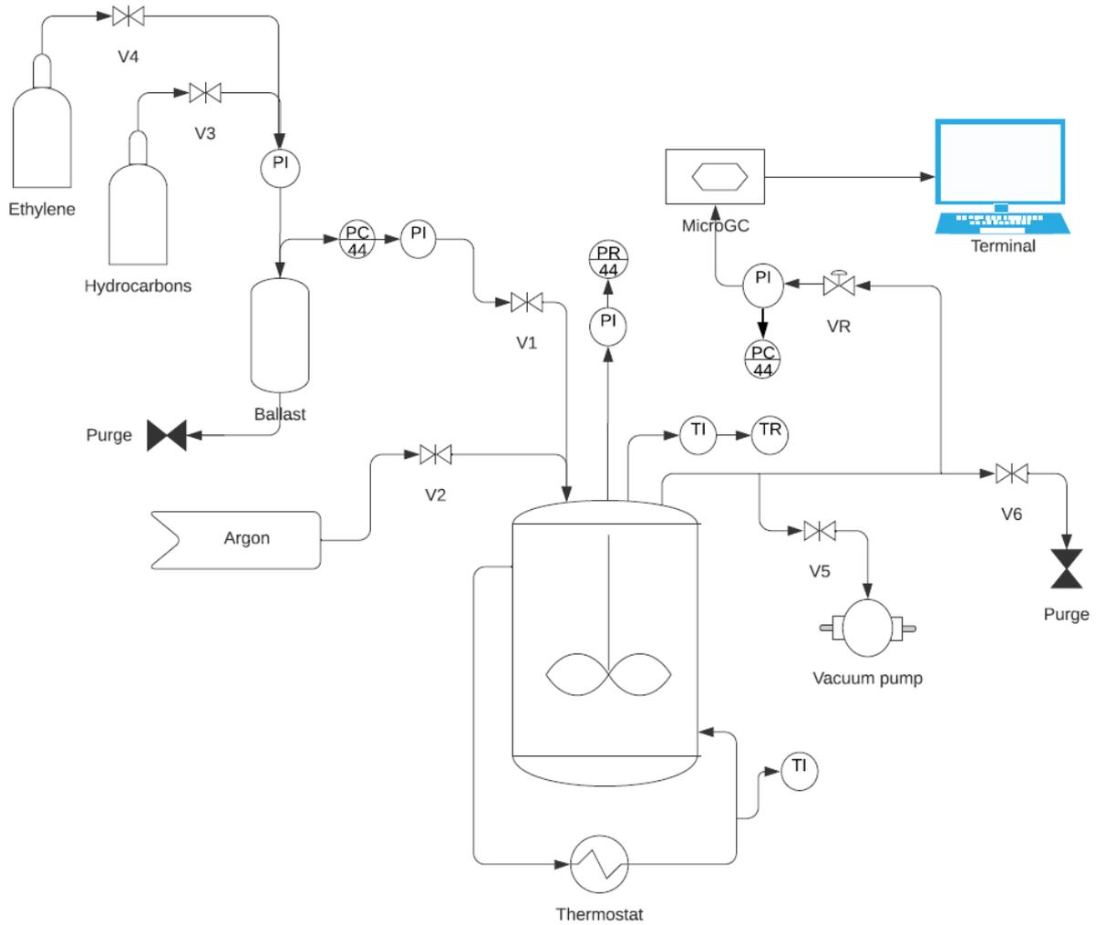
Figure 32. P&ID of the sorption reactor based on pressure decay method
