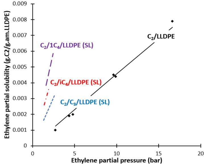
**Figure 28.** Partial ternary solubility of ethylene from SL EoS in presence of  $C_3$ ,  $iC_4$  and  $1C_4$  with the molar fractions:  $x_{1C_4}=0.383$ ,  $x_{iC_4}=0.515$ ,  $x_{C_3}=0.491$ ;  $k_{ij}$  for ternary systems are defined in **Table 15**. Comparison to binary solubility of  $C_2$ /LLDPE, where points represent the experimental solubility and the line represents the solubility fitted to SL EoS, with  $k_{ij}$  defined in **Table 8**
