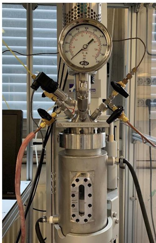
*Figure 128. Experimental set-up for the swelling experiments in slurry*
