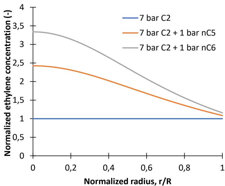
**Figure 124.** Ethylene concentration gradient as a function of the normalized particle radius at 40 minutes of the reaction for 7 bar of ethylene with 1 bar of n-pentane and n-hexane normalized by ethylene concentration gradient without ICA at 80°C
