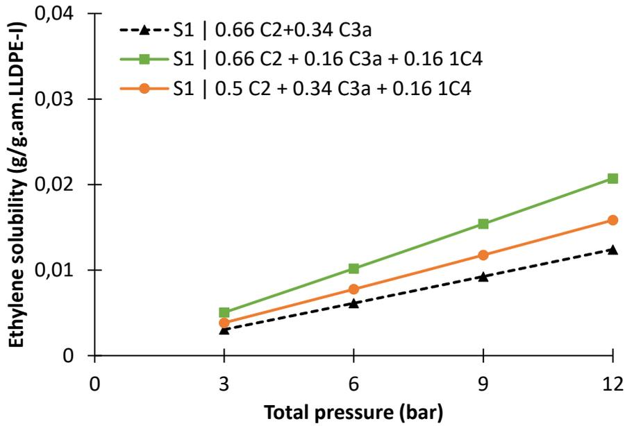
Figure 79. Ethylene partial solubility calculated from SL EoS for ethylene/propane /LLDPE-I ternary system and for ethylene/propane/1-butene/LLDPE-I quaternary system at 80°C.  $k_{ij}$  for the ternary system was taken from Table 20 and for the quaternary system from Table 25
