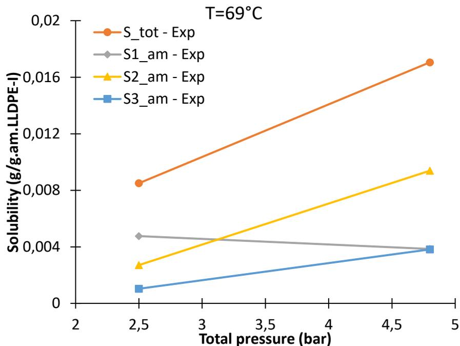
**Figure 57.** Total and partial solubility of ethylene/propane/1-butene/LLDPE-I system at 69°C.  $S_{tot}$ ,  $S_{1_{am}}$ ,  $S_{2_{am}}$  and  $S_{3_{am}}$  are the total solubility of the mixture and the overall solubility of ethylene, propane and 1-butene in the amorphous phase of the polymer, respectively. Gas phase composition of the mixture is given in **Table 23**
