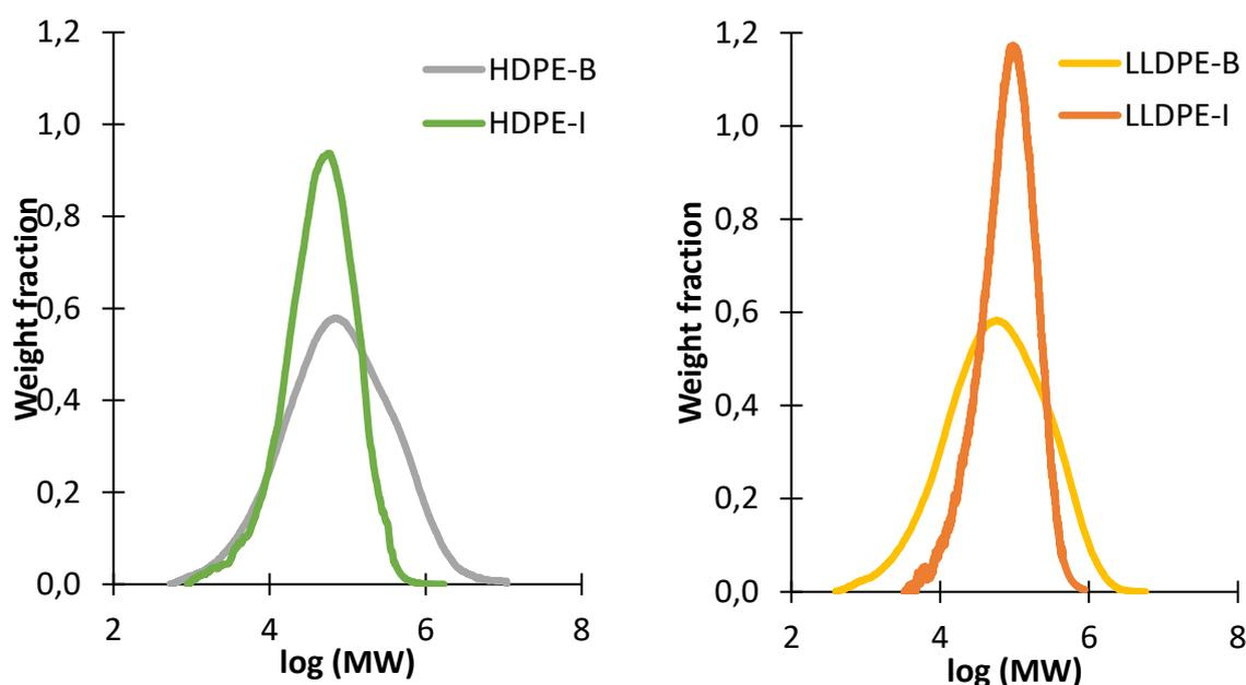
*Figure 74. Molecular weight distribution of the different used PE samples performed with the HT-GPC*
