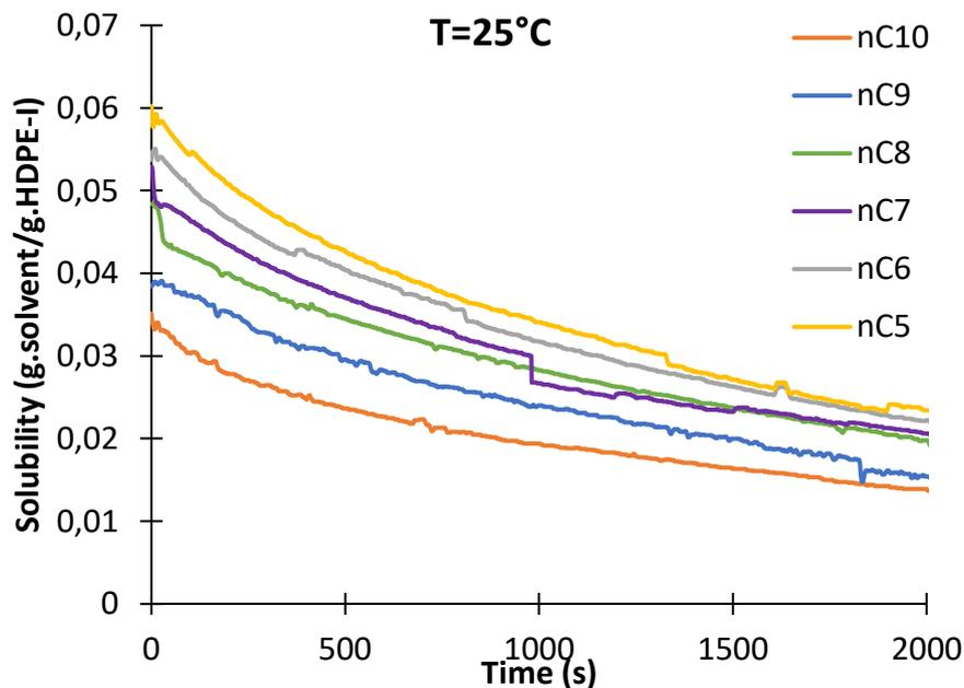
*Figure 141. Solubility of different solvents (nC<sub>5</sub>, nC<sub>6</sub>, nC<sub>7</sub>, nC<sub>8</sub>, nC<sub>9</sub>, nC<sub>10</sub>) in HDPE-I granules at 25°C (Each experiment was repeated at least two times under the same conditions)*
