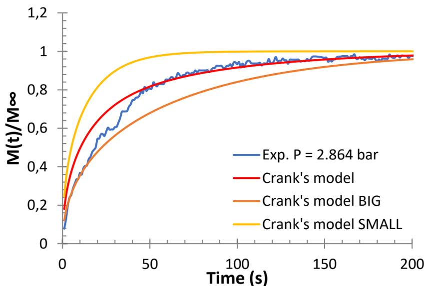
*Figure 102.* Sorption rates of ethylene/isobutane/1-butene/LLDPE-B quaternary system at total pressure of 2.864 bars and 70°C obtained through gravimetric method and Crank's diffusion equation for particles with two sizes of granules for **Composition 3**. Molar composition is:  $x_{iC4}=0.37$ ,  $x_{1C4}=0.23$  and  $x_{C2}=0.40$ .
