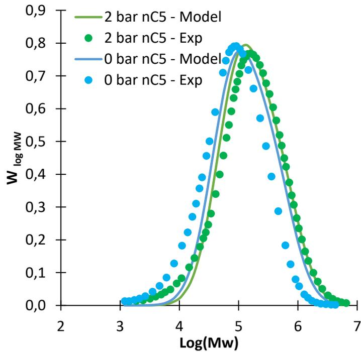
Figure 113. Molecular weight distribution calculated with the PFM and the experimental data measured with high temperature GPC of 7 bar of ethylene, 3 bar of hydrogen and 0 and 2 bar of n-pentane at 80°C
