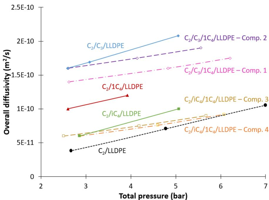
**Figure 109.** Overall diffusivities of all studied systems (i.e. binary, ternary and quaternary) at 70°C and different total pressures. Gas phase composition are given in Tables 3 and 4.
