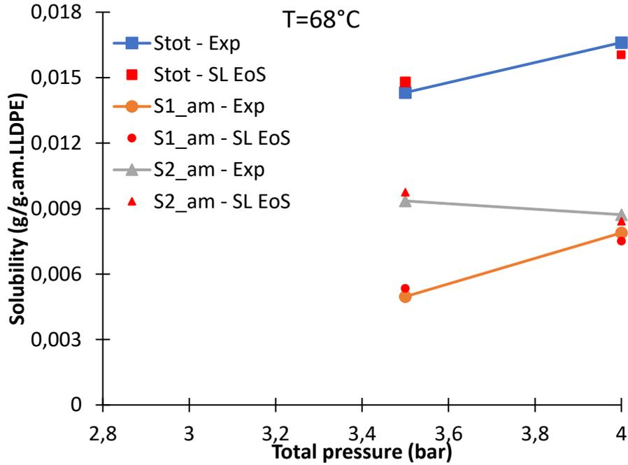
Figure 42. Total ( $S_{tot}$ ) and partial solubility of ethylene ( $S1_{am}$ ) and 1-butene ( $S2_{am}$ ) in ethylene/1-butene/LLDPE-I system at 68°C. The lines represent the experimental solubility and the red points represent the solubility calculated with SL EoS. Gas phase composition is  $x_{C2}=0.834$  and  $x_{1C4}=0.166$  at 68°C.  $k_{ij}$  correlations are given in Table 20
