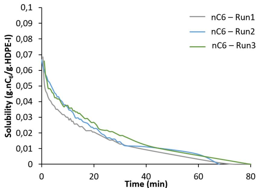
*Figure 133. Solubility of n-hexane in HDPE-I granules at room temperature (the same experiment at the same conditions was repeated three times)*
