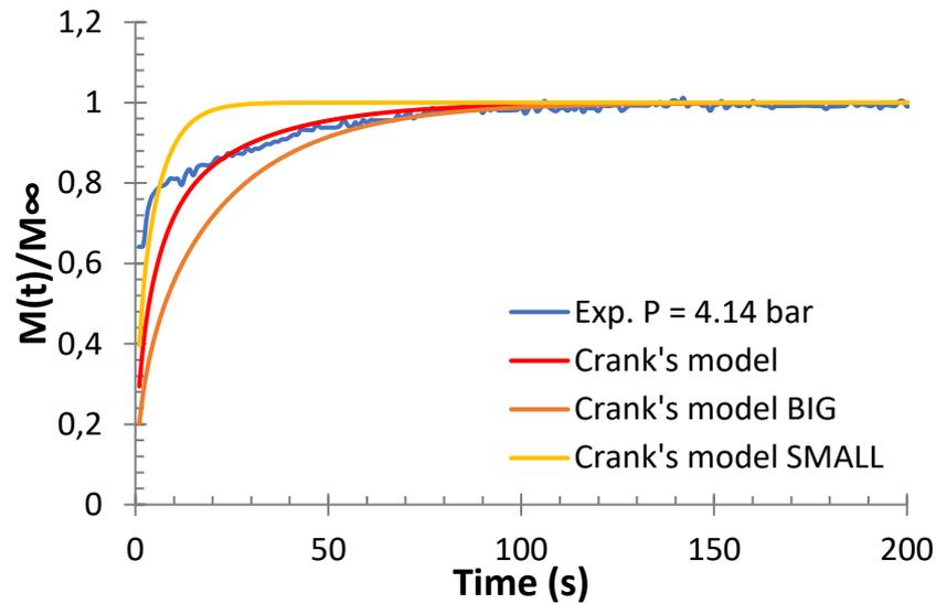
**Figure 99.** Sorption rates of ethylene/propane/1-butene/LLDPE-B quaternary system at total pressure of 4.14 bars and 70°C obtained through gravimetric method and Crank's diffusion equation for particles with two sizes of granules for **Composition 2**. Molar composition is:  $x_{C3}=0.42$ ,  $x_{1C4}=0.17$  and  $x_{C2}=0.41$
