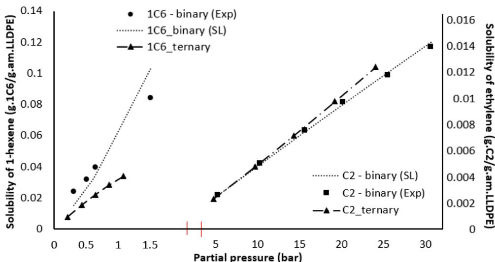
**Figure 19.** Ethylene and 1-hexene partial solubility in ternary system at 90°C with 5 mol% 1-hexene and 95 mol% ethylene and their corresponding partial pressures for each pure component for binary simulations.  $k_{ij}$  for ternary system were taken from **Table 12** and  $k_{ij}$  for binary systems were taken from **Table 5**.
