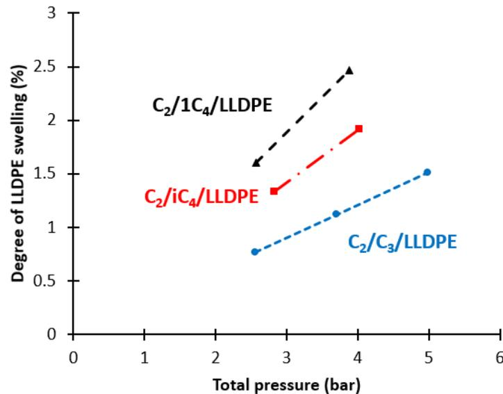
**Figure 27.** Degree of LLDPE swelling caused by the sorption of different penetrants; propane (C<sub>3</sub>), isobutane (iC<sub>4</sub>) and 1-butene (1C<sub>4</sub>) at 70°C. Gas phase composition is given in **Table 14** and  $k_{ij}$  are defined in **Table 15**
