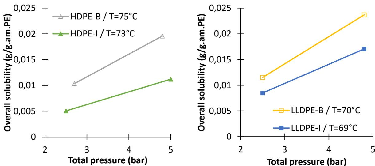
**Figure 73.** Overall solubility of ethylene/propane/1-butene in HDPE on the left and LLDPE on the right at different temperatures, using gravimetry for HDPE-B, HDPE-I and LLDPE-I and pressure decay method for LLDPE-B. Gas phase composition is shown in **Table 23** and **Table 24**. PE characteristics are shown in **Table 1**
