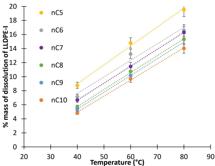
**Figure 131.** Percent mass dissolved of LLDPE-I powders in the presence of different solvents and at different temperatures.
