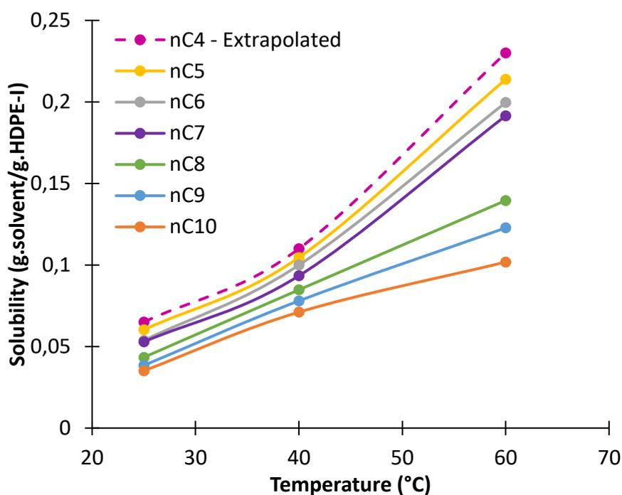
*Figure 144.* Solubility of different solvents (nC<sub>5</sub>, nC<sub>6</sub>, nC<sub>7</sub>, nC<sub>8</sub>, nC<sub>9</sub>, nC<sub>10</sub>) in HDPE-I granules as a function of temperature
