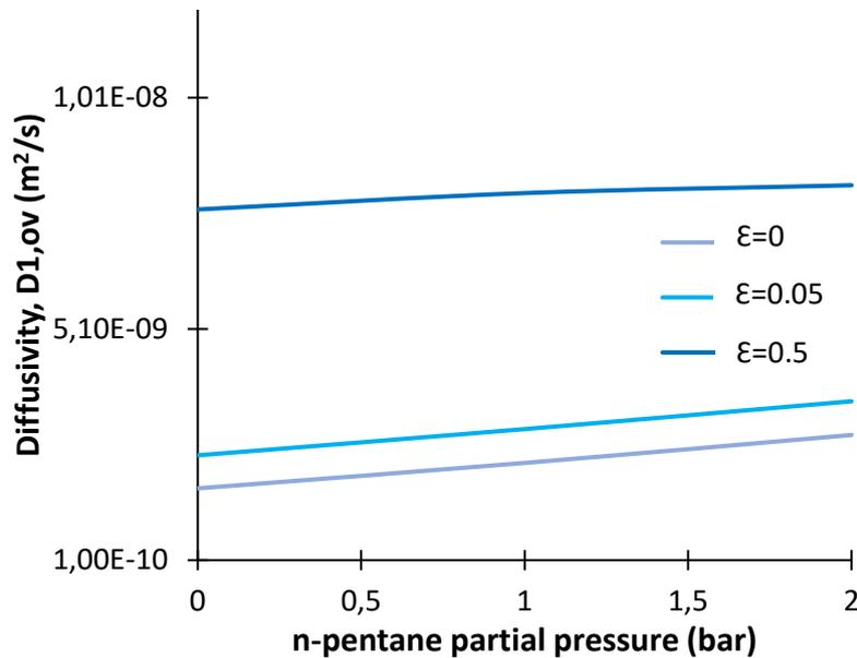
*Figure 115.* Ethylene diffusion coefficient in ethylene/n-pentane/LLDPE at 80°C as a function of n-pentane partial pressure for different polymer porosity.
