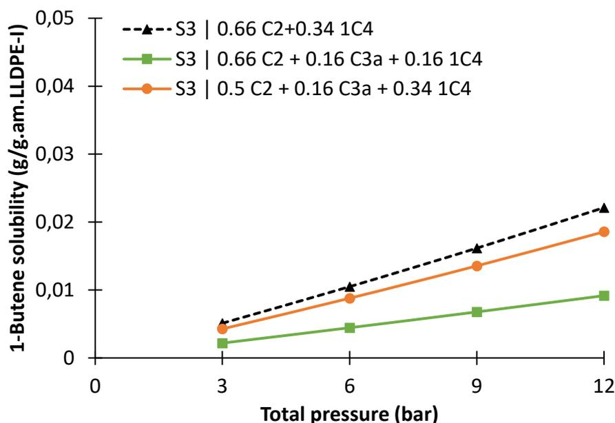
**Figure 77.** 1-Butene partial solubility calculated from SL EoS for ethylene/1-butene/LLDPE-I ternary system and for ethylene/propane/1-butene/LLDPE-I quaternary system at 80°C.  $k_{ij}$  for the ternary system was taken from **Table 20** and for the quaternary system from **Table 25**
