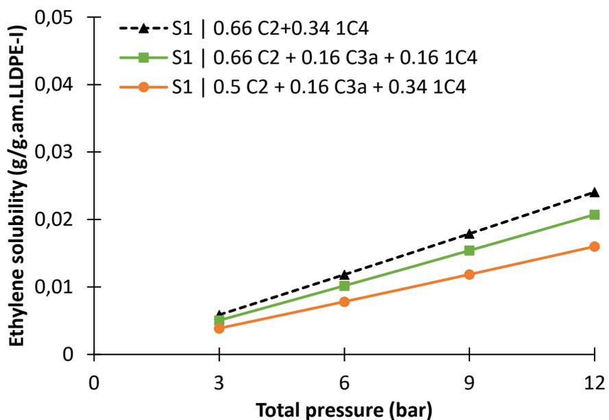
*Figure 76.* Ethylene partial solubility calculated from SL EoS for ethylene/1-butene/LLDPE-I ternary system and for ethylene/propane/1-butene/LLDPE-I quaternary system at 80°C.  $k_{ij}$  for the ternary system was taken from **Table 20** and for the quaternary system from **Table 25**
