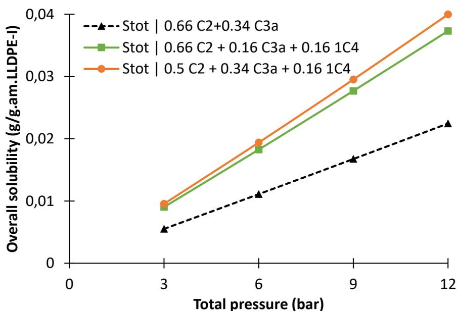
**Figure 78.** Overall solubility calculated from SL EoS for ethylene/propane /LLDPE-I ternary system and for ethylene/propane/1-butene/LLDPE-I quaternary system at 80°C.  $k_{ij}$  for the ternary system was taken from **Table 20** and for the quaternary system from **Table 25**
