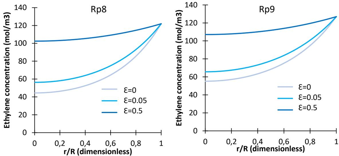
*Figure 116. Effect of polymer porosity on ethylene concentration gradient at 40 minutes of the reaction as a function of the normalized particle radius for 7 bar of ethylene, 1 bar of hydrogen and 1 ( $R_{p8}$ ) and 2 bar ( $R_{p9}$ ) of n-pentane*
