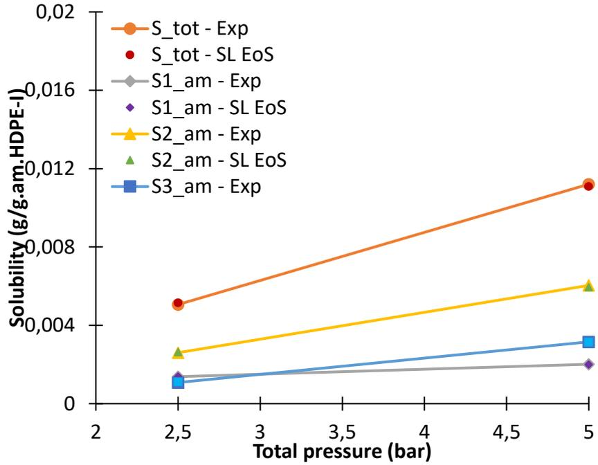
Figure 66. Experimental and SL modeling of overall and partial solubility of each component in ethylene/propane/1-butene/HDPE-I at 73°C. Gas phase composition of the mixture is given in Table 23.  $k_{ij}$  are given in Table 25
