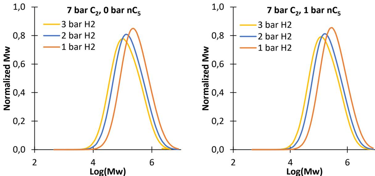
**Figure 120.** Effect of hydrogen on the molecular weight distribution calculated with the method of moments at 7 bar of ethylene and 0 and 1 bar of n-pentane, at 80°C
