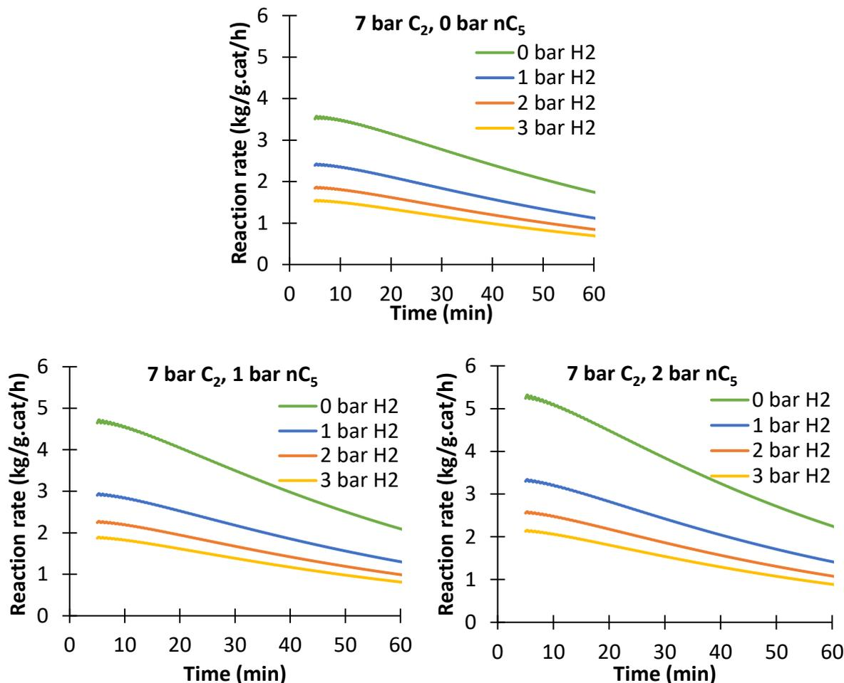
Figure 117. Polymerization rate during the reaction time for 7 bar of ethylene, 0, 1 and 2 bar of  $n$ -pentane and different amounts of hydrogen, at  $80^\circ C$
