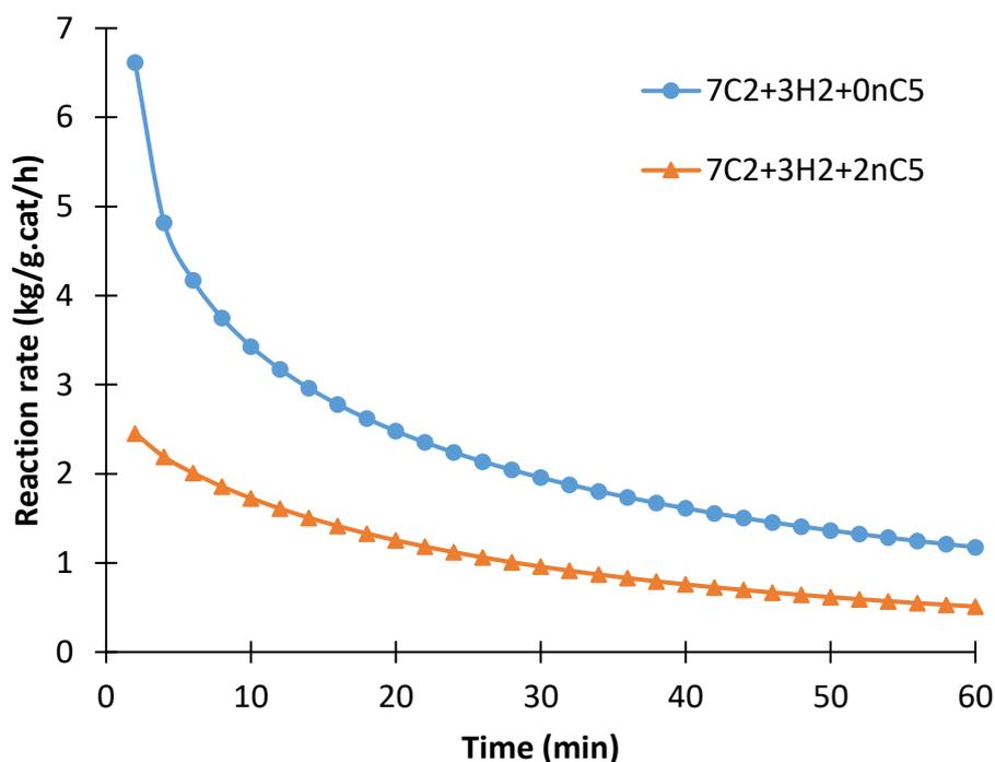
*Figure 151.* Polymerization rate during the reaction time for 7 bar of ethylene, 0, 1 and 2 bar of n-pentane and 3 bar of hydrogen, at 80°C
