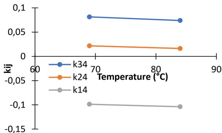
Figure 63. Temperature dependent  $k_{ij}$  interaction parameters between ethylene ( $k_{14}$ ), propane ( $k_{24}$ ), 1-butene ( $k_{34}$ ) and the polymer for ethylene/propane/1-butene/LLDPE-I quaternary system.
