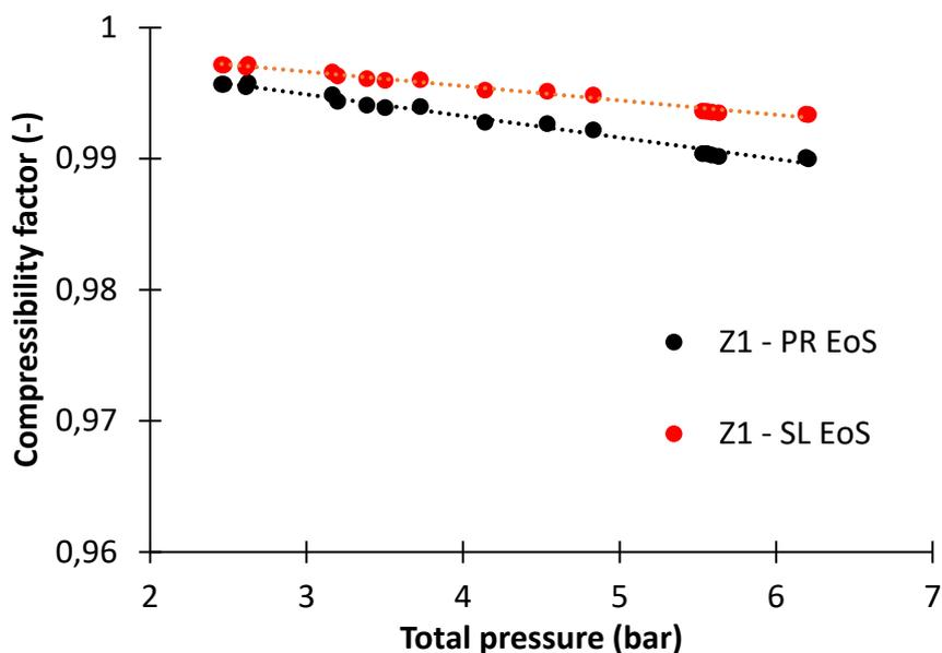
**Figure 70.** Compressibility factor of ethylene in  $C_2/C_3/1C_4/LLDPE-B$  quaternary system at  $70^\circ C$ . The red points represent the compressibility values calculated with Peng-Robinson ( $Z_1 - PR$  EoS) and the black points represent the predictions of the compressibility factor from the ternary SL EoS ( $Z_1 - SL$  EoS). The dashed lines are simply trend lines to guide the eye.
