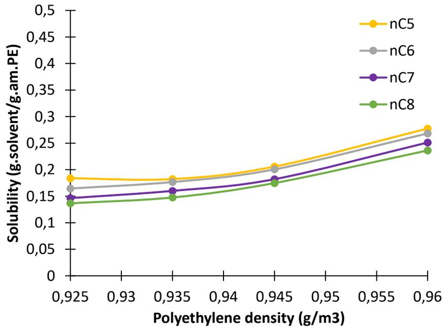
*Figure 140. Solubility (g of solvent / g of amorphous polyethylene) at room temperature of the different solvents in three different PE samples having different densities*
