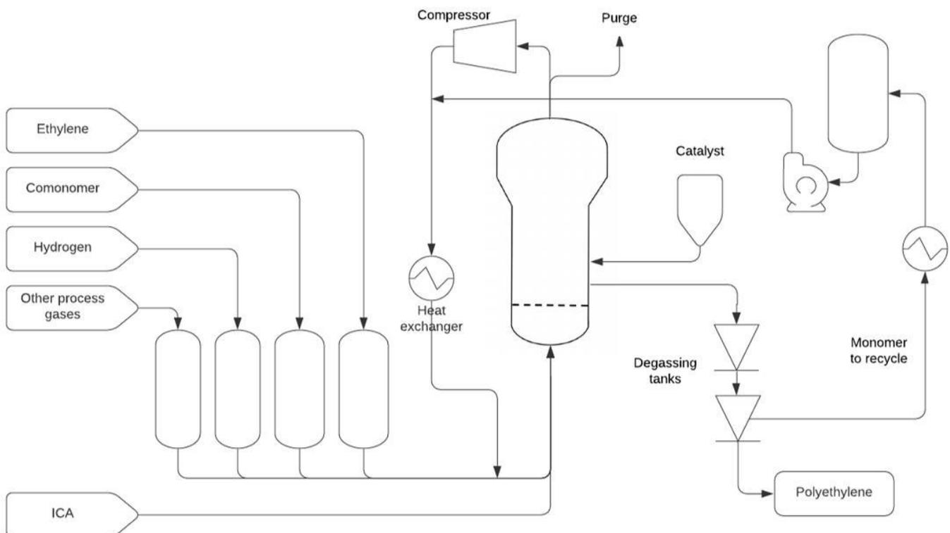
*Figure 4. Scheme of a gas phase process operating in a fluidized bed reactor*
