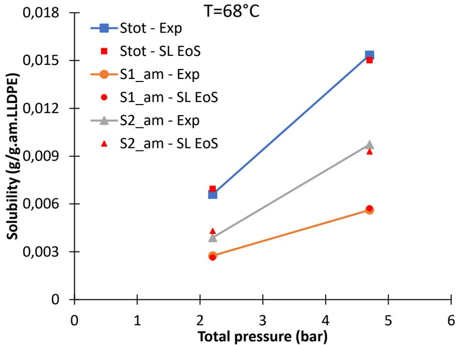
Figure 40. Total ( $S_{tot}$ ) and partial solubility of ethylene ( $S1_{am}$ ) and propylene ( $S2_{am}$ ) in ethylene/propylene/LLDPE-I system at 68°C. The lines represent the experimental solubility and the red points represent the solubility calculated with SL EoS. Gas phase composition is  $x_{C2}=0.475$  and  $x_{C3e}=0.525$  at 68°C.  $k_{ij}$  correlations are given in Table 20
