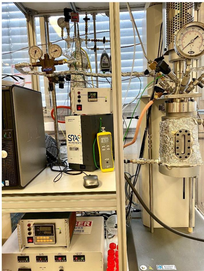
Figure 31. Experimental set-up of the pressure decay method for sorption measurements
