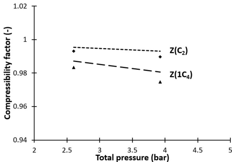
**Figure 23.** Compressibility factor of ethylene ( $C_2$ ) and 1-butene ( $1C_4$ ) in  $C_2/1C_4/LLDPE-B$  mixture. Points represent compressibility values calculated with Peng-Robinson and the lines represent the predictions of the compressibility factor from the ternary SL EoS
