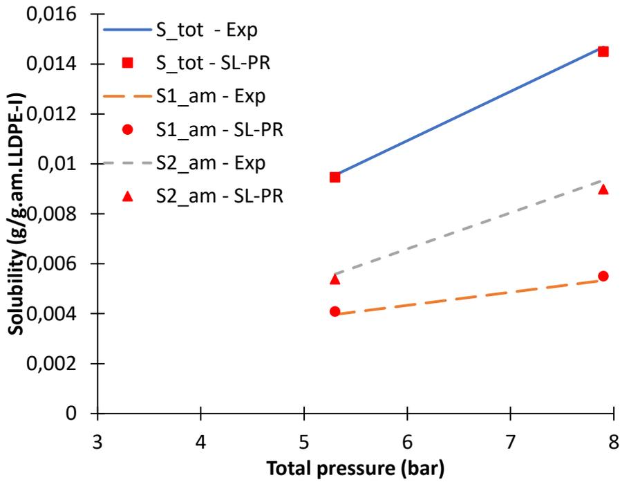
Figure 45. Overall and partial solubility of ethylene/propane/LLDPE-I ternary system at 80°C. The estimation of the partial solubility is achieved by using the SL-PR method. Molar composition of the system is given in Table 19 and  $k_{ij}$  used for this study is given in Table 20
