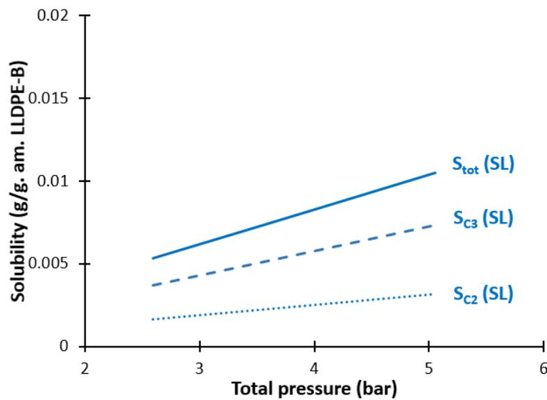
**Figure 24.** Total solubility  $S_{tot}$  (SL), partial solubility of ethylene  $S_{C2}$  (SL) and partial solubility of propane  $S_{C3}$  (SL) in LLDPE-B at 70°C from SL-PR method (ternary system  $C_2/C_3/LLDPE-B$ ).  $k_{ij}$  are defined in Table 15
