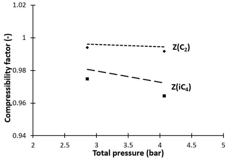
**Figure 22.** Compressibility factor of ethylene ( $C_2$ ) and isobutane ( $iC_4$ ) in  $C_2/iC_4/LLDPE-B$  mixture. Points represent compressibility values calculated with Peng-Robinson and the lines represent the predictions of the compressibility factor from the ternary SL EoS
