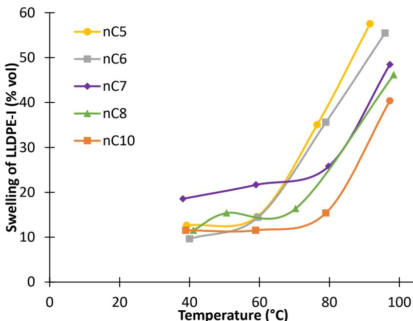
*Figure 146.* Swelling of LLDPE-I (in % vol) powders in presence of different solvents at different temperatures. (Each experiment was repeated at least twice under the same conditions)
