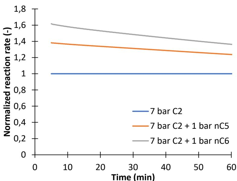
**Figure 122.** Polymerization rate during the reaction time for 7 bar of ethylene with 1 bar of n-pentane and n-hexane normalized by the polymerization rate without ICA at 80°C
