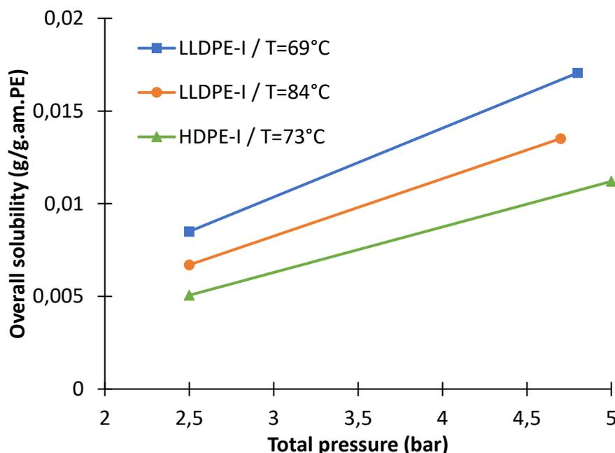
**Figure 56.** Overall solubility of ethylene/propane/1-butene in different PE types (HDPE-I and LLDPE-I) and at different temperatures, using pressure decay method. Gas phase composition is shown in **Table 23**. PE characteristics are shown in **Table 1**.
