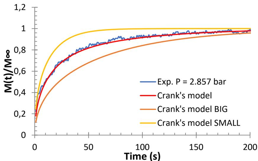
**Figure 86.** Sorption rates of ethylene/isobutane/LLDPE-B ternary system at total pressure of 2.857 bars and 70°C obtained through gravimetric method and Crank's diffusion equation for particles with two sizes of granules. Molar composition is:  $x_{C2} = 0.485$  and  $x_{iC4} = 0.515$ .
