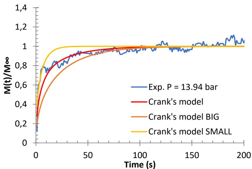
**Figure 85.** Sorption rates of ethylene/LLDPE-B binary system for a total pressure of 13.94 bar at 70°C obtained through gravimetric method and Crank's diffusion equation for particles with two sizes of granules
