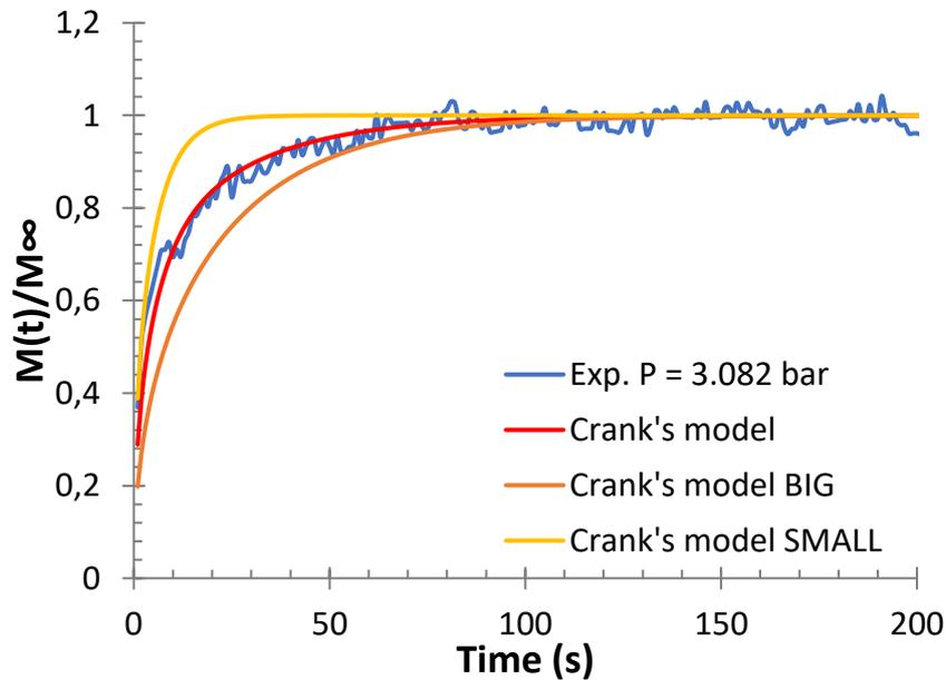
**Figure 92.** Sorption rates of ethylene/propane/LLDPE-B ternary system at total pressure of 3.082 bars and 70°C obtained through gravimetric method and Crank's diffusion equation for particles with two sizes of granules. Molar composition is:  $x_{C_2} = 0.509$  and  $x_{iC_4} = 0.491$ .
