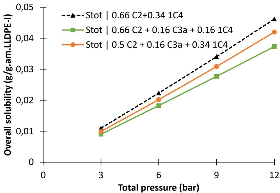
*Figure 75.* Overall solubility calculated from SL EoS for ethylene/1-butene/LLDPE-I ternary system and for ethylene/propane/1-butene/LLDPE-I quaternary system at 80°C.  $k_{ij}$  for the ternary system was taken from **Table 20** and for the quaternary system from **Table 25**
