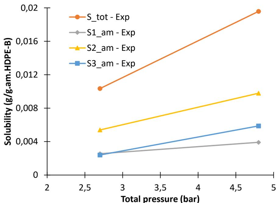
**Figure 60.** Total and partial solubility of ethylene/propane/1-butene/HDPE-B system at 75°C.  $S_{tot}$ ,  $S1_{am}$ ,  $S2_{am}$  and  $S3_{am}$  are the total solubility of the mixture and the overall solubility of ethylene, propane and 1-butene in the amorphous phase of the polymer, respectively. Gas phase composition of the mixture is given in **Table 23**
