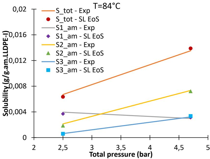
Figure 65. Experimental and SL modeling of overall and partial solubility of each component in ethylene/propane/1-butene/LLDPE-I at 84°C. Gas phase composition of the mixture is given Table 23.  $k_{ij}$  are given in Table 25
