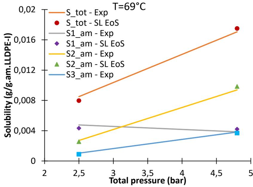
Figure 64. Experimental and SL modeling of overall and partial solubility of each component in ethylene/propane/1-butene/LLDPE-I at 69°C. Gas phase composition of the mixture is given in Table 23.  $k_{ij}$  are given in Table 25
