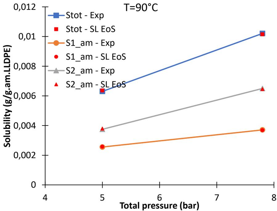
Figure 39. Total ( $S_{tot}$ ) and partial solubility of ethylene ( $S1_{am}$ ) and propane ( $S2_{am}$ ) in ethylene/propane/LLDPE-I system at 90°C. The lines represent the experimental solubility and the red points represent the solubility calculated with SL EoS. Gas phase composition is  $x_{C2}=0.497$  and  $x_{C3a}=0.503$  at 90°C.  $k_{ij}$  correlations are given in Table 20
