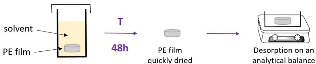
*Figure 126. Scheme of the desorption experiments of PE films and granules at room temperature.*
