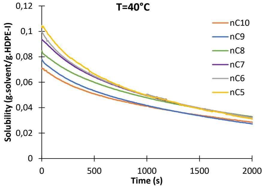
Figure 142. Solubility of different solvents ( $nC_5$ ,  $nC_6$ ,  $nC_7$ ,  $nC_8$ ,  $nC_9$ ,  $nC_{10}$ ) in HDPE-I granules at  $40^\circ\text{C}$  (Each experiment was repeated at least two times under the same conditions)
