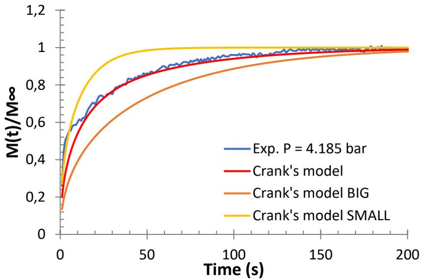
**Figure 106.** Sorption rates of ethylene/isobutane/1-butene/LLDPE-B quaternary system at total pressure of 4.185 bars and 70°C obtained through gravimetric method and Crank's diffusion equation for particles with two sizes of granules for **Composition 4**. Molar composition is:  $x_{iC4}=0.43$ ,  $x_{1C4}=0.17$  and  $x_{C2}=0.40$
