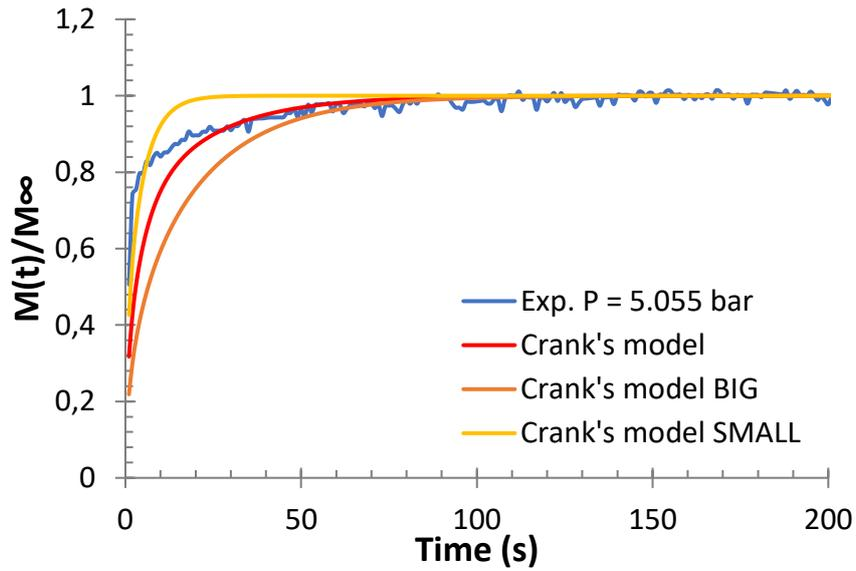
**Figure 93.** Sorption rates of ethylene/propane/LLDPE-B ternary system at total pressure of 5.055 bars and 70°C obtained through gravimetric method and Crank's diffusion equation for particles with two sizes of granules. Molar composition is:  $x_{C_2} = 0.509$  and  $x_{iC_4} = 0.491$ .
