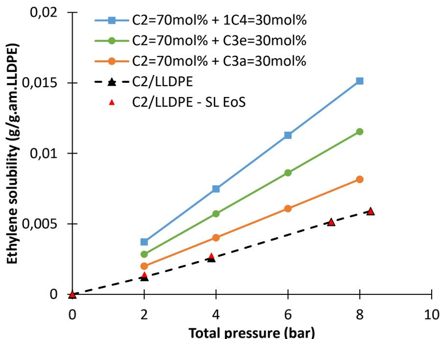
**Figure 53.** Binary solubility of ethylene in LLDPE taken from<sup>21</sup> (dotted lines) and from SL EoS (points) and the partial ternary solubility of ethylene in presence of 30 mol% of propane, propylene and 1-butene in LLDPE-I at 80°C.  $k_{ij}$  for the studied ternary systems at the temperature of interest are defined in Table 20 and for the ethylene/LLDPE binary system in Table 22.
