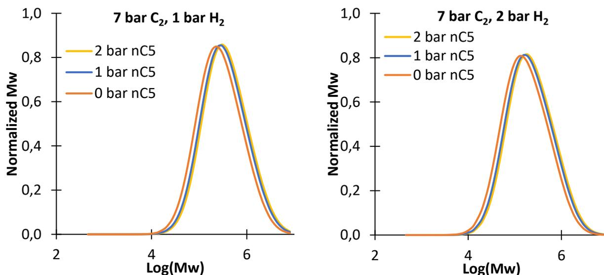
*Figure 121. Effect of n-pentane on the molecular weight distribution calculated with the method of moments at 7 bar of ethylene and 1 and 2 bar of hydrogen, at 80°C*
