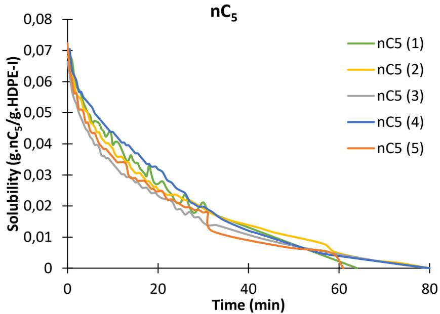
*Figure 134. Solubility of n-pentane in HDPE-I granules at room temperature (the same experiment at the same conditions was repeated five times)*
