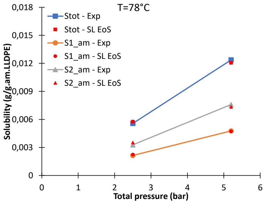
Figure 41. Total ( $S_{tot}$ ) and partial solubility of ethylene ( $S1_{am}$ ) and propylene ( $S2_{am}$ ) in ethylene/propylene/LLDPE-I system at 68°C. The lines represent the experimental solubility and the red points represent the solubility calculated with SL EoS. Gas phase composition is  $x_{C2}=0.395$  and  $x_{C3e}=0.605$  at 68°C.  $k_{ij}$  correlations are given in Table 20
