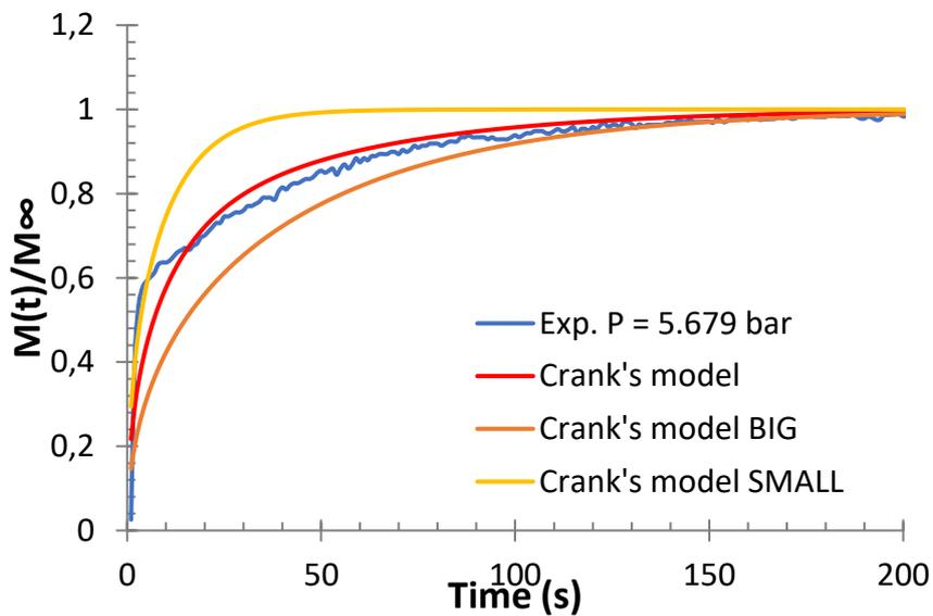
**Figure 107.** Sorption rates of ethylene/isobutane/1-butene/LLDPE-B quaternary system at total pressure of 5.679 bars and 70°C obtained through gravimetric method and Crank's diffusion equation for particles with two sizes of granules for **Composition 4**. Molar composition is:  $x_{iC4}=0.43$ ,  $x_{1C4}=0.17$  and  $x_{C2}=0.40$
