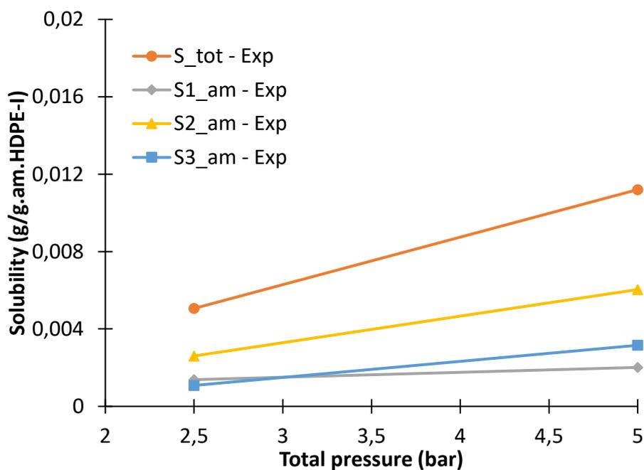
**Figure 59.** Total and partial solubility of ethylene/propane/1-butene/HDPE-I system at 73°C.  $S_{tot}$ ,  $S_{1_{am}}$ ,  $S_{2_{am}}$  and  $S_{3_{am}}$  are the total solubility of the mixture and the overall solubility of ethylene, propane and 1-butene in the amorphous phase of the polymer, respectively. Gas phase composition of the mixture is given in **Table 23**
