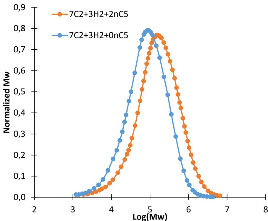
*Figure 152.* Molecular weight distribution calculated using HT-GPC for polymer produced with 7 bar of ethylene, 3 bar of hydrogen and 0 and 2 bar of n-pentane at 80°C.
