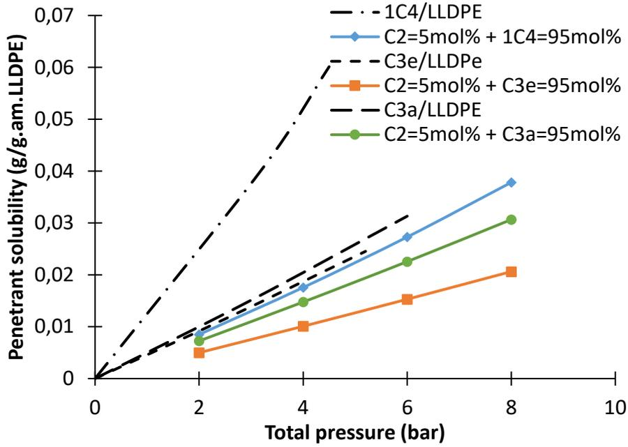
Figure 54. Binary solubility of 1-butene (1C4), propylene (C3e) and propane (C3a) and the partial ternary solubility of these penetrants with 5 mol% of ethylene in LLDPE at 80°C, calculated with SL EoS.  $k_{ij}$  for the studied ternary systems at the temperature of interest are defined in Table 20 and for the ethylene/LLDPE binary system in Table 22.
