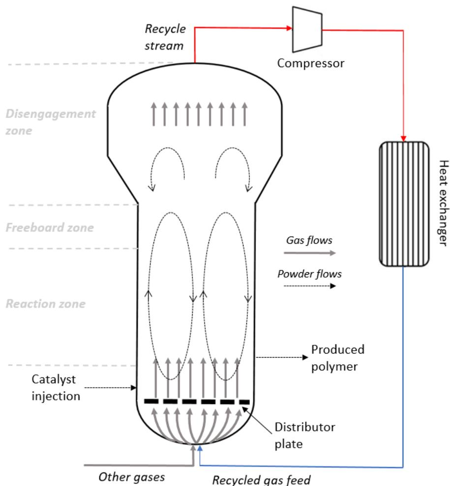
Figure 5. Scheme of a fluidized bed reactor for olefin polymerization. Adapted from <sup>5</sup>
