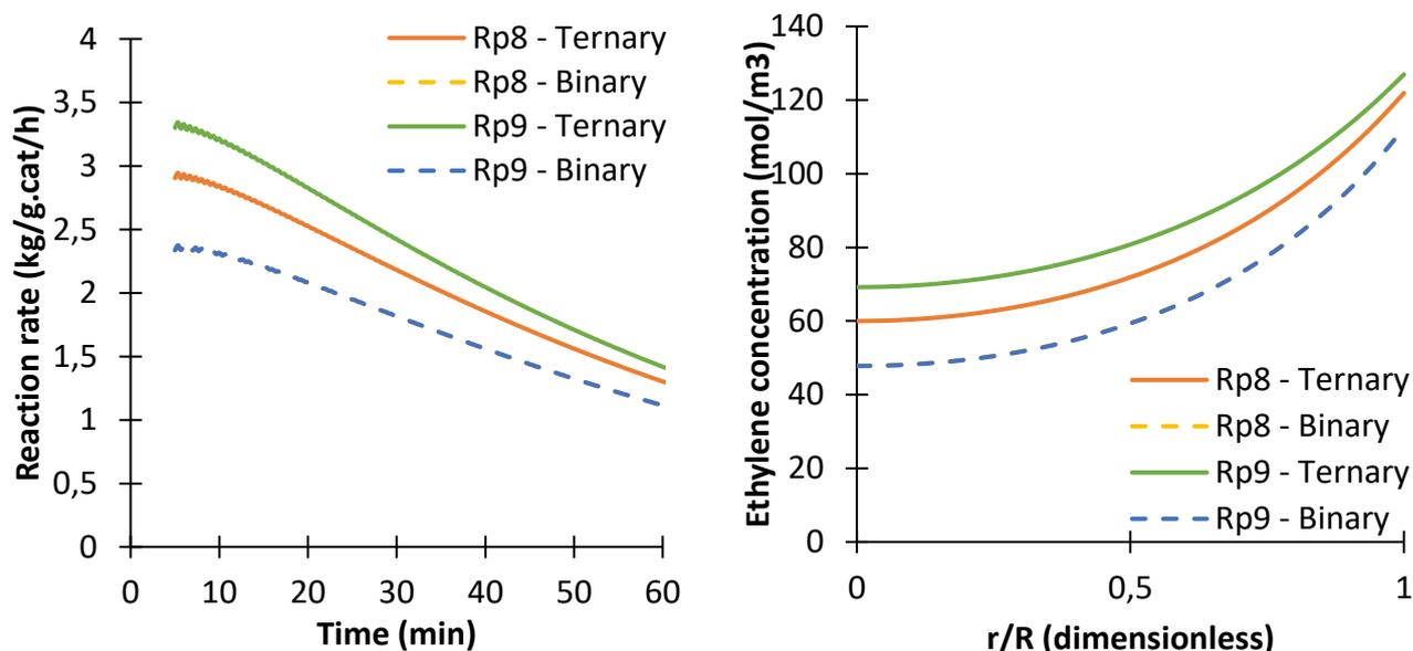
**Figure 114.** Effect of thermodynamic model (i.e. binary, ternary) on the polymerization rate during the reaction and ethylene concentration gradients as a function of the normalized particle radius. The gas phase composition of Rp8 (1 bar C<sub>5</sub>, 1 bar H<sub>2</sub>) and Rp9 (2 bar C<sub>5</sub>, 1 bar H<sub>2</sub>) is described in Table 33. The concentration are taken at 40 minutes of the reaction. The porosity is  $\epsilon=0.05$ .
