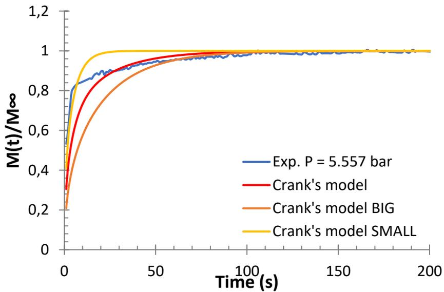
**Figure 100.** Sorption rates of ethylene/propane/1-butene/LLDPE-B quaternary system at total pressure of 5.557 bars and 70°C obtained through gravimetric method and Crank's diffusion equation for particles with two sizes of granules for **Composition 2**. Molar composition is:  $x_{C3}=0.42$ ,  $x_{1C4}=0.17$  and  $x_{C2}=0.41$
