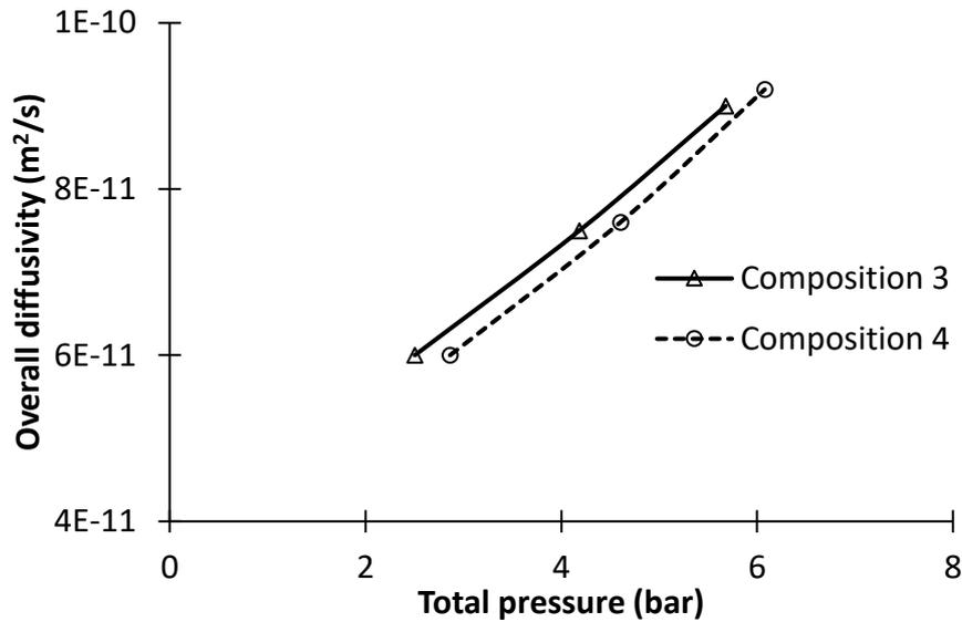
*Figure 108.* Comparison of the diffusivity of ethylene/isobutane/1-butene/LLDPE-B quaternary system obtained from the fitting of Crank's diffusion equation for particles with two sizes of granules from *Composition 3 and Composition 4.*
