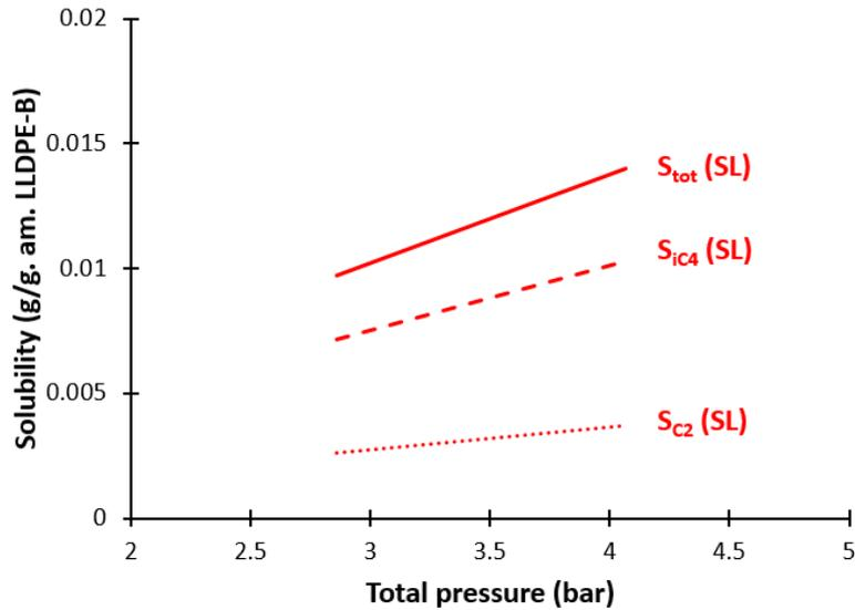
**Figure 25.** Total solubility  $S_{tot}$  (SL), partial solubility of ethylene  $S_{C2}$  (SL) and partial solubility of isobutane  $S_{iC4}$  (SL) in LLDPE-B at 70°C from SL EoS (ternary system  $C_2/iC_4/LLDPE-B$ ).  $k_{ij}$  are defined in **Table 15**
