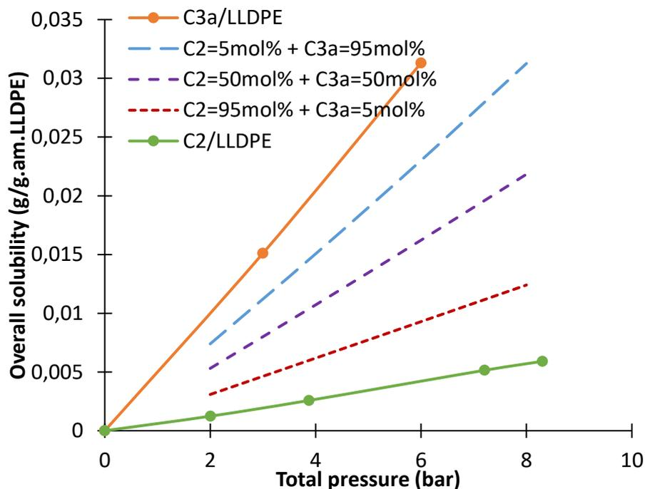
**Figure 49.** Solubility of binary ethylene/LLDPE (C2) and propane/LLDPE (C3a) systems and overall solubility of their mixture in ternary system of ethylene/propane/LLDPE at 80°C, calculated with SL EoS. Different composition of the gaseous mixture in the ternary system is shown.  $k_{ij}$  for binary systems are defined in **Table 22** and for ternary systems in **Table 20**
