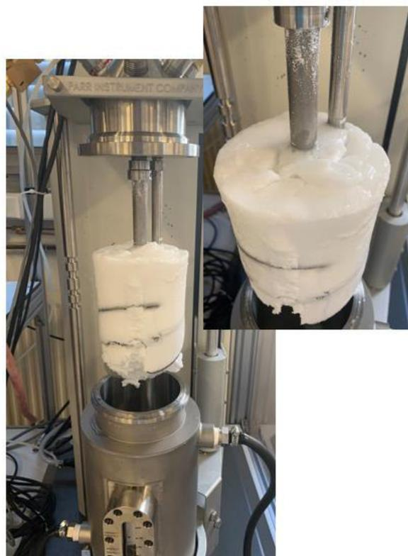
*Figure 129. Example of plasticization of MDPE-B powders in presence of n-hexane at 90°C*
