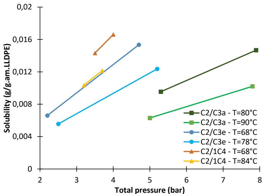
**Figure 37.** Total solubility of ethylene/propane, ethylene/propylene and ethylene/1-butene in LLDPE-I at temperatures between 68-90°C. Gas compositions of the different systems is given in **Table 19**
