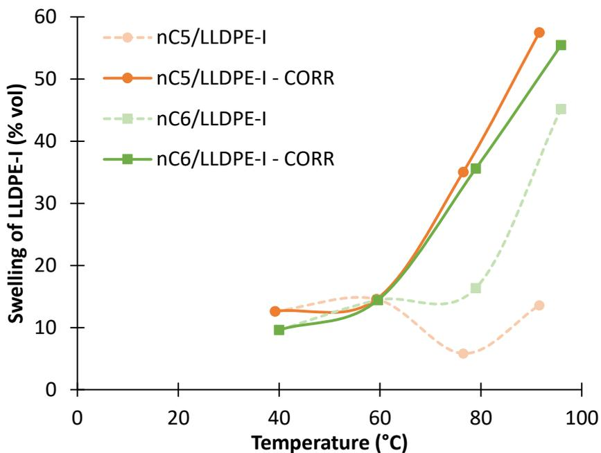
Figure 148. Swelling measured experimentally and corrected with LLDPE-I dissolution in the solvent given in Table 41
