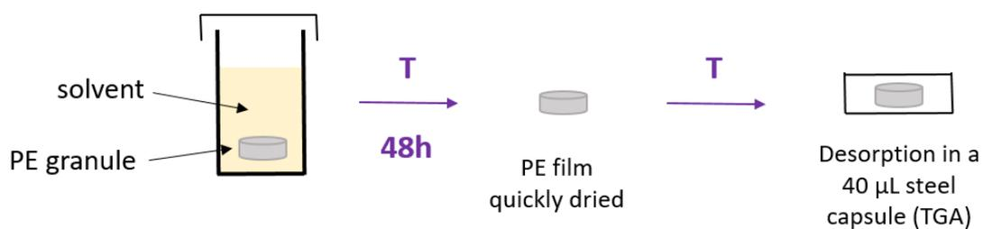
*Figure 127. Schema of the desorption experiments of PE granules at high temperature*
