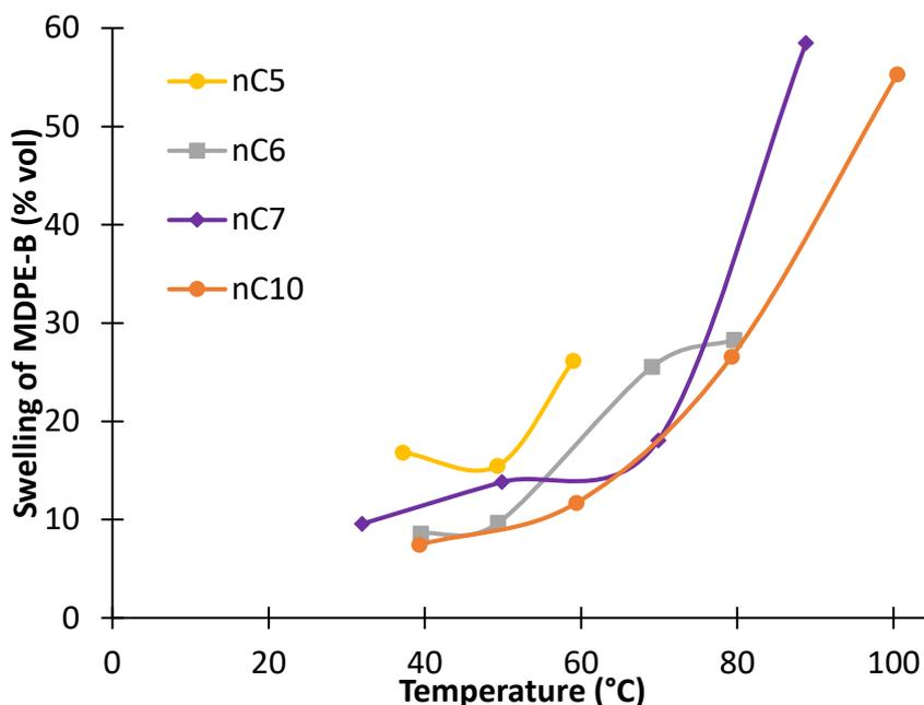
*Figure 147.* Swelling of MDPE-B (in % vol) powders in presence of different solvents at different temperatures. (Each experiment was repeated at least twice under the same conditions).
