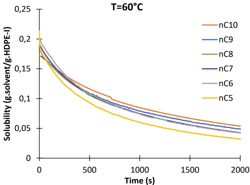
Figure 143. Solubility of different solvents ( $nC_5$ ,  $nC_6$ ,  $nC_7$ ,  $nC_8$ ,  $nC_9$ ,  $nC_{10}$ ) in HDPE-I granules at  $60^\circ\text{C}$  (Each experiment was repeated at least two times under the same conditions)
