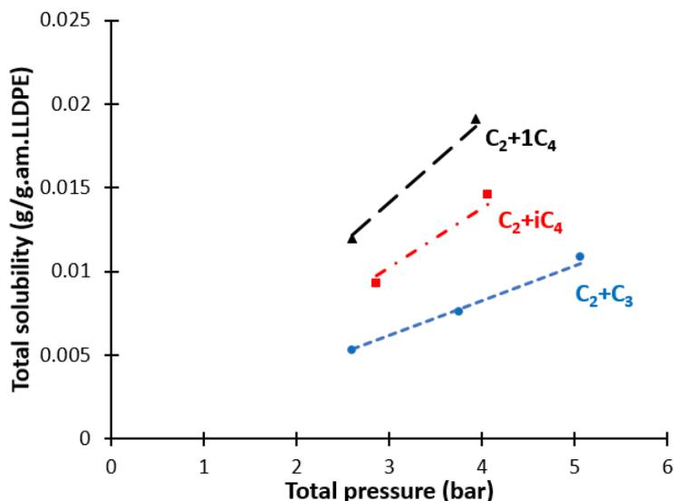
**Figure 20.** Total solubility of ethylene/penetrant mixture in LLDPE-B in presence of different penetrants at 70°C. Points represent experimental values (average of 2 or 3 runs) and the lines represent the predictions of the SL EoS with the fitted parameters.  $k_{ij}$  are defined in Table 15
