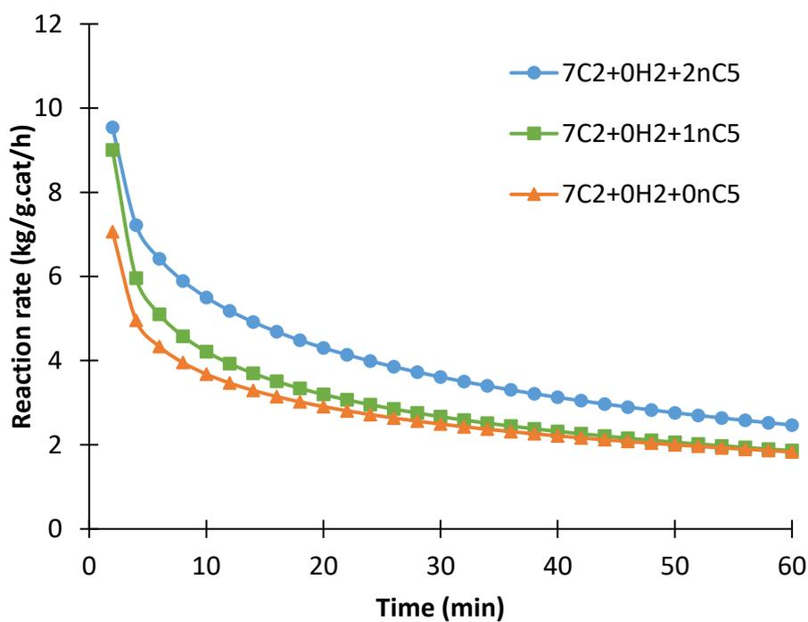
Figure 150. Polymerization rate during the reaction time for 7 bar of ethylene, 0, 1 and 2 bar of n-pentane and without hydrogen, at 80°C
