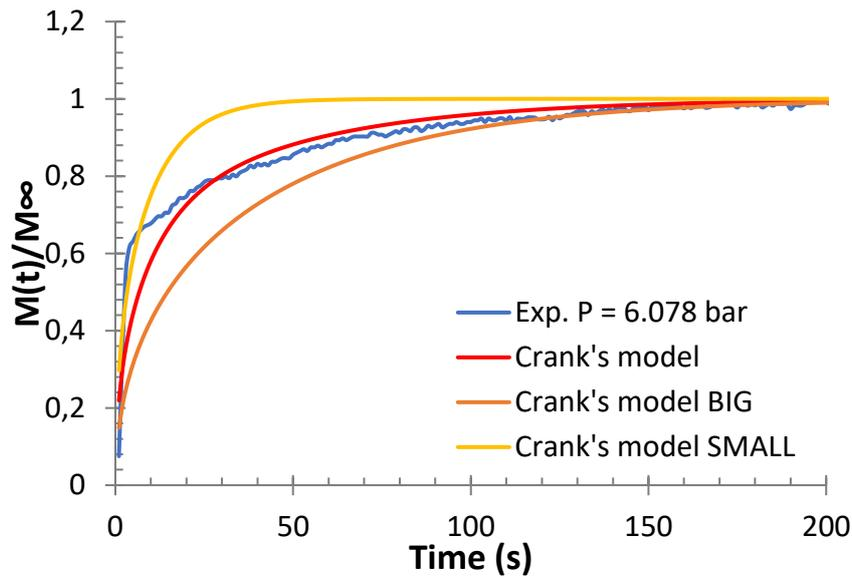
**Figure 104.** Sorption rates of ethylene/isobutane/1-butene/LLDPE-B quaternary system at total pressure of 6.078bars and 70°C obtained through gravimetric method and Crank's diffusion equation for particles with two sizes of granules for **Composition 3**. Molar composition is:  $x_{iC4}=0.37$ ,  $x_{1C4}=0.23$  and  $x_{C2}=0.40$ .
