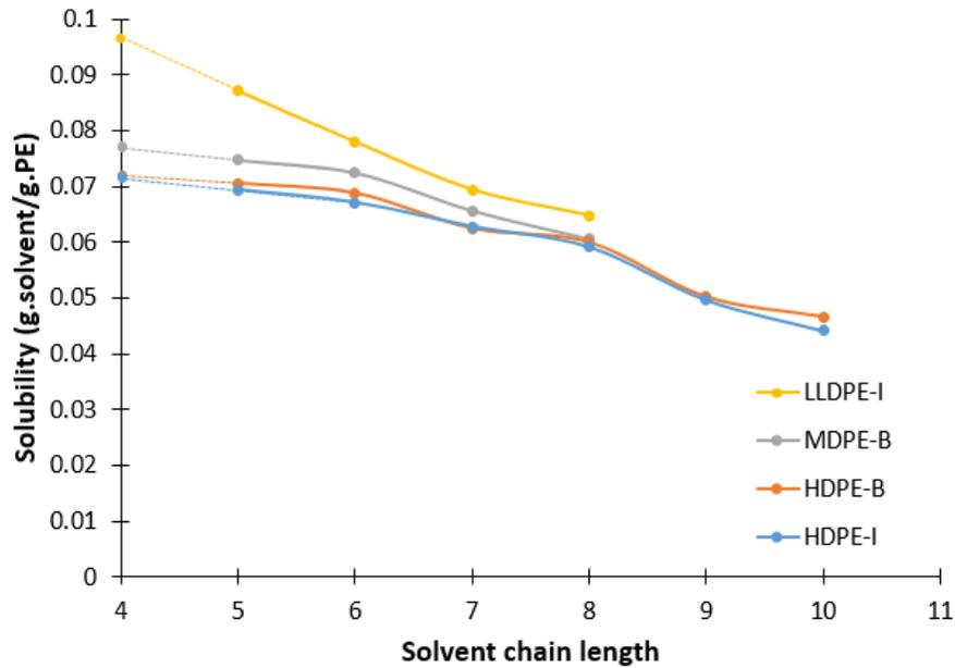
*Figure 138.* Solubility (g of solvent / g of polyethylene) at room temperatures in the different PE samples with respect to the solvent chain length.
