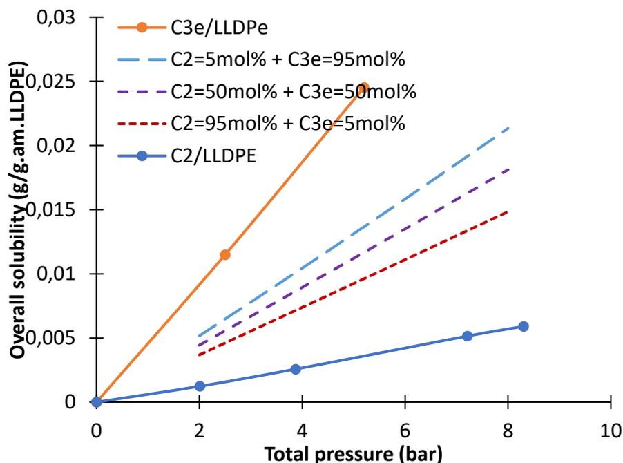
**Figure 50.** Solubility of binary ethylene/LLDPE (C2) and propylene/LLDPE (C3e) systems and overall solubility of their mixture in ternary system of ethylene/propylene/LLDPE at 80°C, calculated with SL EoS. Different composition of the gaseous mixture in the ternary system is shown.  $k_{ij}$  for binary systems are defined in Table 22 and for ternary systems in Table 20
