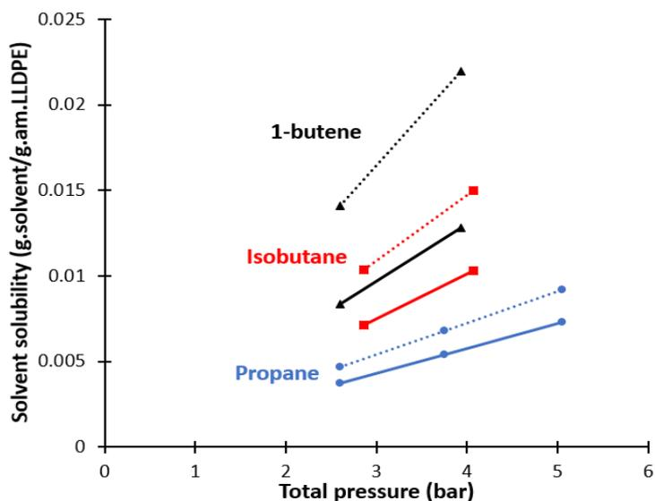
**Figure 29.** Solubility of propane, isobutane and 1-butene in binary (diluent/LLDPE) and ternary (ethylene/diluent/LLDPE) systems using SL EoS.  $k_{ij}$  for ternary systems are defined in **Table 15**.  $k_{ij}$  for binary systems are defined in **Table 8**. The lines represent diluent partial solubility in ternary systems and the dotted lines represent diluent solubility in binary systems.
