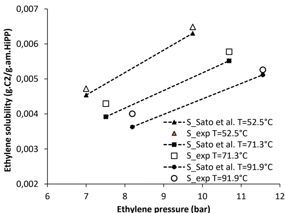
**Figure 33.** Ethylene solubility in the amorphous phase of HiPP at different temperatures and ethylene pressures. The lines represent the solubility from Sato et al.<sup>12</sup> and the points represent the experimental solubility measured with the pressure decay method.
