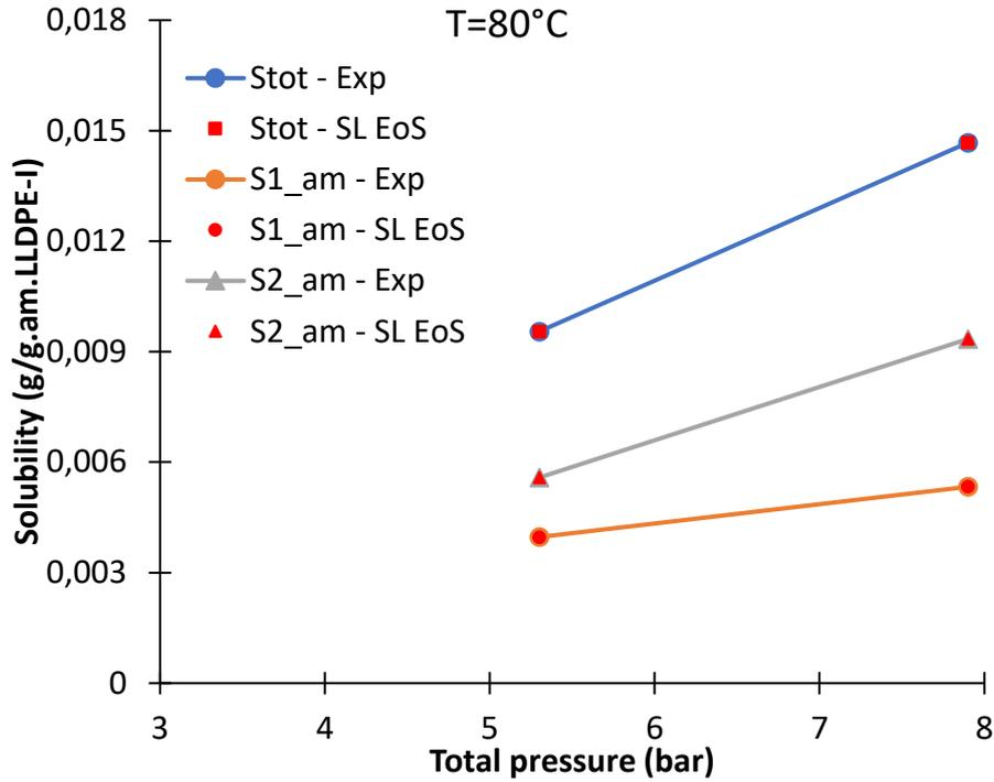
Figure 38. Total ( $S_{tot}$ ) and partial solubility of ethylene ( $S1_{am}$ ) and propane ( $S2_{am}$ ) in ethylene/propane/LLDPE-I system at 80°C. The lines represent the experimental solubility and the red points represent the solubility calculated with SL EoS. Gas phase composition is  $x_{C2}=0.497$  and  $x_{C3a}=0.503$  at 80°C.  $k_{ij}$  correlations are given in Table 20
