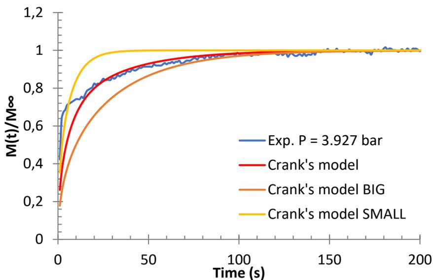
**Figure 90.** Sorption rates of ethylene/1-butene/LLDPE-B ternary system at a total pressure of 3.927 bars and 70°C obtained through gravimetric method and Crank's diffusion equation for particles with two sizes of granules. Molar composition is:  $x_{C_2} = 0.617$  and  $x_{1C_4} = 0.383$ .
