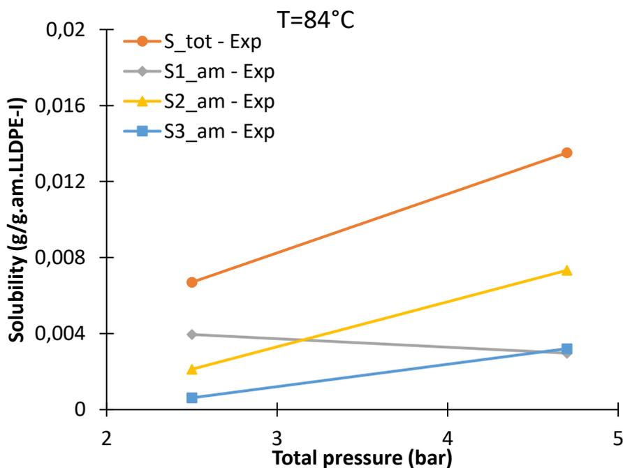
**Figure 58.** Total and partial solubility of ethylene/propane/1-butene/LLDPE-I system at 84°C.  $S_{tot}$ ,  $S_{1_{am}}$ ,  $S_{2_{am}}$  and  $S_{3_{am}}$  are the total solubility of the mixture and the overall solubility of ethylene, propane and 1-butene in the amorphous phase of the polymer, respectively. Gas phase composition of the mixture is given in **Table 23**
