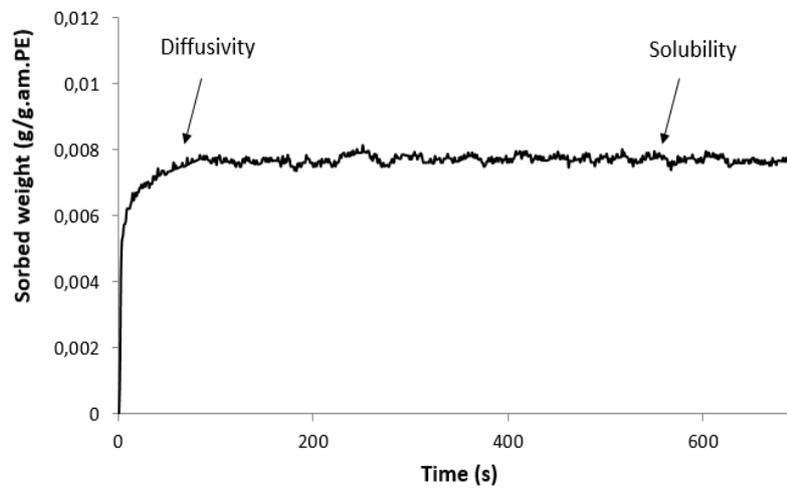
*Figure 81. Sorbed weight measured with a magnetic suspension balance*
