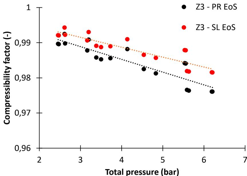
**Figure 72.** Compressibility factor of 1-butene in  $C_2/C_3/1C_4/LLDPE-B$  quaternary system at  $70^\circ C$ . The red points represent the compressibility values calculated with Peng-Robinson ( $Z_1 - PR$  EoS) and the black points represent the predictions of the compressibility factor from the ternary SL EoS ( $Z_1 - SL$  EoS). The dashed lines are simply trend lines to guide the eye.
