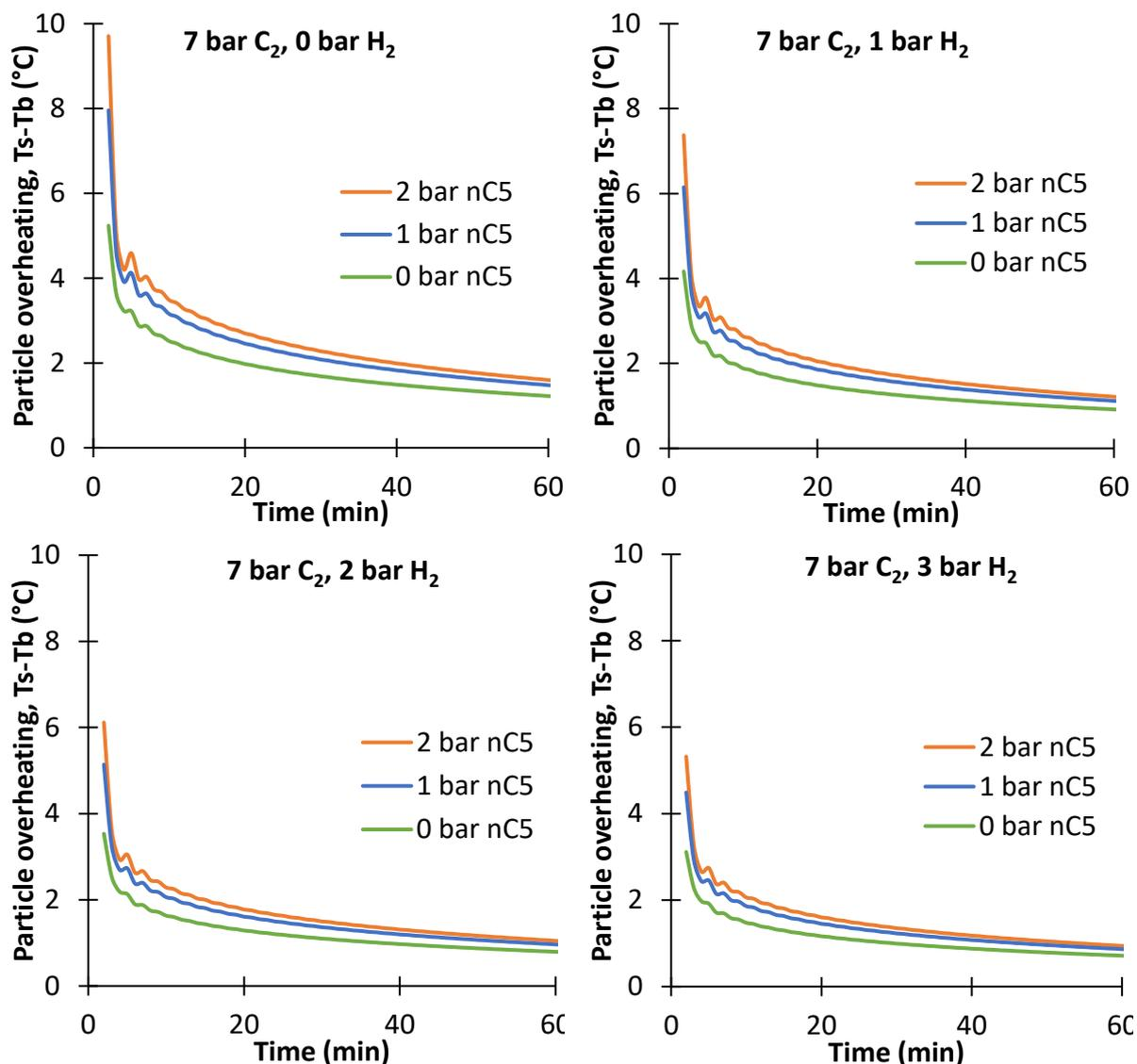
Figure 119. Particle overheating during ethylene polymerization 7 bar of ethylene, 0-2 bar of n-pentane and 1-3 bar of hydrogen at 80°C
