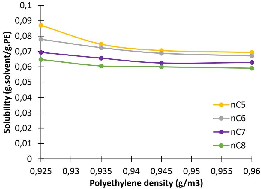
*Figure 139.* Solubility (g of solvent / g of polyethylene) at room temperature of the different solvents in three different PE samples having different densities.
