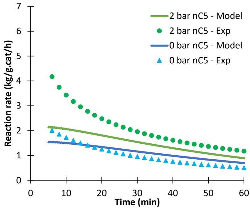
Figure 112. Polymerization rate calculated with the PFM and the experimental data of 7 bar of ethylene, with 3 bar of hydrogen and different amounts of n-pentane, at 80°C
