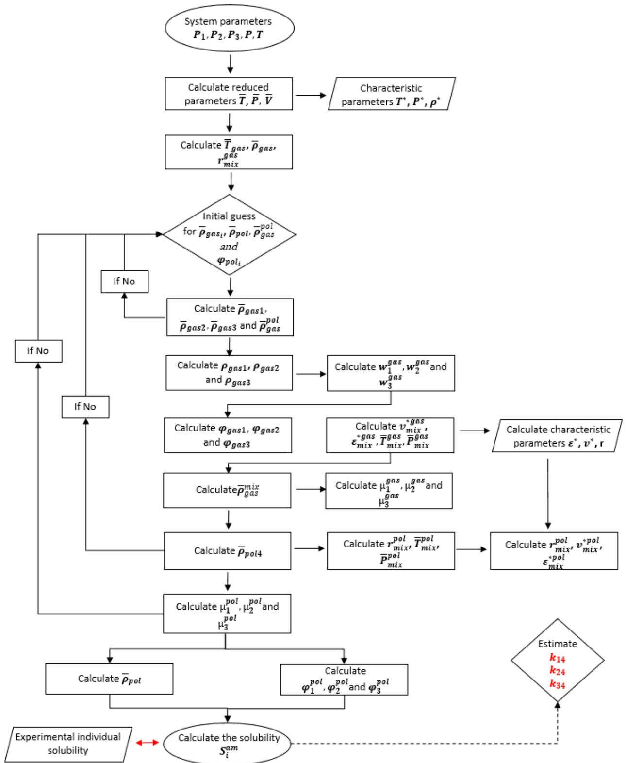
Figure 36. Flowchart for the modeling of quaternary systems with Sanchez-Lacombe Equation of State
