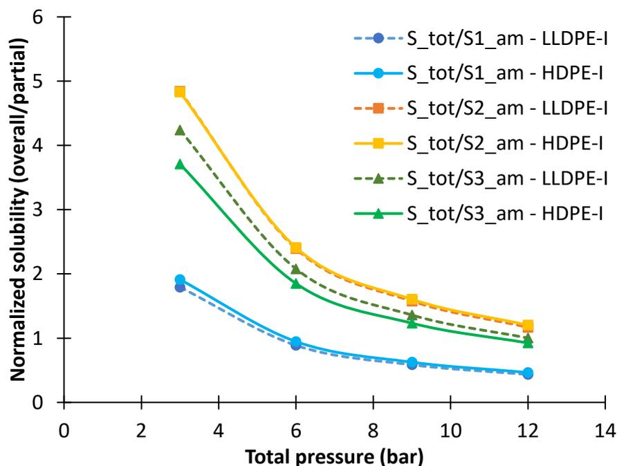
**Figure 68.** Overall solubility of ethylene/propane/1-butene/PE quaternary system normalized by the partial solubility of each component in HDPE-I (lines) and LLDPE-I (dotted lines) at 73°C. Gas phase composition for both system is  $x_{C_2}=0.66$ ,  $x_{C_{3a}}=0.16$  and  $x_{1C_4}=0.16$ .  $k_{ij}$  are given in **Table 25**
