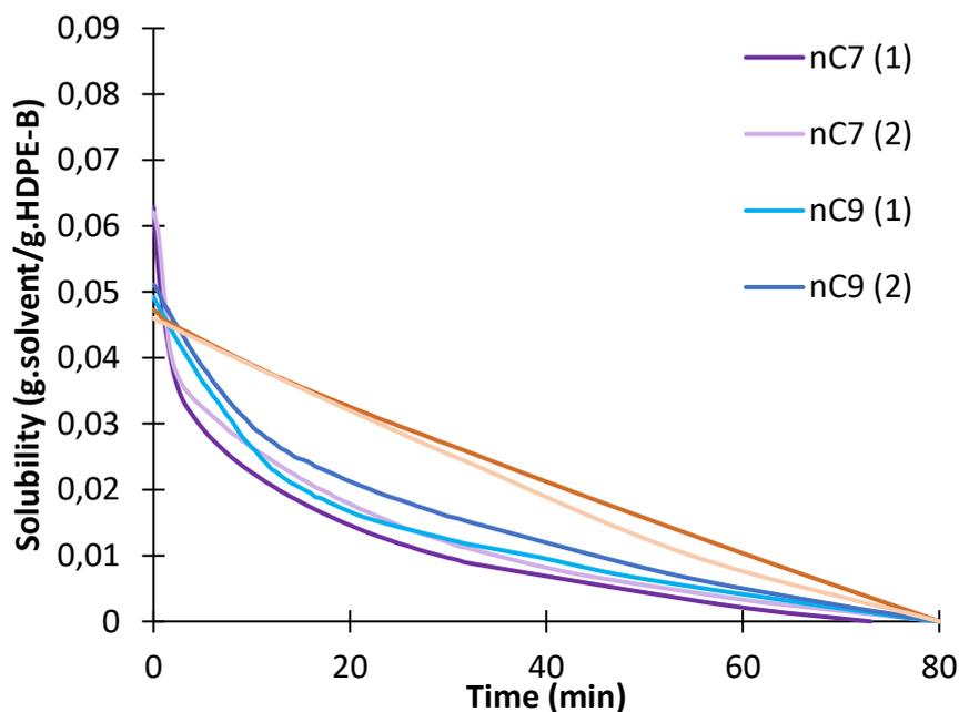
*Figure 135. Solubility of n-heptane, n-nonane and n-decane in HDPE-B films at room temperature (the same experiment at the same conditions was repeated 2 times)*
