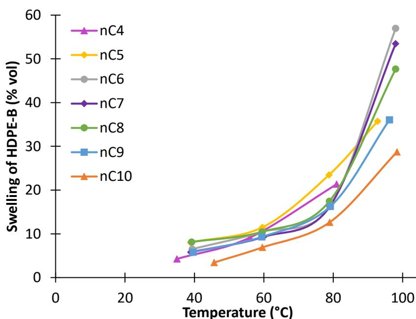
*Figure 145. Swelling of HDPE-B (in % vol) powders in presence of different solvents at different temperatures. (Each experiment was repeated at least twice under the same conditions)*
