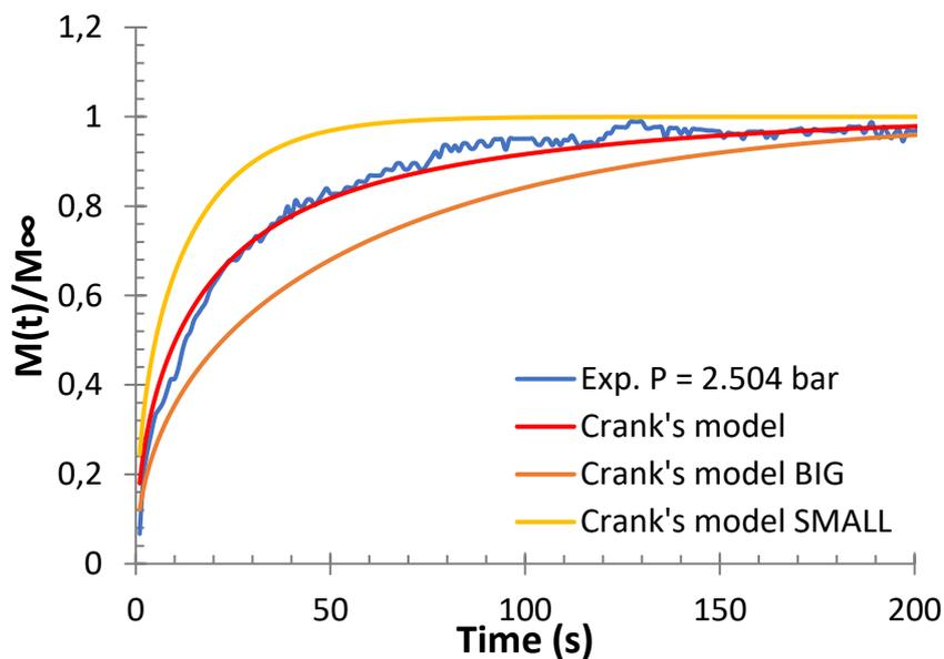
**Figure 105.** Sorption rates of ethylene/isobutane/1-butene/LLDPE-B quaternary system at total pressure of 2.504 bars and 70°C obtained through gravimetric method and Crank's diffusion equation for particles with two sizes of granules for **Composition 4**. Molar composition is:  $x_{iC4}=0.43$ ,  $x_{1C4}=0.17$  and  $x_{C2}=0.40$
