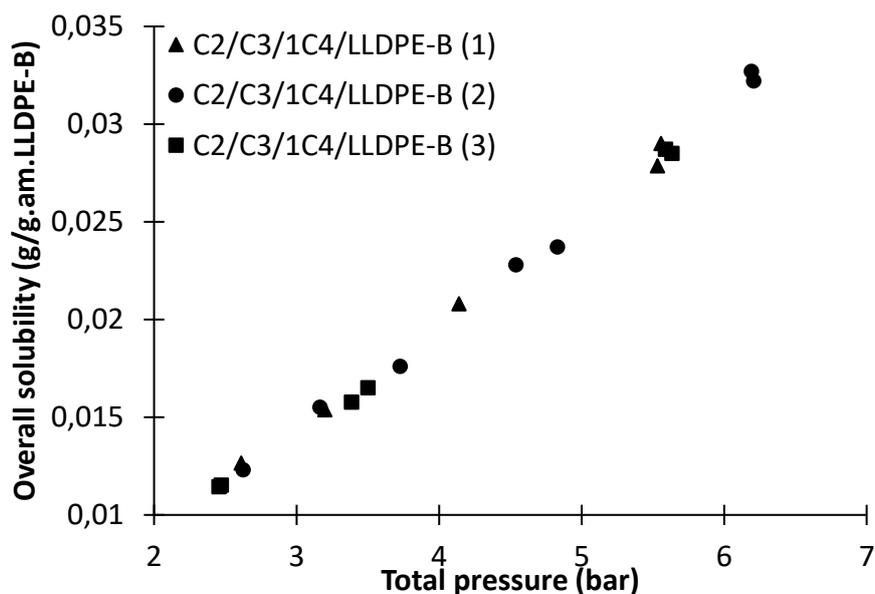
**Figure 61.** Overall solubility of quaternary system of ethylene/propane/1-butene/LLDPE-B at 70°C with different composition of the gas-phase. Gas-phase composition for each experiment is  $x_{C_3}=0.42$  and  $x_{1C_4}=0.17$  for (1),  $x_{C_3}=0.39$  and  $x_{1C_4}=0.23$  for (2) and  $x_{C_3}=0.34$  and  $x_{1C_4}=0.25$  for (3)
