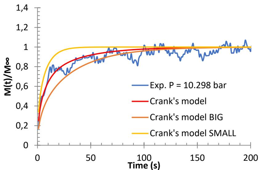
**Figure 84.** Sorption rates of ethylene/LLDPE-B binary system for a total pressure of 10.298 bar at 70°C obtained through gravimetric method and Crank's diffusion equation for particles with two sizes of granules
