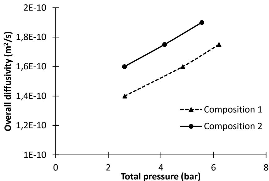
**Figure 101.** Comparison of the diffusivity of ethylene/propane/1-butene/LLDPE-B quaternary system obtained from the fitting of Crank's diffusion equation for particles with two sizes of granules from **Composition 1** and **Composition 2**.
