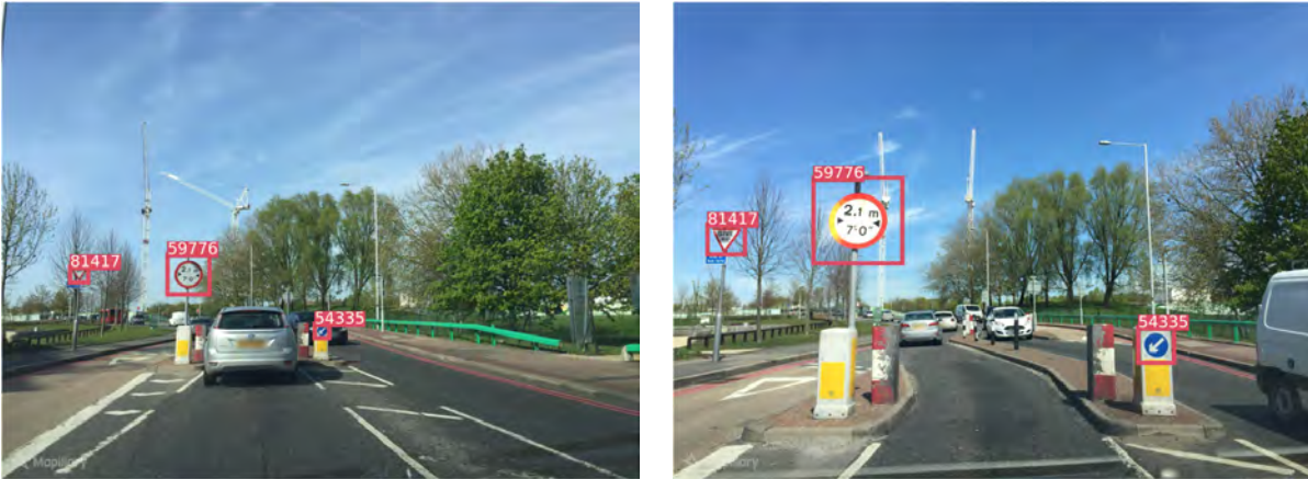
Figure 5.5: Subset of the Mapillary dataset. This scene depicts a dashcam sequence where nearly all signs in the scene are annotated with their instance label (red), and shows strong object scale changes across the different views.
