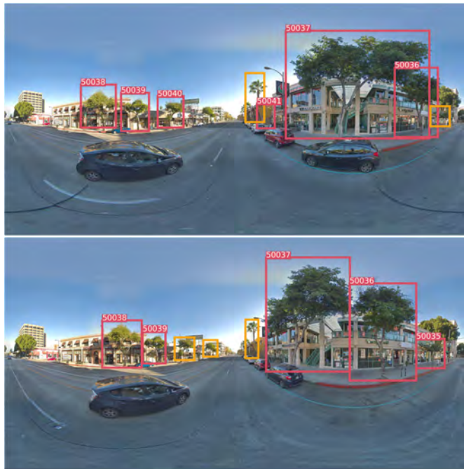
Figure 5.4: Subset of the Pasadena dataset highlighting challenges to be faced by multi-view object detection, re-identification and geo-localization. The trees are in close proximity and share very similar appearances due to their same species and size (trees on the curb are planted together at the same time). Some objects are annotated with their instance label (red), some without (orange). (Imagery ©2021 Google)
