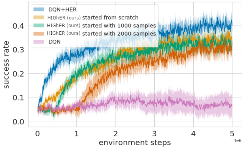
Figure 4.5: The instruction generator is triggered after collecting 0, 1000 and 2000 positive trajectories (i.e, approximately 0%, 20%, 50% accuracy). Even when the instruction generator is not accurate, the policy still makes steady progress and the final success rate is not impacted. Delaying the generator instructor does not provide additional benefit
