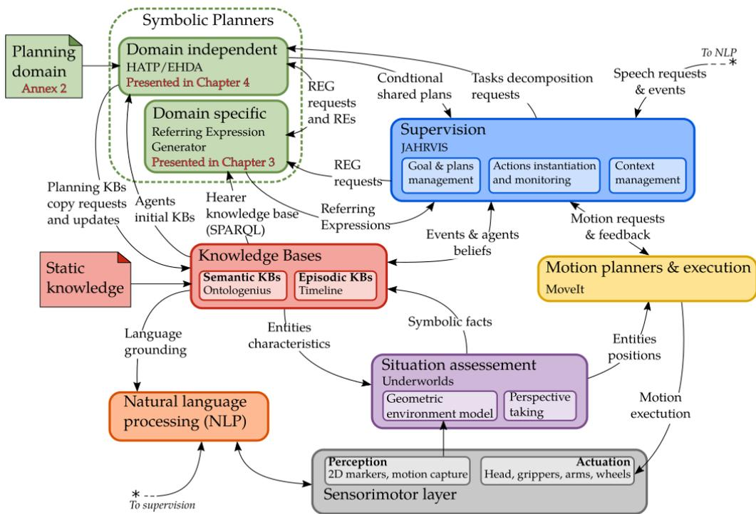
Figure 5.4: The robotic architecture implemented to handle both perspectives of the director task. The components circled with a dashed green line are presented in this thesis.
