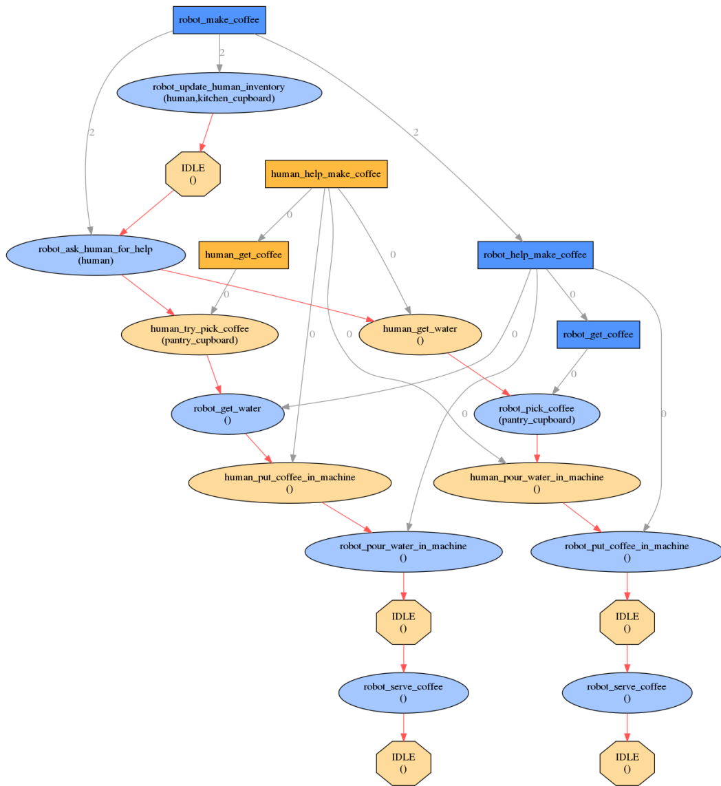
Figure 4.11: A conditional plan returned by the planner to make coffee with human help in case of (known) beliefs divergence. Here, the robot chooses to communicate to realign the beliefs with the human, then asking him for help, preventing any human misleading.
