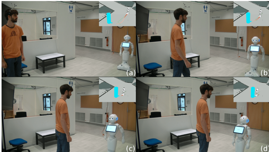
Figure 2.9: The Pepper robot approaching a human. The planner adapts to the human moves. In (a) the planned path is long but decrease in (b) and (c) as the human is actively taking part in the approach task until the robot successfully reaches a position close in front of the human (d).
