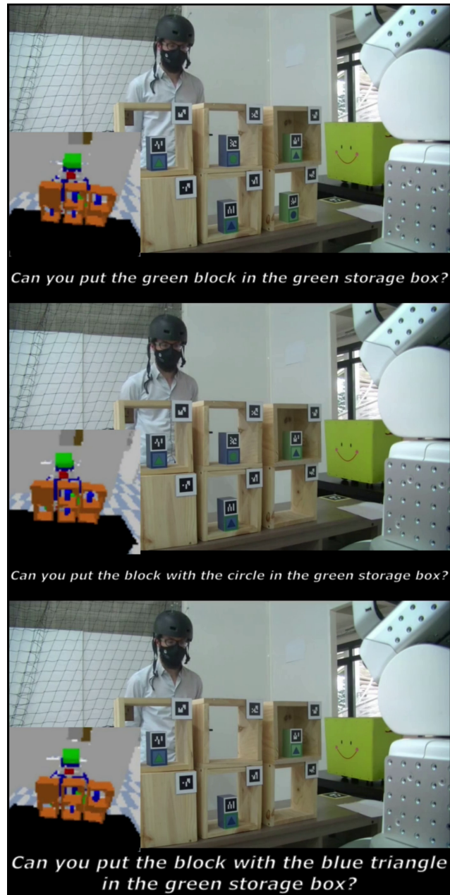
Figure 5.5: The director task handled by an autonomous PR2 robot in the director role. The computed human perspective is displayed in the bottom left hand corner of the picture. The robot said sentence is printed under each picture.
