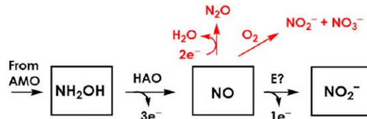
Figure 1.4: Two models for obligate intermediates of NH 3 oxidation to NO 2 - production by AOB (Caranto and Lancaster, 2017)
