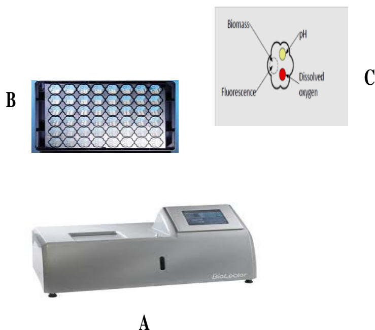
Figure 31 A) Biolector ® fermentation system; B) 48-well MTP; C) Probes inside each well
