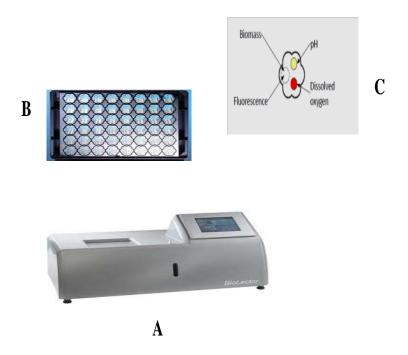
**Figure 31 A)** Biolector<sup>®</sup> fermentation system; **B)** 48-well MTP; **C)** Probes inside each well
