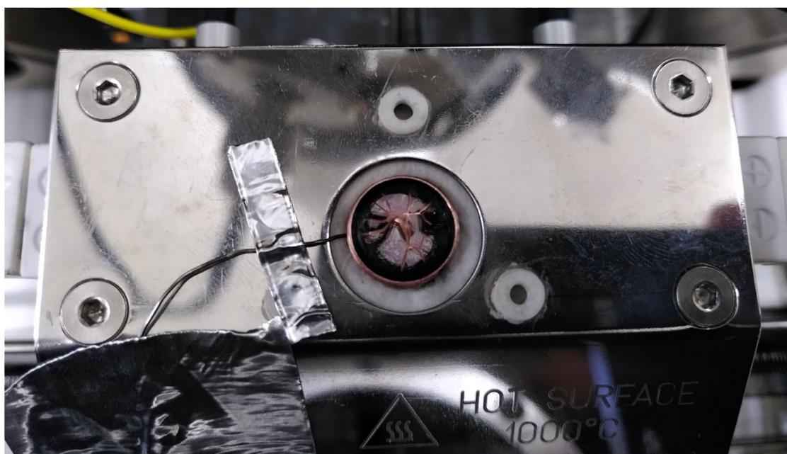
Figure D.7: Sample at the end of the experiment. A black color seems to diffuse from the edges.
