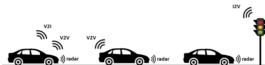
Figure 1.6: Illustration of vehicles forming a CACC string.
