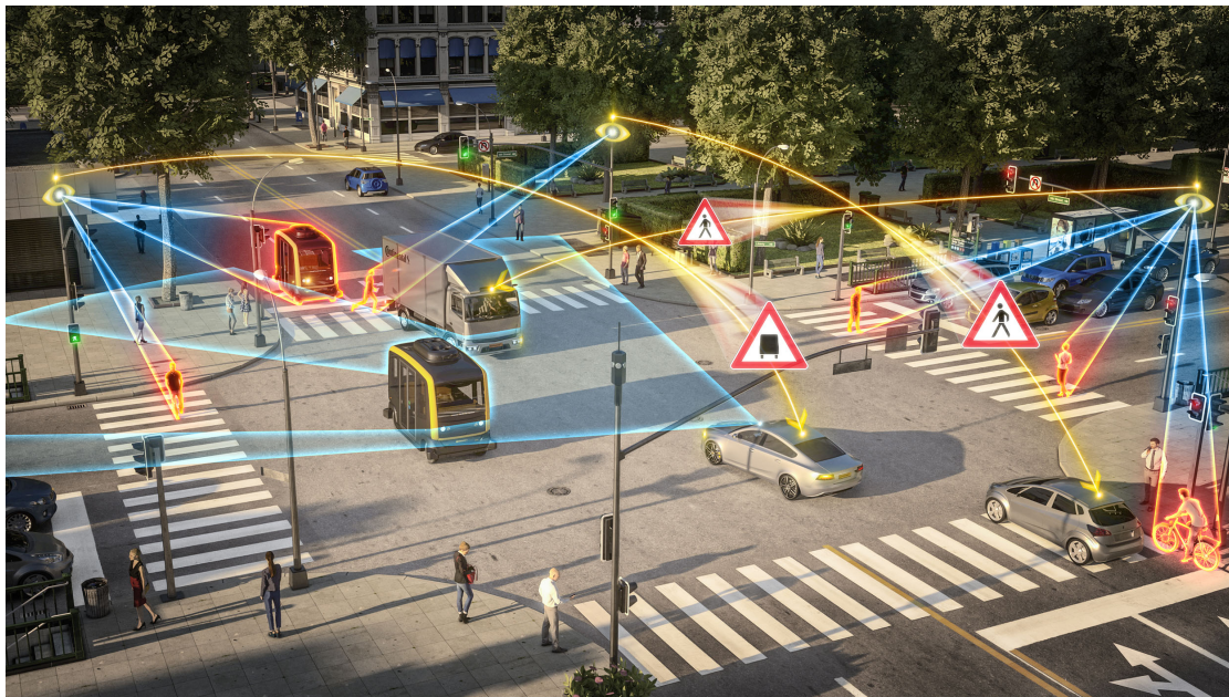
Figure 1.9: Strategy to increase safety by communicating hidden dangers to approaching vehicles and pedestrians at an intersection [45] [©2019 Continental. All rights reserved].
