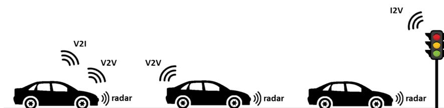
Figure 1.6: Illustration of vehicles forming a CACC string.
