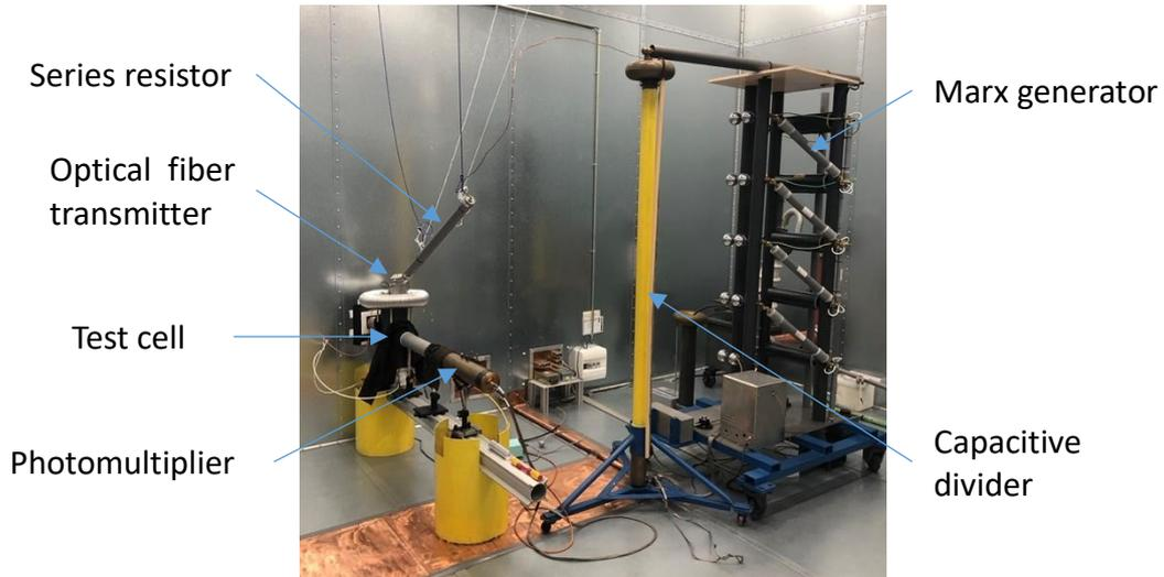
Figure 2. 8 : Photograph of the test system
