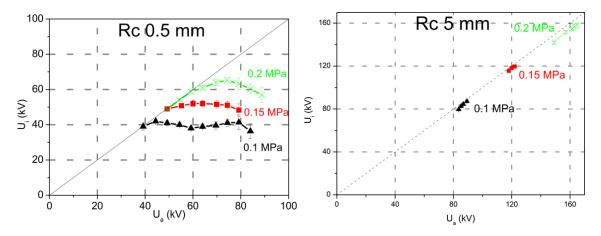
Figure 3. 6: Initiation voltage  $U_i$  as a function of the applied voltage  $U_a$  in a very inhomogeneous field in HFO ( $R_c = 0.5 \text{ mm}$ , d = 50 mm,  $\eta = 84$ )
