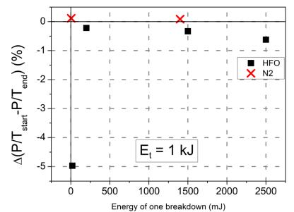
Figure 4. 28: Pressure variation in the HFO as a function of the energy of one breakdown ( $R_c = 5 \text{ mm}$ , d = 10 mm, P = 0.1 MPa)
