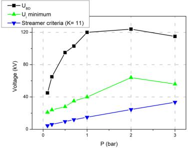
Figure 4. 40 : Streamer criteria for  $SF_6$  ( $R_c = 0.2$  mm, d = 50 mm,  $\eta = 86$ , K = 11)
