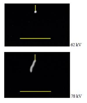
Figure 1. 13: Photographs of pre-breakdown discharges in HFO at voltages lower than the breakdown voltage. ( $R_c = 0.5 \text{ mm}$ , d = 5 cm, P = 0.2 MPa) [7]
