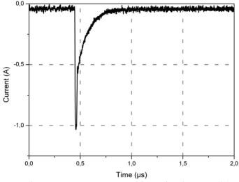
Figure 3. 11 : Current of positive streamer in air  $(R_c = 0.2 \text{ mm}, d = 50 \text{ mm}, P = 0.1 \text{ MPa}, U_a = 36 \text{ kV})$
