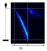
Figure 1. 22 : Image of a streak camera of a positive corona discharge (U = 7.2 kV, d = 7 mm, tipplane configuration, P = 0.1 MPa) [57]
