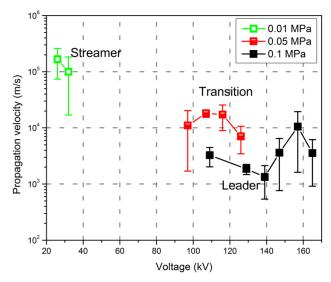
Figure 3. 19: Velocity of propagation in negative polarity in HFO as a function of voltage and pressure ( $R_c = 0.2 \text{ mm}, d = 50 \text{ mm}, \text{ error bar: standard deviation}$ )
