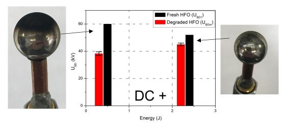
Figure 4. 27: Influence of energy on the stability of breakdowns and powder deposits on electrodes with positive polarity electrodes ( $R_c = 5 \text{ mm}$ , d = 20 mm, P = 0.1 MPa)
