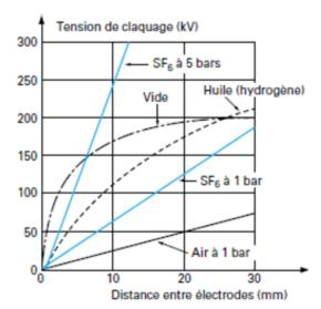
Figure 1.1: Impact of the distance between the electrodes on the breakdown voltage in uniform field [116]
