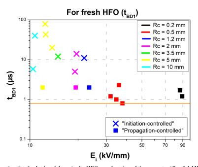
Figure 4. 8 : Delay time for the 1st breakdown in the HFO as a function of the geometry (P = 0.1 MPa). Orange line corresponds to the voltage rise time
