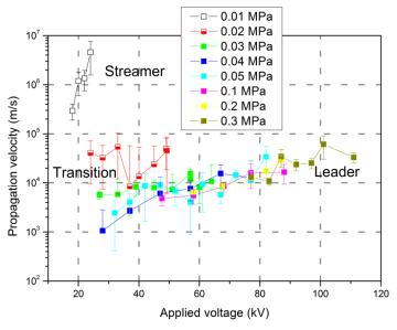
Figure 3. 18: Velocity of propagation in positive polarity in the HFO as a function of voltage and pressure ( $R_c = 0.2 \text{ mm}$ , d = 50 mm, error bar: standard deviation)
