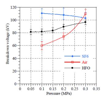
Figure 1. 12: Breakdown voltage versus pressure in point-plane geometry under impulse voltage, in HFO, SF<sub>6</sub> and dry Air. ( $R_c = 0.5$  mm, d = 5 cm) [7]
