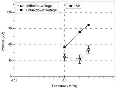
Figure 3. 39 : Difference between initiation and breakdown voltage in positive polarity as a function of pressure for  $air(R_c = 0.2 \text{ mm}, d = 50 \text{ mm}, max/min error bar)$
