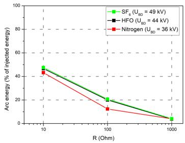
Figure 4. 24: Arc energy as a percentage of the maximum energy stored in capacitor (plan-plan, d = 5 mm)
