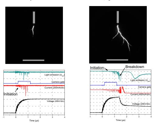
Figure 3. 2 : Leader not leading to breakdown in HFO  $(U_a = 86 \text{ kV}, R_c = 0.2 \text{ mm}, d = 50 \text{ mm}, P = 0.1 \text{ MPa})$
