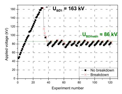
Figure 4. 1 : Up and down measurement series in HFO including 120 shots ( $R_c = 5$  mm, d = 50 mm, P = 0.1 MPa,  $\eta = 7$ )
