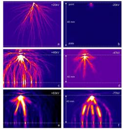
Figure 1. 19: Time-integrated photographs of positive (left column) and negative (right column) streamers in air in a space of 40 mm in air at 0.1 MPa ( $Rc = 15 \mu m$ ) [55]
