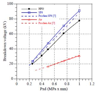
Figure 1. 8: Comparison of breakdown measurements obtained in HFO, SF<sub>6</sub>, and dry Air in the same conditions, versus (Pressure x distance) product. DC ramp 1 kV/s, d = 5 mm, plan-plan. [7]
