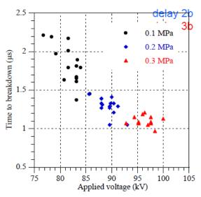
Figure 1. 11: Time to breakdown  $t_b$  versus breakdown voltage  $V_b$  in HFO at different pressure under impulse voltage. (Rc =0.5 mm, d = 5 cm) [7]
