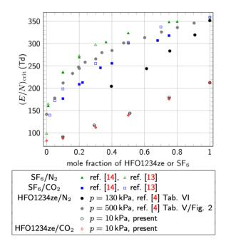
Figure 8: Reduced critical electric field as a function of HFO1234ze or SF<sub>6</sub> mole fraction in N2 or CO<sub>2</sub> [114]
