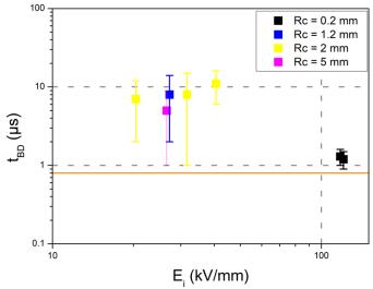
Figure 4. 10: Average delay time to breakdown in the SF<sub>6</sub> as a function of the geometry (P = 0.1 Mpa, max/min error bar). Orange line corresponds to the voltage rise time
