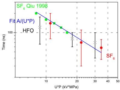
Figure 3. 26: Time between 2 re-illuminations in HFO and SF<sub>6</sub> as a function of the product  $U^*P$  with comparison with the data of Qiu ( $R_c = 0.2$  mm, d = 50 mm and A = 1680) [83]
