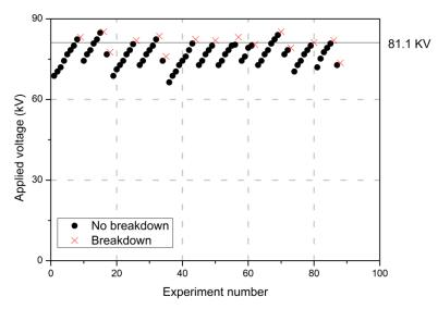
Figure 3. 35 : « Up and down » breakdown measurement for HFO ( $R_c = 0.5$  mm, d = 50 mm, P = 0.1 MPa,  $\eta = 40$ )
