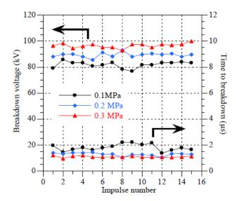
Figure 1. 10: Measurement of breakdown voltage  $V_b$  in point-plane geometry and corresponding time to breakdown  $t_b$  in HFO under impulse voltage. ( $R_c = 0.5 \text{ mm}$ , d = 5 cm) [7]
