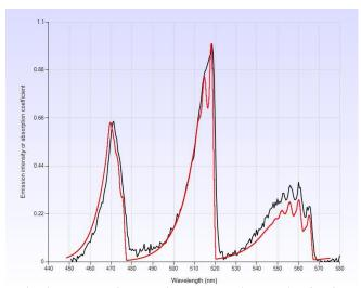
Figure 3. 34: Example of comparison between the spectrum of  $C_2$  simulated with Specair (red) and the one observed experimentally in HFO during the breakdown (black) with ( $T_e = 10000 \text{ k}$ ,  $T_v = 5300 \text{ K}$  and  $T_r = 5000 \text{ K}$ ,  $R_c = 0.2 \text{ mm}$ , d = 50 mm, P = 0.1 MPa,  $U_a = 67 \text{ kV}$ )
