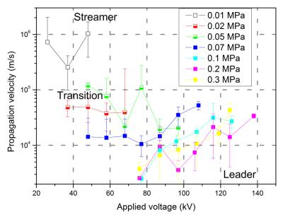
Figure 3. 16: Velocity of propagation in positive polarity in SF<sub>6</sub> as a function of voltage and pressure ( $R_c = 0.2 \text{ mm}$ , d = 50 mm, error bar: standard deviation)
