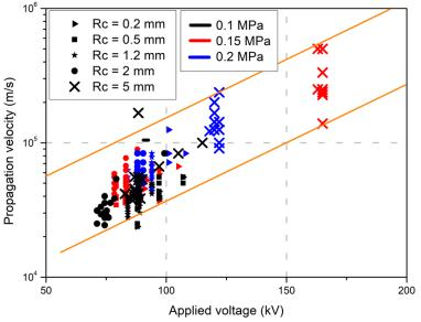
Figure 4. 12 : Propagation velocity as a function of pressure in the degraded HFO for different  $R_c$  and pressure (d = 50 mm)
