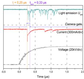
Figure 2. 14: Characteristic measurements of voltage, current, camera signal and light emission
