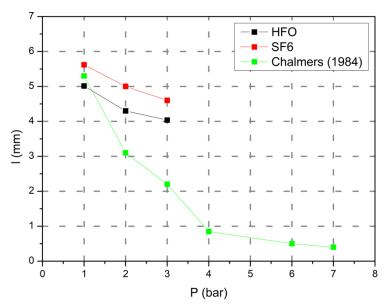
Figure 3. 27: Leader step lengths in SF<sub>6</sub> and HFO as a function of pressure ( $R_c = 0.2$  mm, d = 50 mm) in comparison with the results of Chalmers et al. [79] ( $R_c = 0.05$  mm, d = 30 mm)
