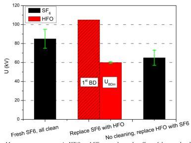
Figure 4. 14: Measurement sequence in HFO and SF<sub>6</sub> to evaluate the effect of the powder deposit on the dielectric strength ( $\eta = 2.5$ , P = 0.1 MPa, up and down method)
