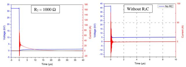
Figure 4. 19: Example of measurement of voltage and breakdown current in the HFO (plane-plane, d = 5 mm, P = 0.1 MPa,  $U_a = 34$  kV,  $R_2 = 1000$   $\Omega$  and without  $R_2C$ )
