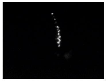
Figure 5 : Image of emitted light 100  $\mu s$  after breakdown in HFO ( $R_c=5$  mm, d=50 mm, P=0.1 MPa,  $U_a=90$  kV)
