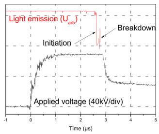
Figure 3. 4: Breakdown in degraded HFO ( $U_a = 73 \text{ kV}$ ,  $R_c = 5 \text{ mm}$ , d = 10 mm, P = 0.1 MPa)
