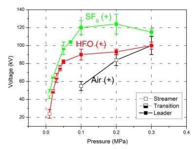
Figure 3. 37: Average of 15 breakdown voltage in air,  $SF_6$  and HFO as a function of the pressure in positive polarity ( $R_c = 0.2$  mm, d = 50 mm, max/min error bar) "up and down" method.
