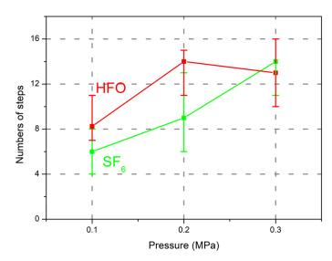
Figure 3. 25 : Total number of leader steps as a function of the pressure in the HFO and SF<sub>6</sub> in positive polarity  $(R_c=0.2\ mm,\ d=50\ mm,\ P=0.1\ MPa,\ max/min\ error\ bar)$
