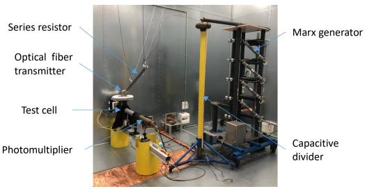
Figure 2. 8 : Photograph of the test system
