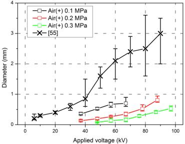
Figure 3. 14: Diameter of streamers in air as a function of voltage for different pressures (Propagation velocity of pre-disruptive phenomena in air as a function of pressure in positive polarity ( $R_c = 0.2 \text{ mm}$ , d = 50 mm, max/min error bar) with the results of [55]
