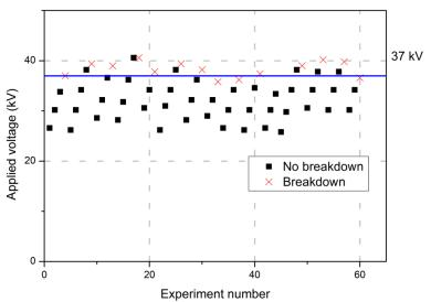
Figure 3. 10: « Up and down » method in HFO for 15 breakdowns (( $R_c = 0.5 \text{ mm}, d = 10 \text{ mm}, P = 0.1 \text{ MPa}$ )
