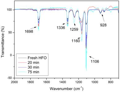
Figure 4. 30: FTIR of HFO gas after 20, 30 and 75 minutes
