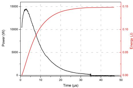
Figure 4. 22 : Arc power and energy in HFO (plane-plane, d = 5 mm, P = 0.1 MPa,  $U_a = 34$  kV,  $R_2 = 1000\Omega$ )
