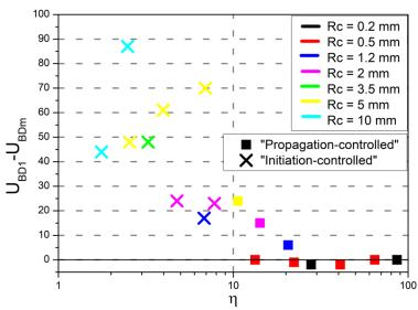
Figure 4. 6 : Difference between the 1<sup>st</sup> breakdown voltage  $U_{BD1}$  and the average breakdown voltage  $U_{BDmean}$  depending on the amplification factor of the field  $\eta$  (P=0.1 MPa)
