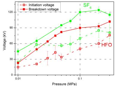
Figure 3. 40: Difference between initiation and breakdown voltage in positive polarity as a function of pressure for HFO and  $SF_6$  ( $R_c = 0.2$  mm, d = 50 mm, max/min error bar)
