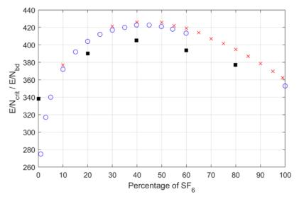
Figure 9: Critical field strength (E/N)crit of mixtures of  $SF_6$  with HFO1234ze(E). In blue circles, a measurement series at pressures of 360-480 Pa is shown. In red crosses, we used higher, variable pressures from 4-12 kPa. In black squares, breakdown results (E/N)bd for the mixture of  $SF_6$  with  $C_3F_6$  is given at pressure of 67 kPa [115].
