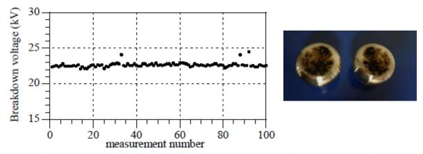
Figure 1. 9: Evolution of breakdown voltage of HFO subjected to repeated breakdown measurements under DC ramp. P = 0.1 MPa, d = 3 mm [7]
