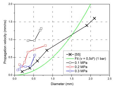
Figure 3. 15: Propagation velocity of streamers as a function of diameter and air pressure ( $R_c = 0.2 \text{ mm}$ , d = 50 mm, max/min error bar) with the results of [55]
