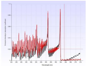
Figure 3. 33: Example of comparison between the spectrum of  $C_2$  simulated with Specair (red) and the one observed experimentally in HFO during the breakdown (black) with  $(T_v = T_r = 5000 \text{ K}, R_c = 0.2 \text{ mm}, d = 50 \text{ mm}, P = 0.1 \text{ MPa}, U_a = 86 \text{ kV})$
