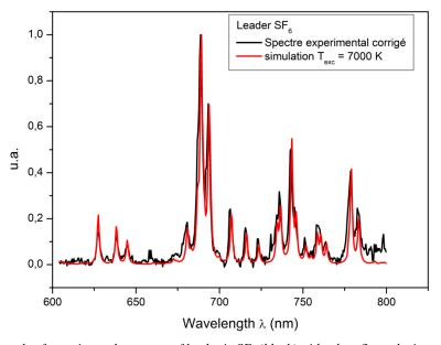
Figure 3. 31: Example of experimental spectrum of leader in SF<sub>6</sub> (black) with a best fit synthetic spectrum of FI line (red). The experimental spectrum is corrected for the wavelength depending on sensitivity of the spectrometer  $(R_c = 0.2 \text{ mm}, d = 50 \text{ mm}, P = 0.1 \text{ MPa})$
