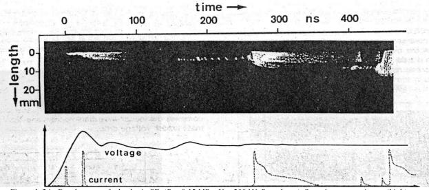
Figure 1. 24: Development of a leader in SF<sub>6</sub> (P = 0.15 MPa, U = 200 kV, Rc = 1 mm). Scanning camera image (high), applied voltage and current associated with leader steps (low) [66].
