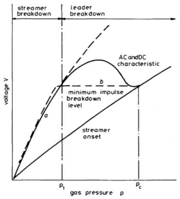
Figure 3. 41: Idealised V/P characteristic for a point-plane gap in SF<sub>6</sub>[79]
