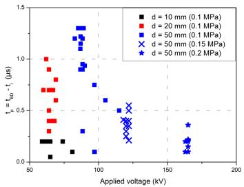
Figure 4. 11: Propagation time as a function of voltage, and pressure in the degraded HFO ( $R_c = 5$  mm, d = 50 mm)
