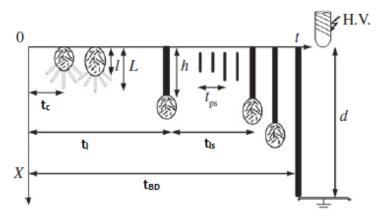
Figure 1. 25: Schematic diagram of leader development.  $t_c$ , time of formation of the first corona;  $t_l$ , leader training time;  $t_{PS}$ , progression time of the precursor;  $t_{lS}$ , leader training time;  $t_{BD}$ , breakdown time. Adapted from [121].
