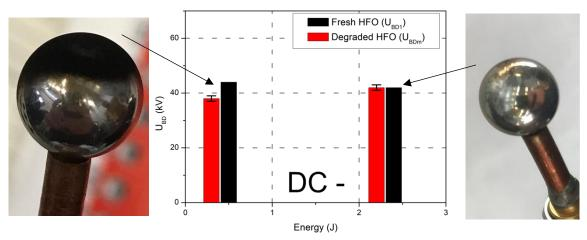
Figure 4. 26: Influence of energy on the stability of breakdowns and powder deposits on electrodes with negative polarity ( $R_c = 5 \text{ mm}$ , d = 20 mm, P = 0.1 MPa)
