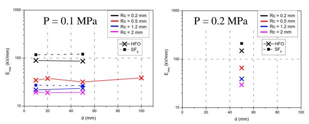
Figure 3. 44: Value of the initiation field  $E_i$  as a function of the distance when the breakdown is controlled by propagation (P = 0.1 and 0.2 MPa)
