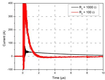
Figure 4. 20 : Arc current for different resistances  $R_2 = 1000$  and  $100 \Omega$  ( $U_{BD} = 44 \text{ kV}$ )
