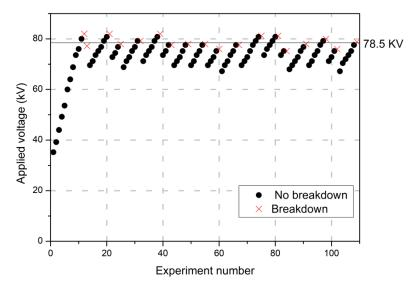
Figure 3. 36: « Up and down » breakdown measurement for HFO ( $R_c = 1.2$  mm, d = 50 mm, P = 0.1 MPa,  $\eta = 21$ )
