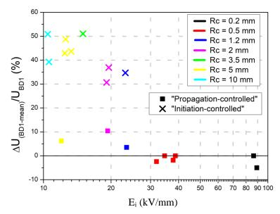
Figure 4. 7: Maximum initiation field at the electrode as a function of the difference between  $U_{BD1}$  and  $U_{BDm}$  (P=0.1~MPa)
