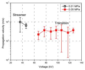
Figure 3. 17: Velocity of propagation in negative polarity in  $SF_6$  as a function of voltage and pressure  $(R_c = 0.2 \text{ mm}, d = 50 \text{ mm}, error bar: standard deviation})$
