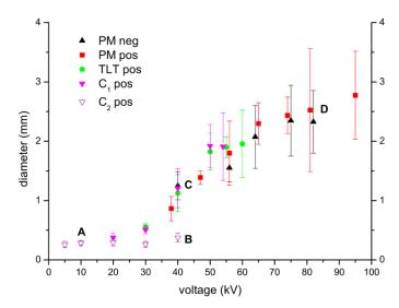
Figure 1. 20: Diameters of positive and negative streamers in air according to the applied voltage (P=0.1 MPa,  $R_c=15$   $\mu$ m and d=40 mm) [55]
