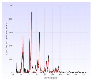
Figure 3. 30: Example of comparison between second positive nitrogen system simulated by Specair (red) and measured experimentally (black) in air during the streamer discharge ( $R_c = 0.2$  mm, d = 50 mm, P = 0.1 MPa) spectrum corrected ( $T_v = 5000$  K,  $T_r = 500$  K)
