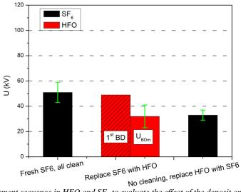
Figure 4. 15 : Measurement sequence in HFO and SF<sub>6</sub> to evaluate the effect of the deposit on the dielectric strength of the HFO ( $\eta = 9$ , P = 0.1 MPa, up and down method)
