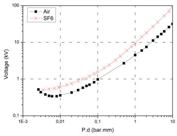
Figure 1. 15: Paschen curve for air and  $SF_6$  at  $20^{\circ}C$  in logarithmic scales from [120]
