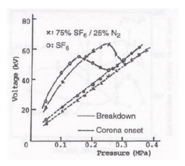
Figure 1. 27: Voltage versus pressure characteristic of SF<sub>6</sub> and a 75% SF<sub>6</sub>-25%  $N_2$  mixture for a point-plane gap and lighting impulse (1.2/50  $\mu$ s) [122]
