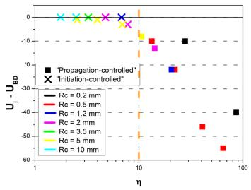
Figure 3. 8: Difference between the initiation voltage and the breakdown voltage as a function of the field strengthening factor ( $\eta = \frac{E_{max}}{E_{mov}}$ , P = 0.1 MPa).
