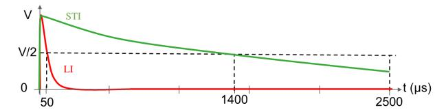
Figure 2. 10: Characteristic parameters of a pulse wave
