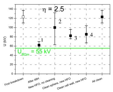
Figure 4. 13: Various tests to understand the origin of the loss of dielectric strength after the  $1^{st}$  breakdown  $(R_c = 5 \text{ mm}, d = 10 \text{ mm}, P = 0.1 \text{ MPa})$
