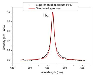
Figure 3. 32: Example of experimental spectrum of breakdown in HFO (black) with a best fit synthetic spectrum of  $H\alpha$  line (red). The experimental spectrum is corrected for the wavelength depending sensitivity of the spectrometer  $(R_c = 0.2 \text{ mm}, d = 50 \text{ mm}, P = 0.1 \text{ MPa})$
