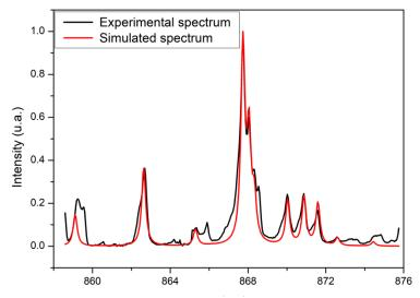
Figure 2: Experimental spectrum and simulated spectrum of N I for breakdown in air  $(R_c = 0.2 \text{ mm}, d = 50 \text{ mm}, P = 0.1 \text{ MPa})$  corrected spectrum
