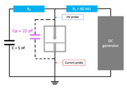
Figure 2. 7: Schematic representation of the configuration used for the DC breakdown measurements
