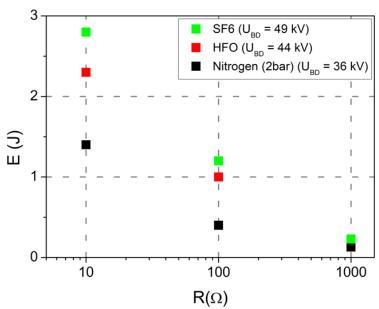
Figure 4. 23: Variation of the energy dissipated in the arc as a function of the series resistance and the gas (plan-plan, d = 5 mm)
