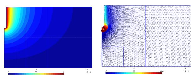
Figure 2. 3 : Electrical potential obtained ( $R_c = 0.5 \text{ mm}$  and d = 50 mm)
