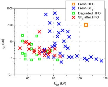
Figure 4. 17 : Delay to breakdown in HFO and SF<sub>6</sub> before and after degradation (P = 0.1 MPa,  $\eta = 2.5$ )
