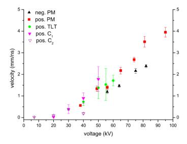
Figure 1. 18: Velocity of positive and negative streamers in air at atmospheric temperature and pressure as a function of the voltage (gap = 4 cm, Rc =  $15 \mu m$ ) [55]
