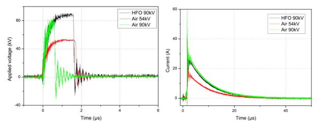
Figure 3: Current of arc and applied voltage in air and HFO (STI,  $R_c = 5$  mm, d = 50 mm, P = 0.1 MPa)
