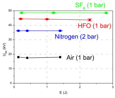
Figure 4. 25: Average DC breakdown voltage in nitrogen, air, SF<sub>6</sub> and HFO in a homogeneous field as a function of energy (d = 5 mm, plane-plane, DC)
