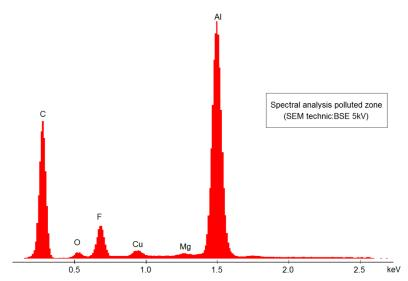
Figure 4. 33: EDX-Spectral analysis of the dusty layer on electrodes after breakdown tests in HFO-1234ze(E) [102]
