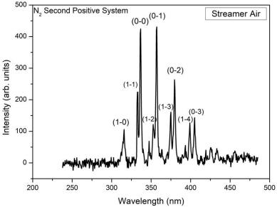
Figure 3. 29: A typical emission spectrum from streamer in air exhibiting  $N_2$  ( $C_3\Pi$ - $B_3\Pi$ ) with assigned vibrational quantum numbers v'-v' ( $R_c = 0.2$  mm, d = 50 mm, P = 0.1 MPa) spectrum not corrected
