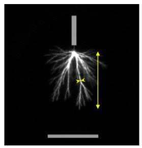
Figure 2. 15: Image of a streamer being propagated in the air (Rc = 0.5 mm and d = 50 mm) allowing to measure the length of propagation lp
