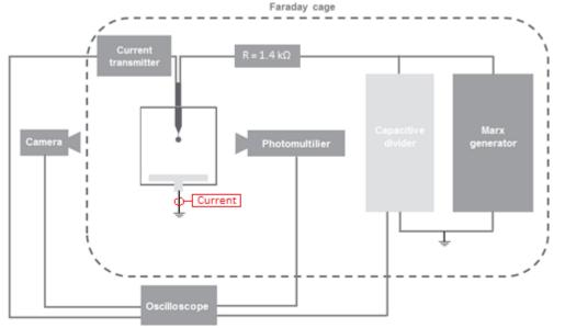
Figure 2. 9 : Schematic representation of the configuration used for the impulse breakdown measurements
