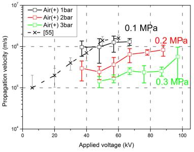
Figure 3. 12: Velocity of positive streamers in air as a function of voltage and pressure  $(R_c = 0.2 \text{ mm}, d = 50 \text{ mm}, error bar: standard deviation})$  with the results of [55]
