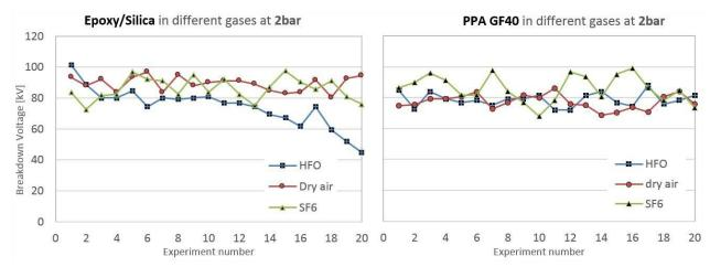
Figure 10: Breakdown voltages solid/gas insulation with PPA and Epoxy with SF<sub>6</sub>, dry air and HFO1234zeE [7]
