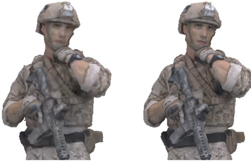
Fig. V-5. The decoded frame of soldier using V-PCC in R01 condition (left). The estimated frame of soldier using the proposed method with equivalent encoding cost (right).
