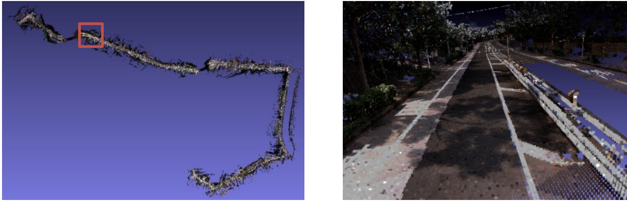
City tunnel (R. Cohen, H. Ochimizu, D. Tian, 2017): entire scene (left) with around 19 M points and a local zoom (right)
