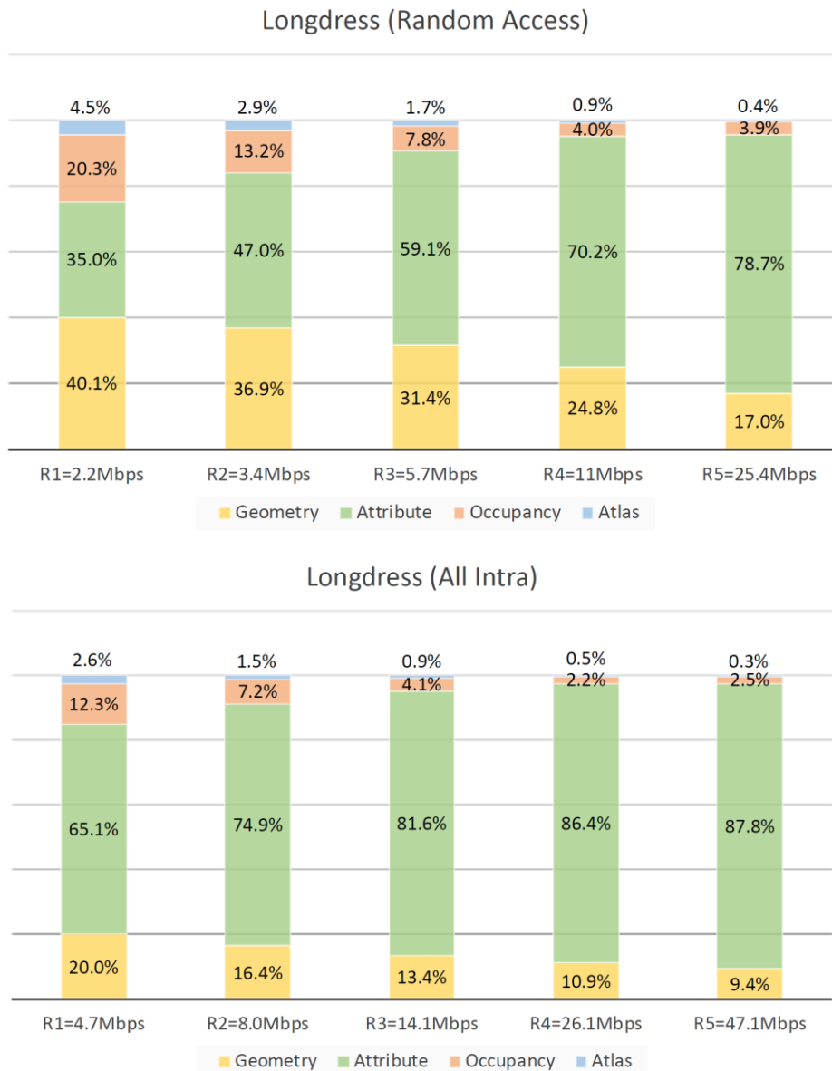
Fig. III-6. The composition of the bitstream components for the longdress sequence (the other sequences have similar distribution).
