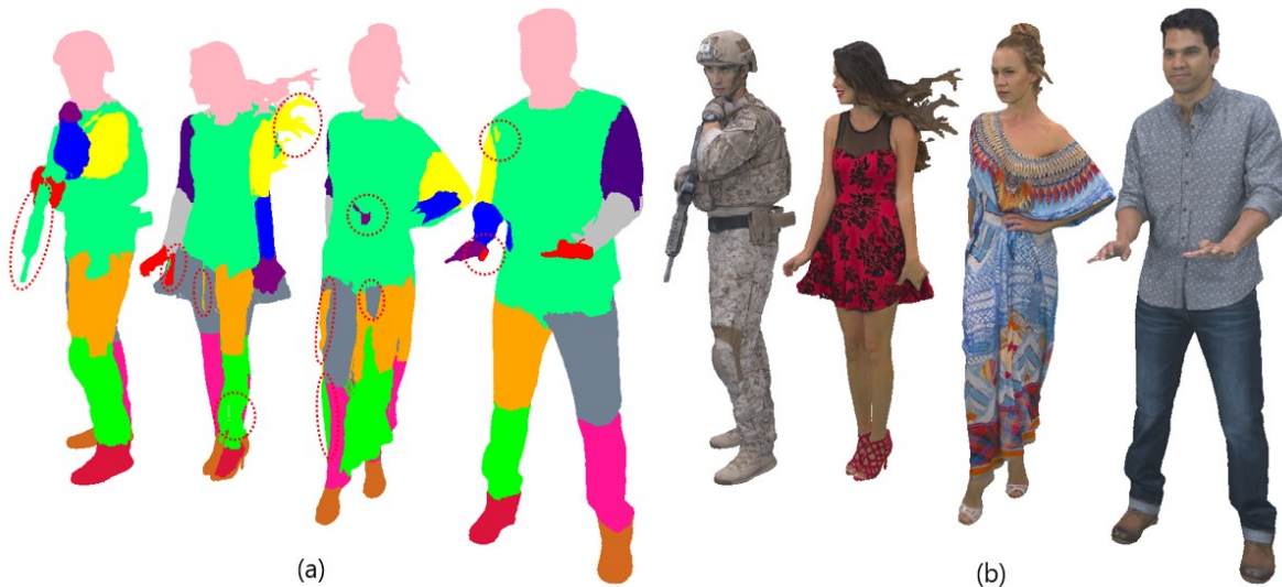
Fig. V-12. (a) The generated 3D body parts of the tested sequences (the segments with incorrect labels are circled, from left to right: soldier, redandblack, longdress, and loot). (b) the original point clouds.
