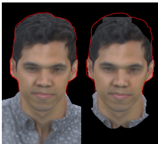
Fig. VI-3. The input image (left) to DensePose of the face part from loot and the segmented output image (right) from DensePose. (Red lines represent the contour of the head)
