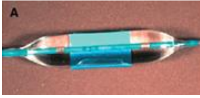
Figure 3.1: Bench test showing the different profiles between a non-compliant balloon (A) and a semi-compliant balloon (B) during high-pressure inflation. The blue central cylinder represents the balloon-plaque contact region. A “dog bone” effect can be observed in the semi-compliant balloon case. (A) and (B) were reproduced from [169].
