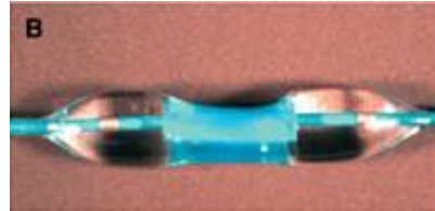
Figure 3.1: Bench test showing the different profiles between a non-compliant balloon (A) and a semi-compliant balloon (B) during high-pressure inflation. The blue central cylinder represents the balloon-plaque contact region. A “dog bone” effect can be observed in the semi-compliant balloon case. (A) and (B) were reproduced from [169].
