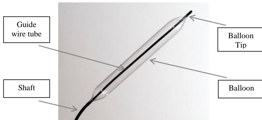
Figure 1.2: A standard high-pressure inflated PTA balloon [healthmanagement.org].
