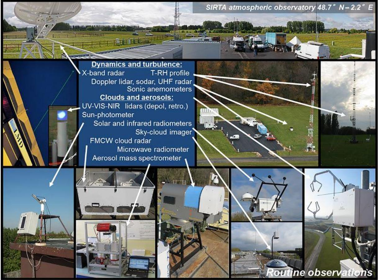
**Figure 2-2:** Photos of some of the instruments installed in the SIRTA observatory. This figure is extracted from Chiriaco et al., (2018).
