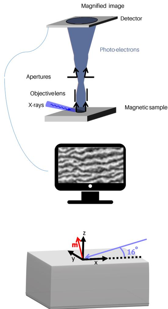
Figure 5.2: **X-ray photo-emission electron microscope.** The X-ray beam impinges the sample at a grazing angle of  $16^\circ$  on the sample surface as shown in the bottom image. The emitted photo-electrons are processed by the different electron-optic components before reaching an electron-sensitive screen.
