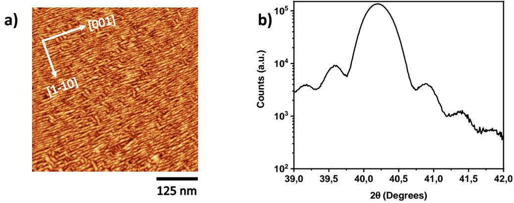
Figure 4.3: **Morphology of as-deposited tungsten studied with scanning tunneling microscopy and after annealing with x-ray diffraction** a) Tungsten morphology as-deposited with scanning tunneling microscopy. Two types of grooves orientation are observed. The majority is along the W-[001] b) x-ray diffraction in the  $\theta - 2\theta$  geometry of a bcc-W film grown at 373 K and annealed at 1073 K. The W(110) peak is located at  $\theta = 40.1^\circ$ , with Kissing fringes.
