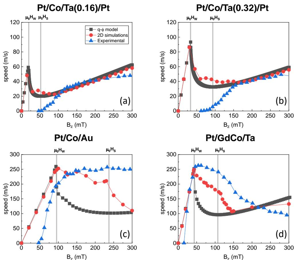
Figure 3.7: **Experimental domain wall speed driven by an out-of-plane magnetic field.** Blue dots represent the experimental speeds, the red dots the micromagnetic simulations, and the black dots, the 1D model. The vertical gray lines represent the exact values of the Walker and Slonczewski field,  $\mu_0 H_W$  and  $\mu_0 H_S$  respectively. **a)** Pt/Ta(0.16nm)/Co(0.8nm)/Pt; **b)** Pt/Ta(0.32nm)/Co(0.8nm)/Pt; **c)** Au/Co(0.8nm)/Pt; **d)** Ta/GdCo(4nm)/Pt.
