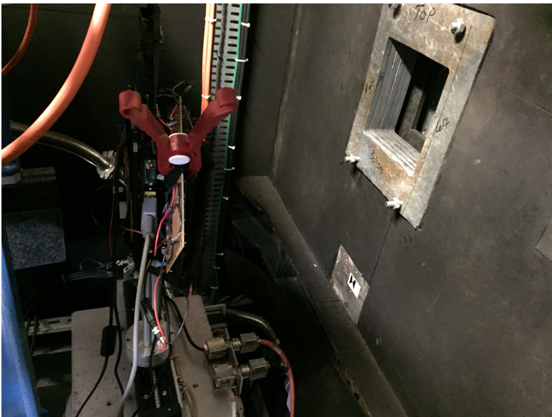
Figure 4.3: FPGA board installed at the D50 thermal neutron accelerator facility
