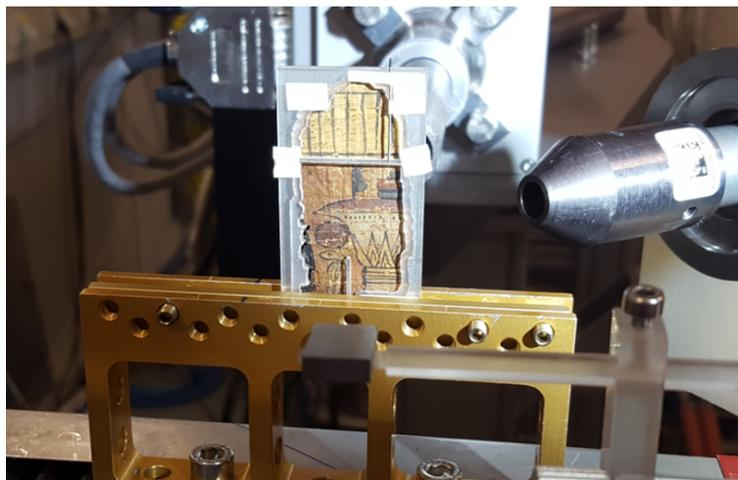
Figure 3.7: Experimental setup on ID22 beamline with papyrus fragment PAP-12 mounted on the 3D printed support.
