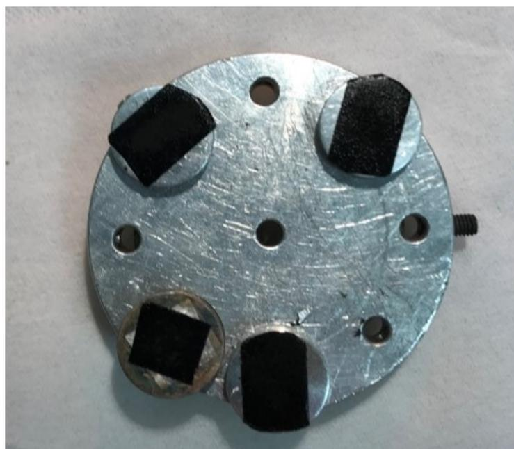
Figure 1.20: Sample stage with four samples put on carbon tape. These pieces of carbon tape were not carefully cut to be easily identifiable.
