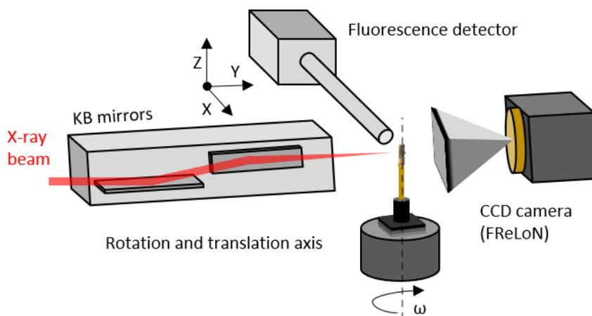
Figure 1.10: XRD-CT experimental setup on the ID11 beamline
