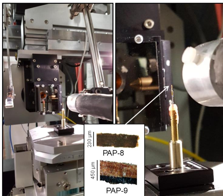
Figure 3.59: XRD-CT experimental setup on ID11 with PAP-8 and PAP-9.
