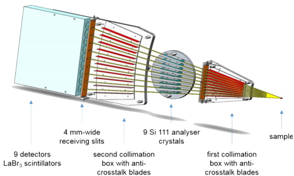
Figure 1.6: Schematic representation of ID22 beamline multi-analyser stage.
