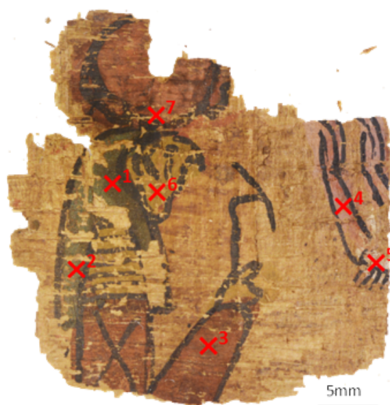
Figure 3.18: XRD measurement point locations on papyrus fragment PAP-6
