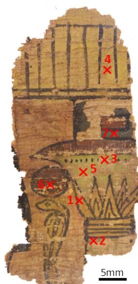
Figure 3.34: Location of the XRPD measurement points made on fragment PAP-12.
