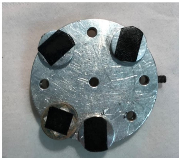
Figure 1.20: Sample stage with four samples put on carbon tape. These pieces of carbon tape were not carefully cut to be easily identifiable.
