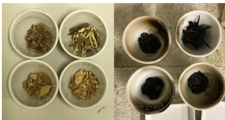
Figure 1.15: Vegetables before and after carbonization: hazelnut shells (top-left), vine branches (top-right), almond shells (bottom-left), and walnut shells (bottom-right).
