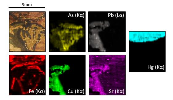
Figure 3.25: XRF maps of major elements, each map represents the ROI around the main emission line (i.e.  $K\alpha$  or  $L\alpha$ ) (mercury (Hg) map is displayed on a log scale).
