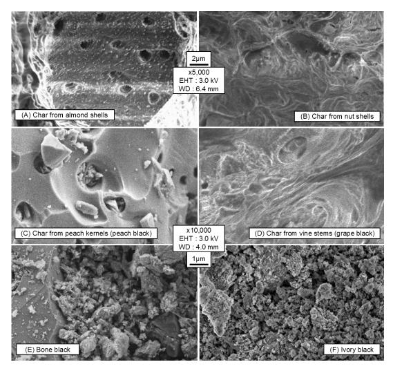
Figure 3.53: SEM observation of six carbon pigment references.
