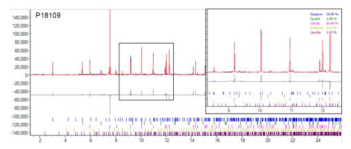
Figure 2.12: Rietveld refinement of P18109 HR-XRPD pattern. (Red = Fit, Blue = Observed, Rwp = 15.2, Rexp = 3.10, Rp = 11.0)
