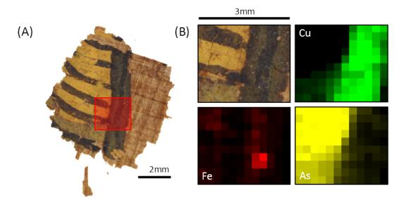
Figure 3.33: (A) PAP-11 fluorescence mapping acquisition. (B) Fluorescence maps of copper  $K\alpha$  (Cu), iron  $K\alpha$  (Fe) and arsenic  $K\alpha$  (As).
