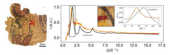
Figure 3.56: XRPD patterns taken on ink and ink-free areas superposed with lampblack diffraction pattern.
