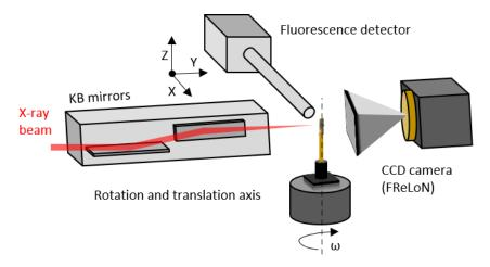
Figure 1.10: XRD-CT experimental setup on the ID11 beamline
