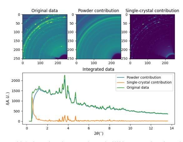
Figure 2.9: Single-crystal contribution removal on sample P9505 from Pompeii. The single-crystal contribution comes mostly from leucite, quartz and orthoclase.
