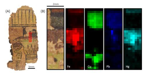
Figure 3.40: (A) PAP-12 fluorescence mapping acquisition (Map 2 (Table 3.6), 28x8 points of 250 $\mu$ m) in the column area. (B) Measured area with fluorescence maps of iron K $\alpha$  (Fe), copper K $\alpha$  (Cu), lead L $\alpha$  (Pb) and mercury L $\alpha$  (Hg).
