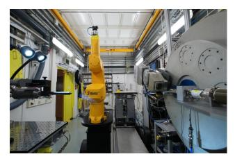
Figure 1.4: ID22 Robot setup with a cryostream (left)
