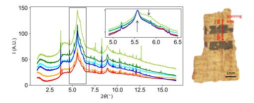
Figure 3.15: XRD signal of six measurement points recorded on black papyrus from fragment PAP-1. Insert: 200 reflection of cellulose. The two arrows indicate the presence of the two contributions. Data have been normalized on the diffraction peak at 5.51°.
