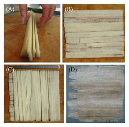
Figure 3.3: Papyrus paper manufacturing steps (Le papyrus comme support d'écriture, E. Menei [66]). (A) Stem cut into strips, (B) First layer of strips, (C) Strips laid down on top with 90 degrees angle, (D) Final product after pressing and drying.
