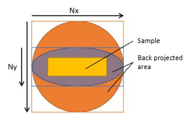
Figure 3.60: Optimisation of acquisition time in XRD-CT. The classic acquisition has Nx=Ny, in this case, Ny < Nx to match the sample shape. The reconstructed area is now an ellipse instead of a circle.
