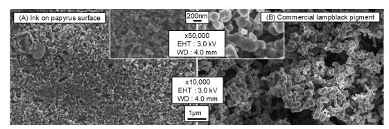
Figure 3.52: SEM observations of (A) Ink at the surface of PAP-1, (B) Kremer pigmente lampblack pigment.
