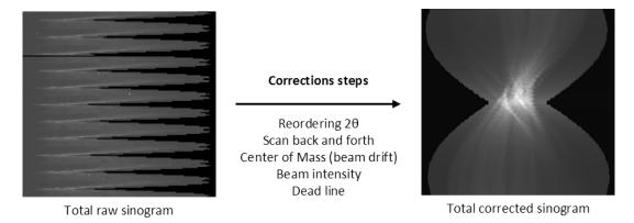
Figure 3.61: Starting point sinogram and corrected sinogram with correction steps. (see subsubsection 3.4.5)
