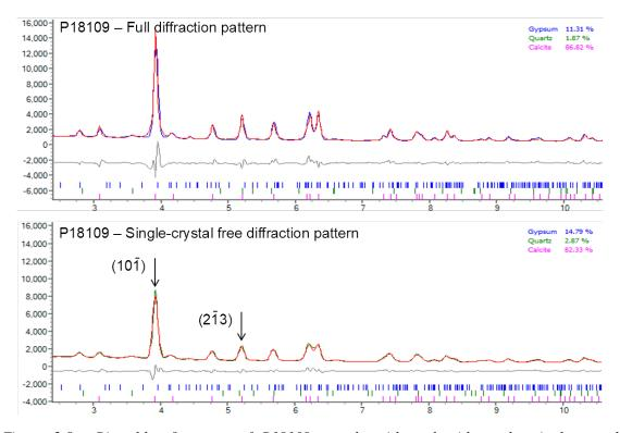
Figure 2.8: Rietveld refinements of P18109 sample with and without the single-crystal contribution (ID22–60keV, Red = Fit, Blue/Green = Observed, Rwp = 6.1 and 5.62 respectively)
