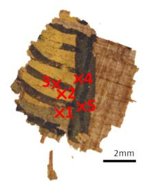
Figure 3.30: Location of the XRD measurement points made on papyrus fragment PAP-11.
