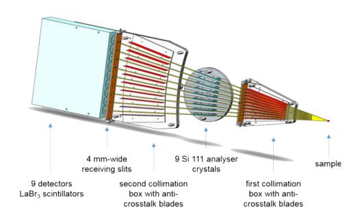
Figure 1.6: Schematic representation of ID22 beamline multi-analyzer stage.
