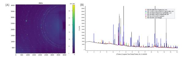
Figure 3.19: (A) 2D diffraction pattern of sample PAP-6 on measurement point 1. (B) 1D diffraction pattern of papyrus PAP-6 on measurement point 1. Weddellite, whewellite and cellulose are present but not shown in the phase identification.
