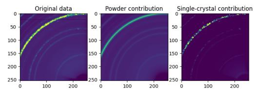
Figure 2.5: Separation of single-crystal and powder contribution from a 2D diffraction pattern portion of sample P18109.
