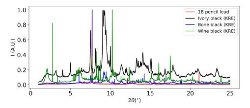
Figure 1.16: HR-XRPD diffraction patterns from ID22 beamline of the reference containing mostly crystalline phases. (KRE = Kremer pigmente)
