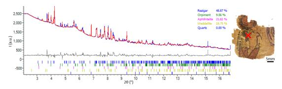
Figure 3.21: Rietveld refinement of measurement point 6 of fragment PAP-6. (Red = Fit, Blue = Observed, Rwp = 2.58, Rexp = 2.85, Rp = 1.56)
