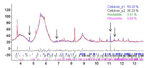
Figure 3.14: Rietveld refinement of a powder diffraction pattern recorded on the papyrus support of PAP-1 ( $\lambda$ = 0.4009Å). The  $I_{\beta}$  structural model was used for both Cellulose\_p1 and Cellulose\_p2 (Blue: experimental data, Red: calculated pattern, Grey: difference curve, Rwp = 5.13). Black arrows indicate non-indexed diffraction peaks.
