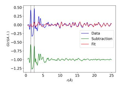
Figure 2.15: PDF fit of sample P2445 (only one crystalline phase (whitlockite) is considered), the data was fit with an r value superior to 15 Å, then it was applied to the whole range (Rw = 0.82). The green curve represents the subtraction of the blue from the red. The two black dotted lines correspond to the two first carbon-carbon bond distances of a graphite layer (1.42 Å and 2.42 Å)
