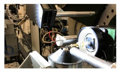
Figure 1.23: HR-XRPD setup with hot air blower for the in-situ experiment on ID22.
