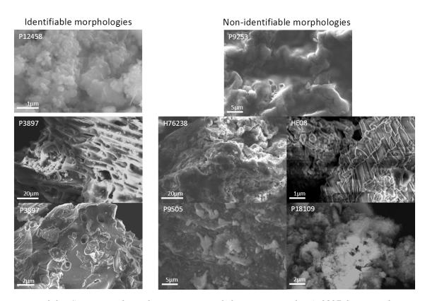
Figure 2.3: SEM secondary electrons image of the seven samples (P3897 has two distinct morphologies) (20kV, WD=7.4mm)
