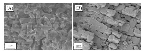
Figure 3.48: Scanning electron microscopy images in SE2 mode. (A) Papyrus fragment PAP-10 surface on white pigment area. (B) Image of a KPb<sub>2</sub>Cl5 crystals
