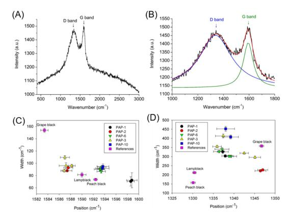
Figure 3.51: (A) Raman spectrum recorded on the black scepter, of god Re from papyrus fragment PAP-6 (B) Fit of the D and G Raman bands of carbon using a 2-band model, (C) Width as a function of position for the G band, (D) Width as a function of position for the D band.
