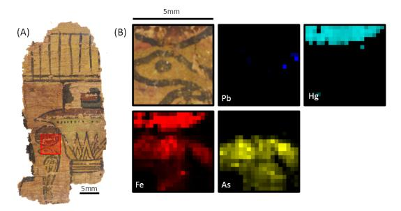
Figure 3.39: (A) PAP-12 fluorescence mapping acquisition (Map 1 (Table 3.6), 20x20 points of 250 $\mu$ m) on the cobra area.(B) Measured area with fluorescence maps of lead L $\beta$  (Pb), iron K $\alpha$  (Fe), arsenic K $\alpha$  (As), and mercury L $\alpha$  (Hg)
