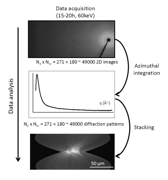
Figure 1.11: Data analysis pipeline for an XRD-CT experiment. The numbers are based on a sample size of  $100x400\mu m$  size with a beam size of  $2x2\mu m$
