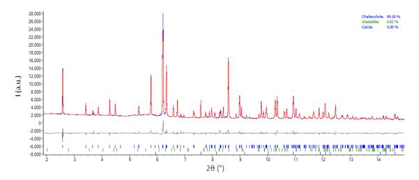
Figure 3.23: Rietveld refinement of point 5 of PAP-6. Calcite was added using pattern matching refinement to fit the peak at 7.6°, coming from single-crystal diffraction behavior. Cellulose contribution was part of the background (Red = Fit, Blue = Observed, Rwp = 5.99, Rexp = 2.34, Rp = 3.95).
