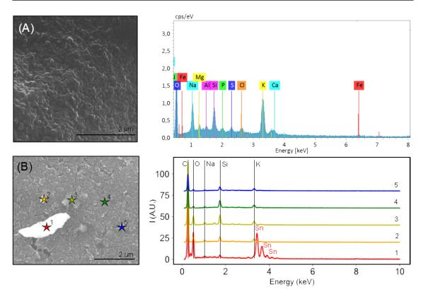
Figure 3.54: (A) EDX spectra recorded on a map at the surface of PAP-1, with corresponding SEM secondary electrons image (20kV, WD=8.2mm) (B) EDX spectra recorded at five different positions at the surface of PAP-1, with corresponding SEM backscattering image (20kV, WD=8.2mm) in the insert. A Sn cluster was identified.
