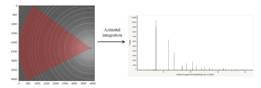
Figure 1.8: Example of the azimuthal integration of a 2D diffraction pattern (Silicon)
