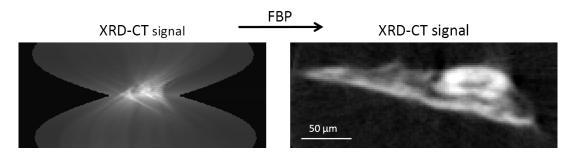
Figure 1.12: Reconstruction of XRD-CT signal using the filtered back-projection algorithm (FBP)
