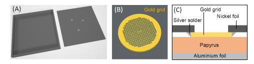
Figure 3.8: Design steps of papyrus sample holder for SEM observation and EDX. (A) Aluminium holder (left), drilled nickel sheet with three holes covered with the gold grids (right), (B) Gold grid laid on the nickel sheet. (C) Cut view of the superposition of all the elements of the support.
