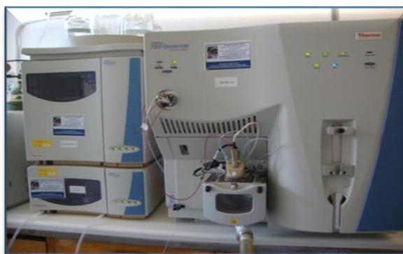
Figure 38: Finnigan Surveyor LC system.
