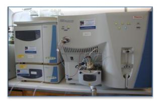
Figure 38: Finnigan Surveyor LC system.
