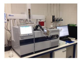
Figure 46: Bruker 456 GC-Scion TQ MS/MS, PAL SPME Autosampler.
