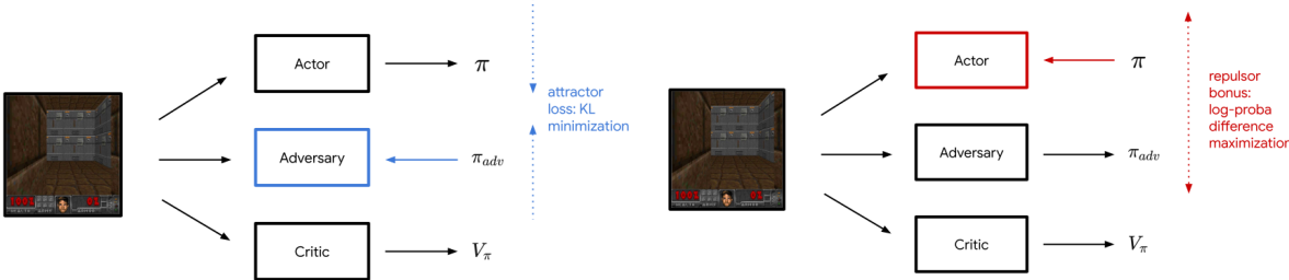
Figure D.4 – A simple schematic illustration of AGAC. Left: the adversary minimizes the KL-divergence with respect to the action probability distribution of the actor. Right: the actor receives a bonus when counteracting the predictions of the adversary.
