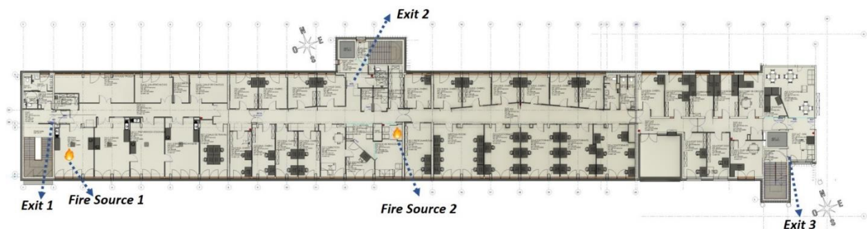
Figure 3.9: LGCgE plan view – fire simulations input
