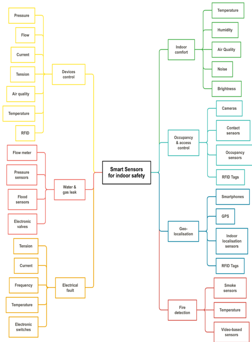
Figure 2.12: Sensors used for indoor hazard management
