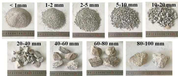
**Figure III .1:** Shuang-Jiang-Kou rock aggregates in different size fractions
