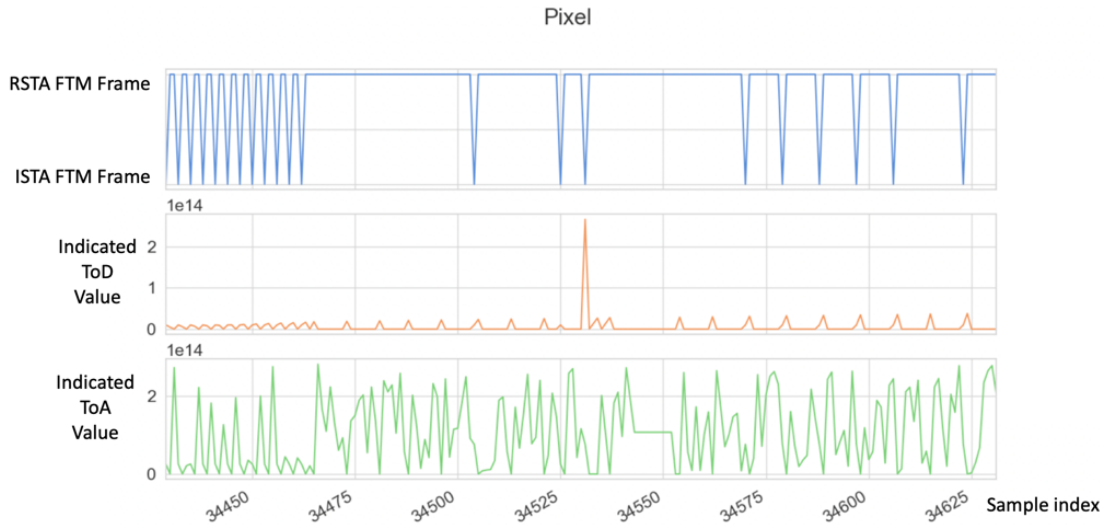
Figure 6.6 – FTM frames for client Pixel. Top figure shows the ISTA request and RSTA responses, the second figure shows the t_1 and the lower figure shows the t_4 values.
