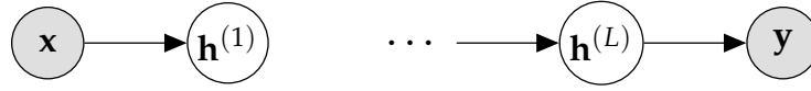
Figure 36: A hidden variable probabilistic model, where the observed variables are the data \mathbf{x} and target \mathbf{y} , with L hidden stochastic layers \mathbf{h}^{(1:L)} .
