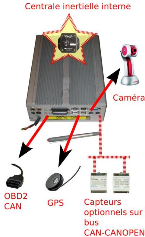
**Figure III.1: DIRCO data logger**
