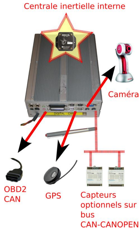
Figure III.1: DIRCO data logger
