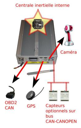
Figure III.1: DIRCO data logger
