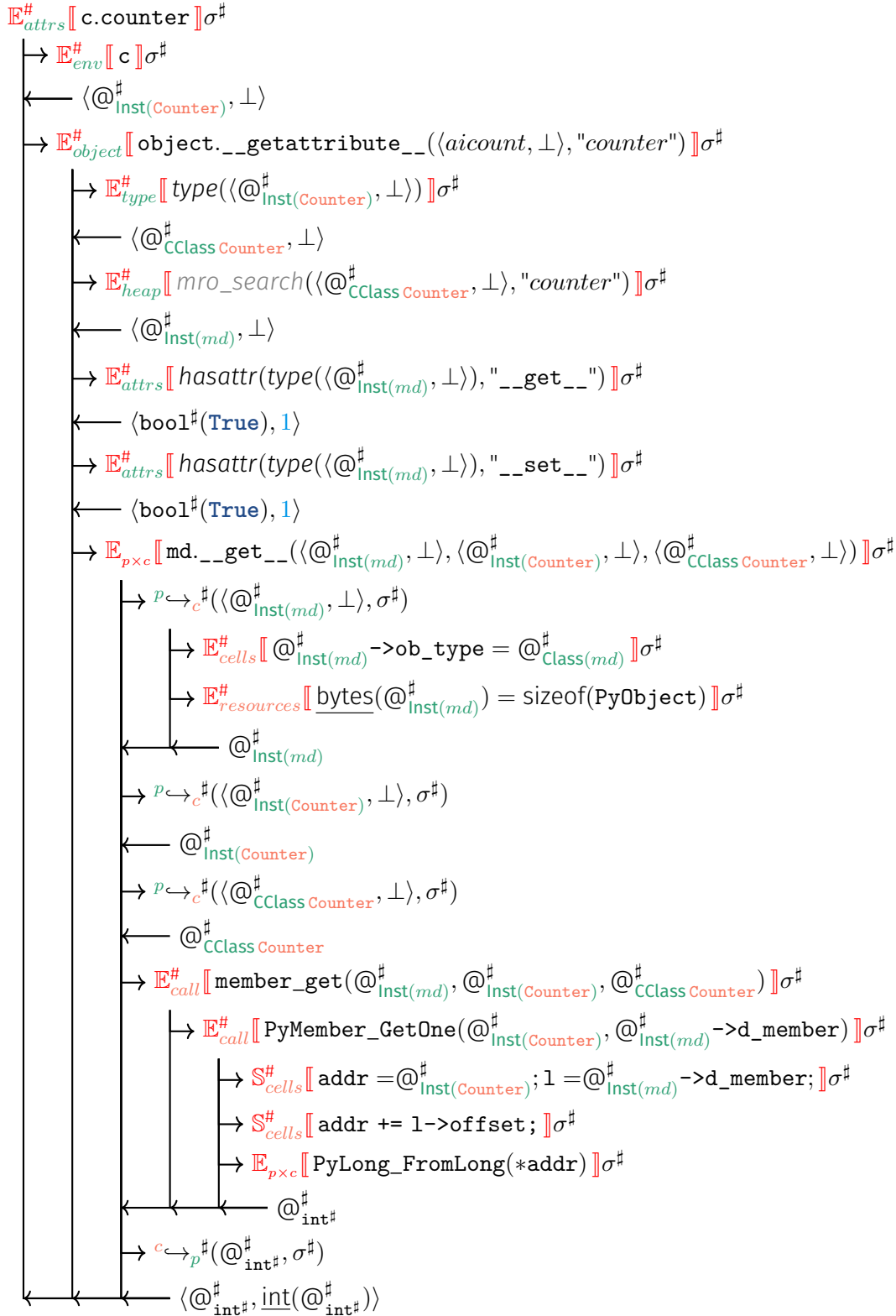
Figure 11.8: Sequence diagram of the analysis of Counter access (Listing 91, line 8)
