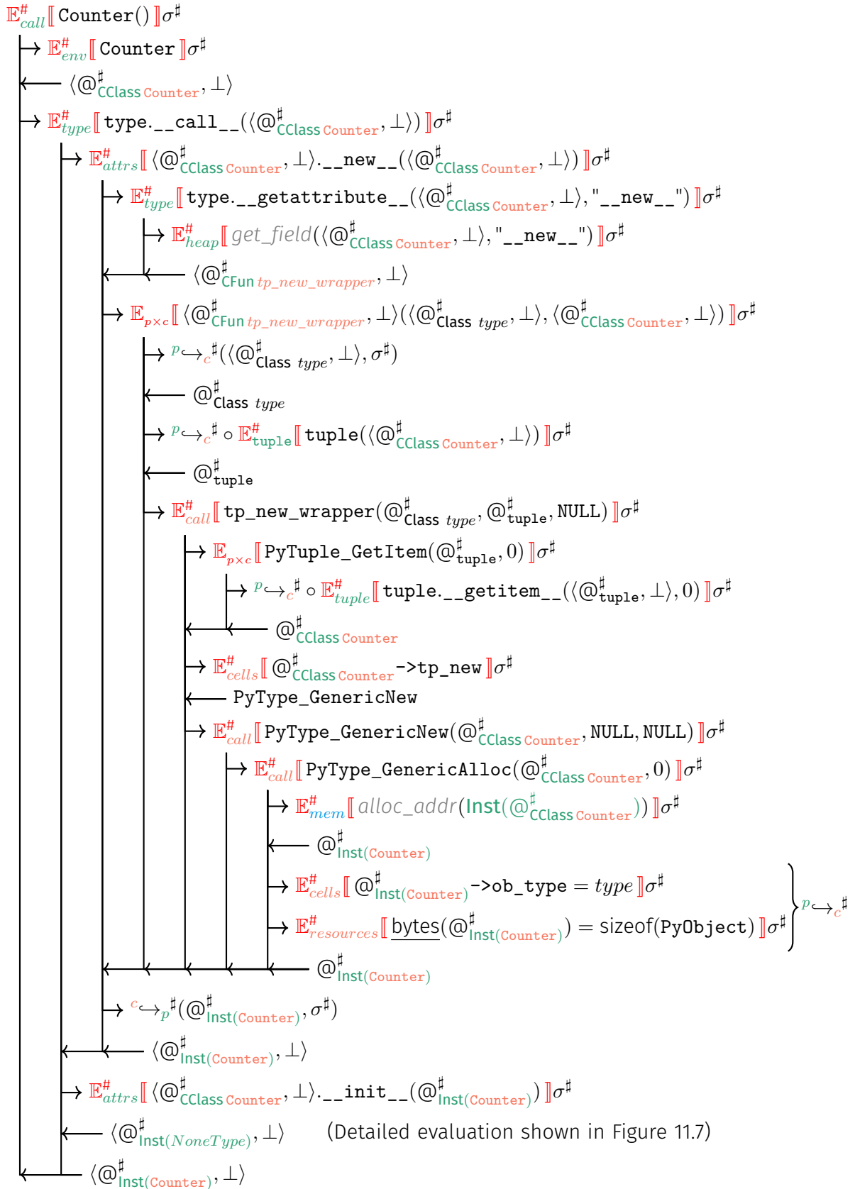
Figure 11.6: Sequence diagram of the analysis of Counter creation (Listing 9.1, line 4) – part 1
