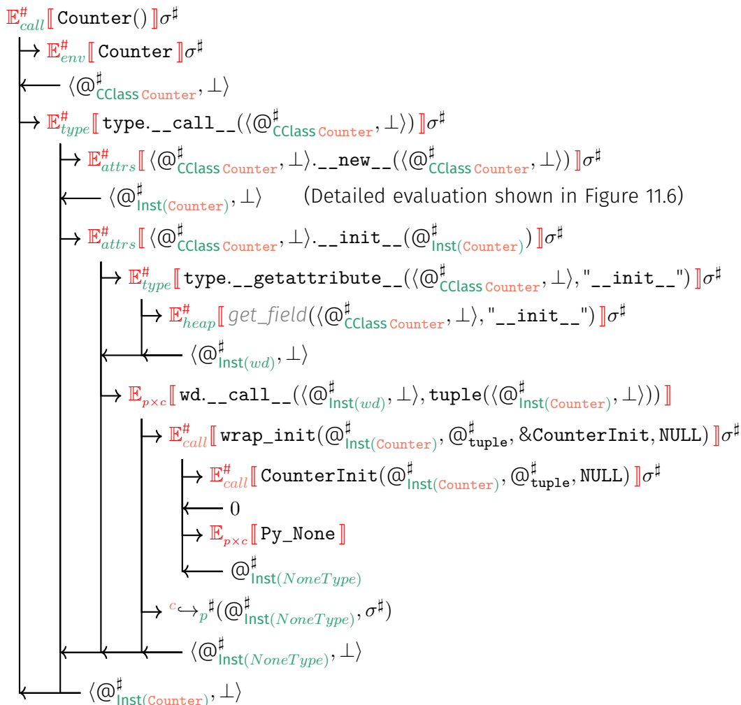
Figure 11.7: Sequence diagram of the analysis of Counter creation (Listing 9.1, line 4) – part 2
