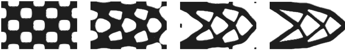
Fig. 2.3: Two-dimensional cantilever computed with the level set method. Initial shape is presented in the left figure. The shape of the cantilever remains clear through all the iterations. Results extracted from the works of Allaire, Jouve and Toader [13].
