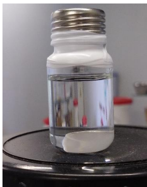
Figure S5.1. Mixture of L - and D -LA (1/1 molar ratio) at 23^\circ\text{C} ( [\text{rac-LA}]_0 = 0.22\text{ M} )
